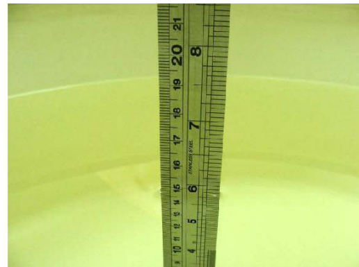
Fig 7.2 Photo of Liquid Height for Body SAR
