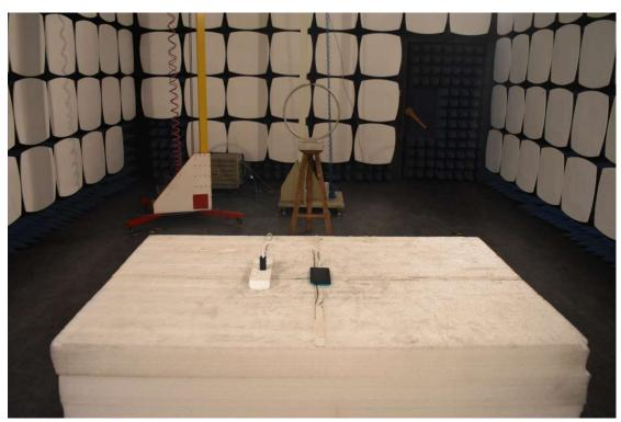
3. Radiated emission (9KHz-30MHz)
