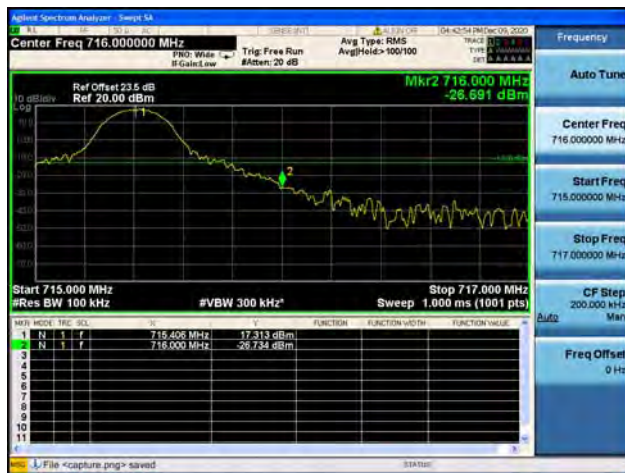
Band12 / 10MHz / High CH / QPSK / 1 RB
