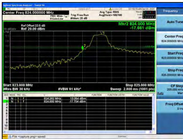
Band5 / 3MHz / Low CH / 16QAM / 1 RB
