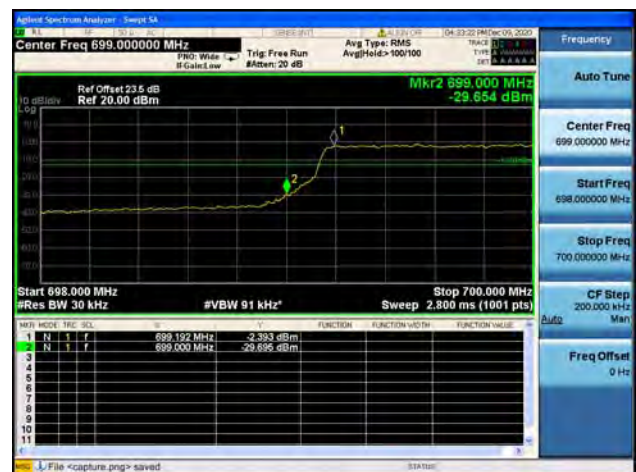
Band12 / 3MHz / Low CH / 16QAM / FULL RB
