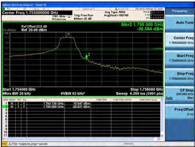
Band4 / 1.4MHz / High CH / QPSK / 1 RB
