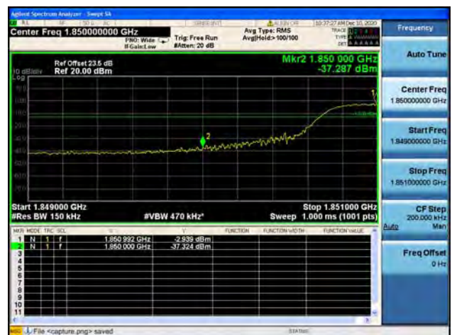
Band2 / 15MHz / Low CH / 16QAM / FULL RB
