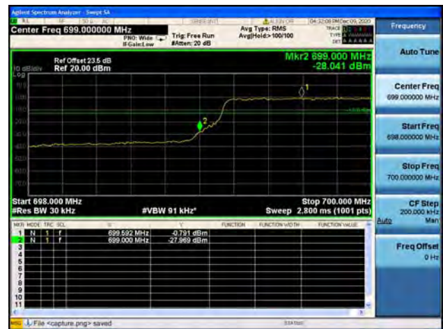
Band12 / 3MHz / Low CH / 16QAM / FULL RB
