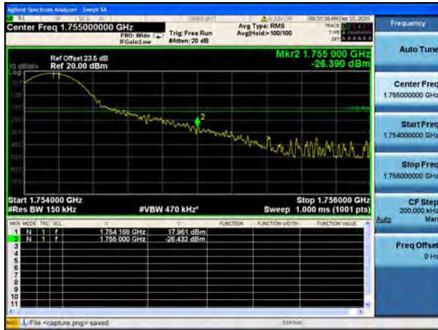
Band4 / 15MHz / High CH / 16QAM / 1 RB
