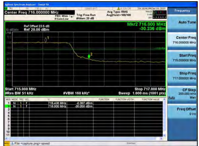
Band12 / 5MHz / High CH / 16QAM / FULL RB
