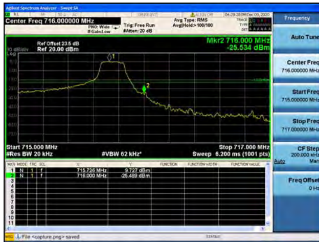
Band12 / 3MHz / Low CH / QPSK / 1 RB
