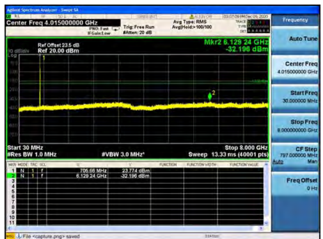
Band12 / 5MHz / Mid CH / 64QAM
