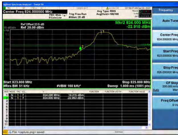
Band5 / 5MHz / High CH / QPSK / 1 RB
