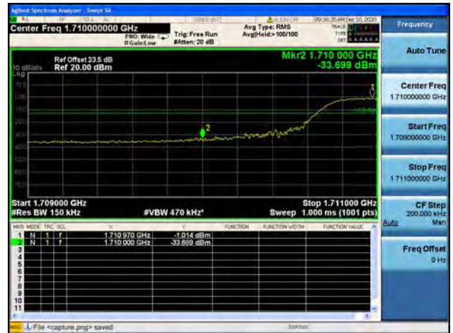
Band4 / 15MHz / Low CH / 16QAM / FULL RB
