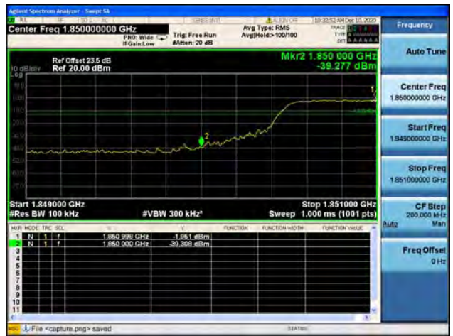
Band2 / 10MHz / Low CH / 16QAM / FULL RB
