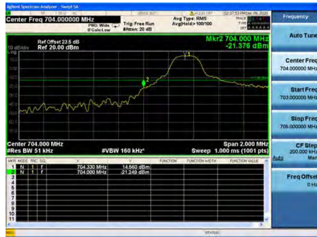
Band17 / 5MHz / Low CH / 16QAM / 1 RB
