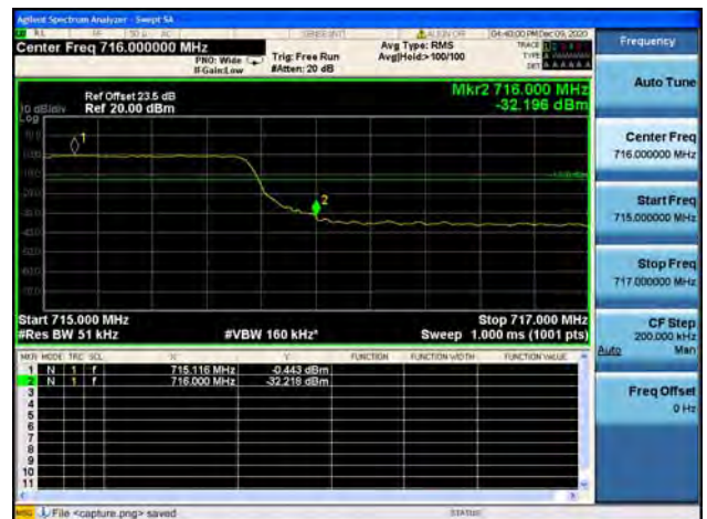
Band12 / 5MHz / High CH / 16QAM / FULL RB
