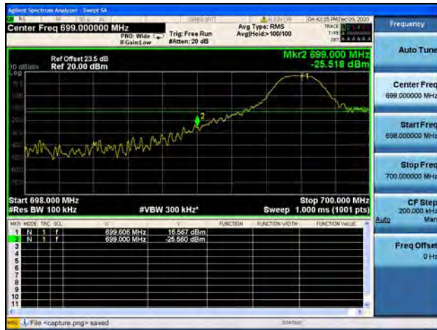
Band12 / 10MHz / High CH / QPSK / 1 RB
