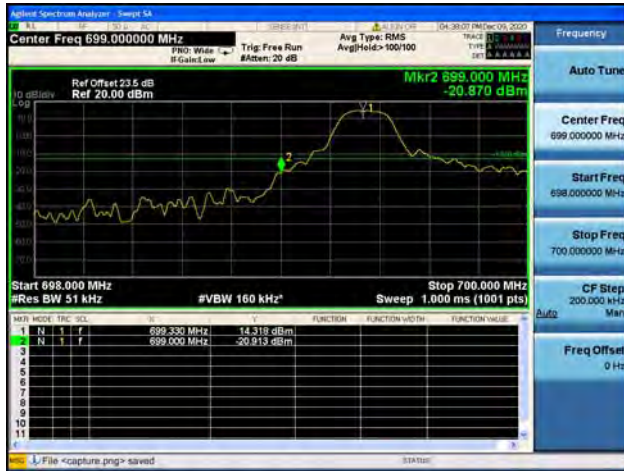
Band12 / 5MHz / High CH / QPSK / 1 RB
