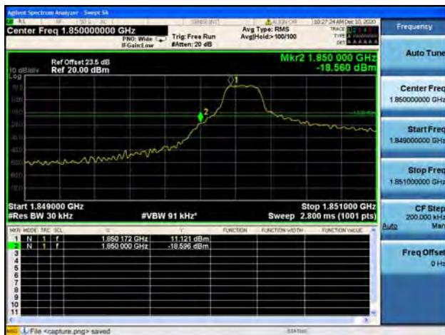
Band2 / 3MHz / Low CH / 16QAM / 1 RB
