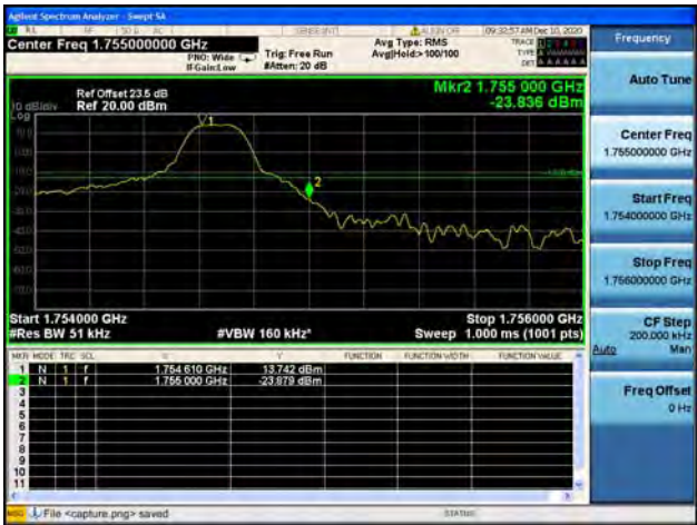
Band4 / 5MHz / High CH / 16QAM / 1 RB
