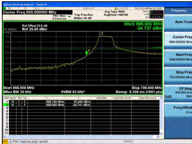
Band12 / 1.4MHz / High CH / QPSK / 1 RB
