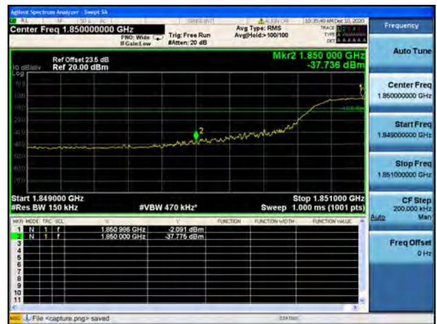
Band2 / 15MHz / Low CH / 16QAM / FULL RB
