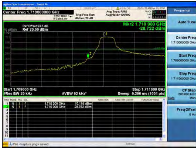
Band4 / 1.4MHz / Low CH / 16QAM / 1 RB
