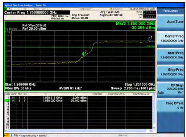
Band2 / 3MHz / Low CH / 16QAM / FULL RB
