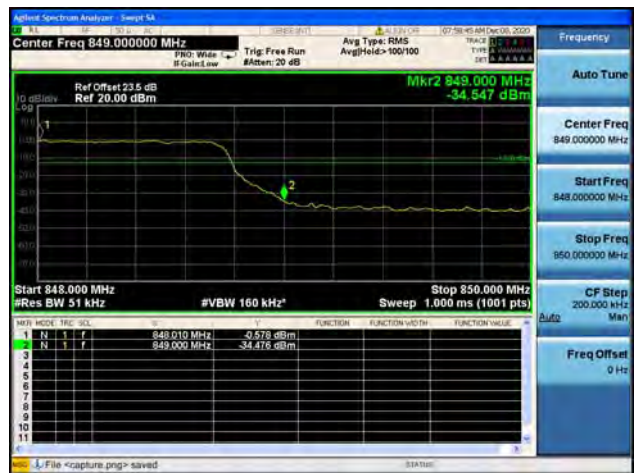
Band5 / 5MHz / High CH / 16QAM / FULL RB
