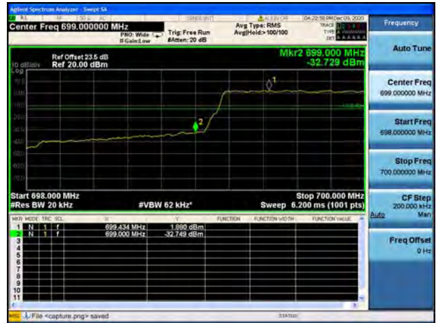
Band12 / 1.4MHz / Low CH / 16QAM / FULL RB
