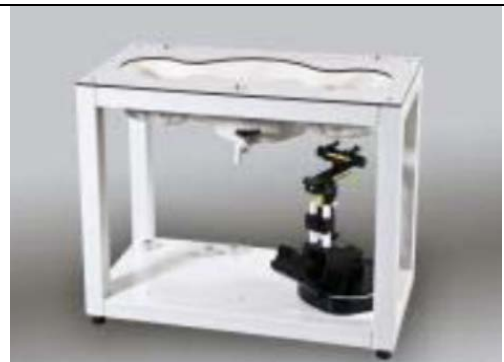
Fig. 6.8 Photo of SAM Phantom
