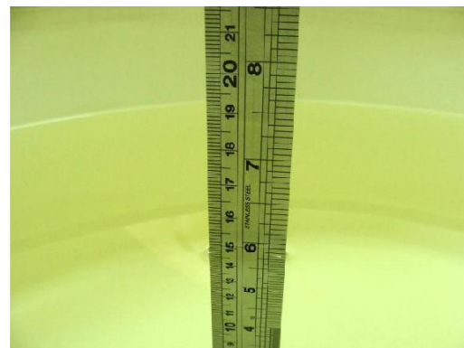
Fig 7.2 Photo of Liquid Height for Body SAR
