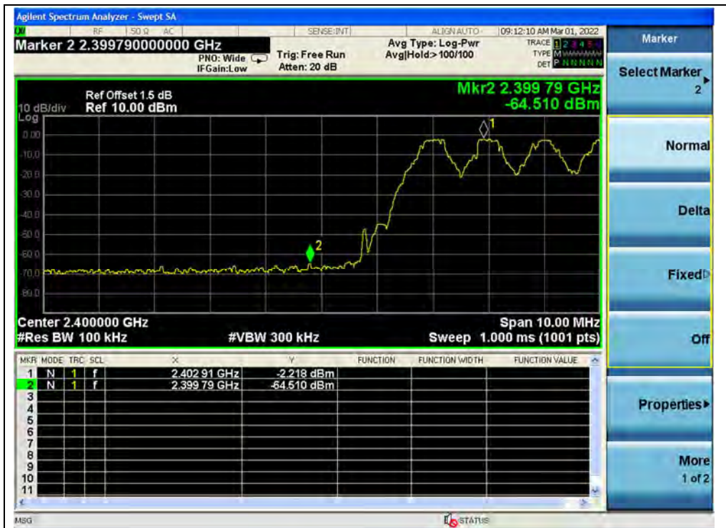
(Band edge with hopping on, Channel 0, GFSK)
