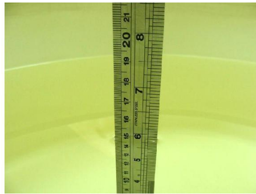
Fig 6.12 Photo of Liquid Height for Body SAR
