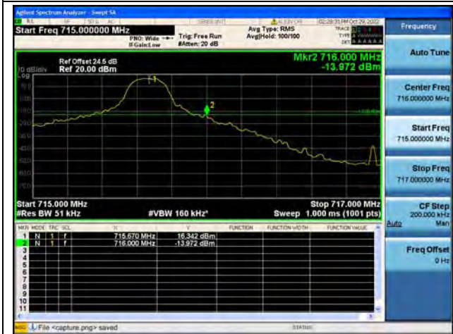
Band12 / 5MHz / High CH / QPSK / 1 RB
