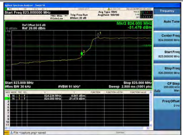
Band5 / 1.4MHz / Low CH / QPSK / FULL RB
