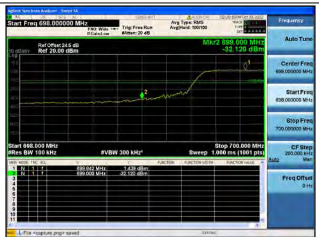
Band12 / 10MHz / Low CH / QPSK / FULL RB
