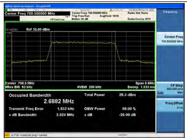
Band12 / 3MHz / 16QAM/ Low CH
