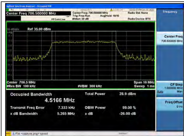
Band17 / 5MHz / QPSK/ Low CH
