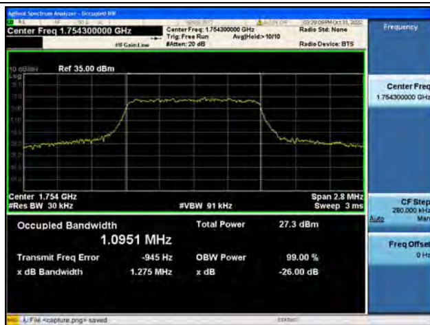
Band4 / 1.4MHz / QPSK/ High CH
