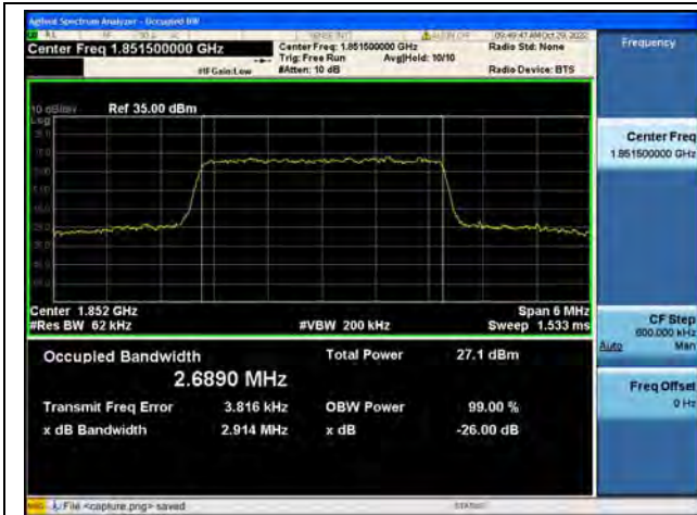
Band2 / 3MHz / QPSK/ Low CH
