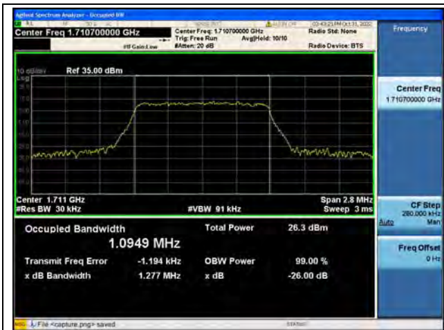
Band66 / 1.4MHz / QPSK/ Low CH
