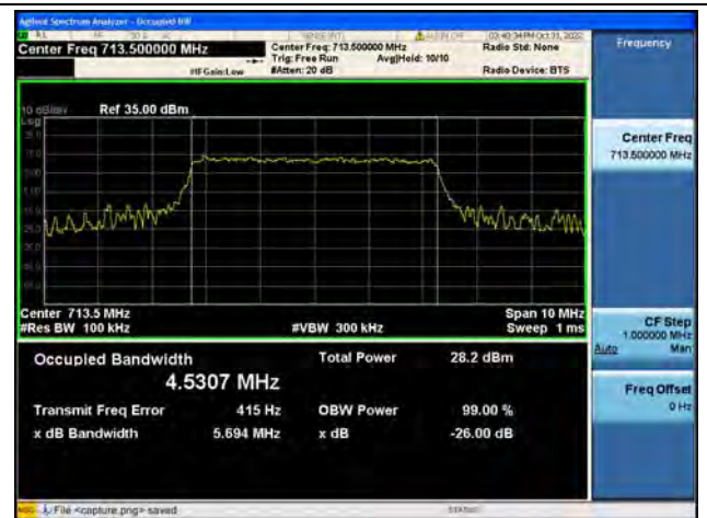
Band12 / 5MHz / 16QAM/ High CH
