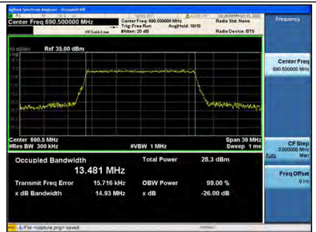
Band71 / 15MHz / 16QAM/ High CH
