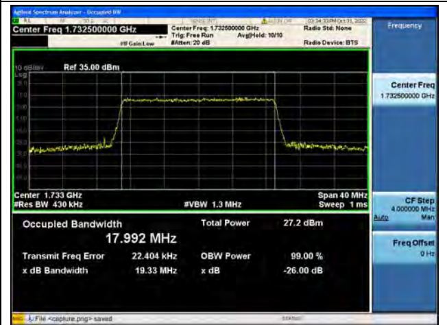
Band4 / 20MHz / 16QAM/ Mid CH
