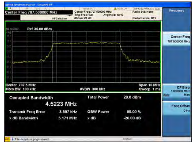
Band12 / 5MHz / 16QAM/ Mid CH
