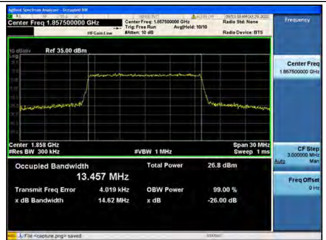
Band2 / 15MHz / 16QAM/ Low CH
