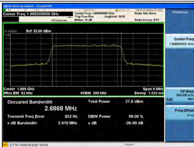
Band2 / 3MHz / QPSK/ High CH
