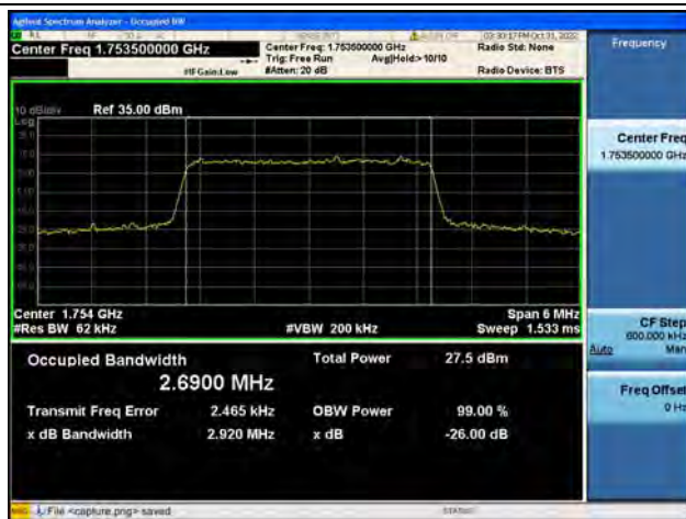
Band4 / 3MHz / QPSK/ High CH
