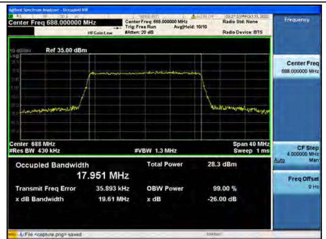
Band71 / 20MHz / 16QAM/ High CH
