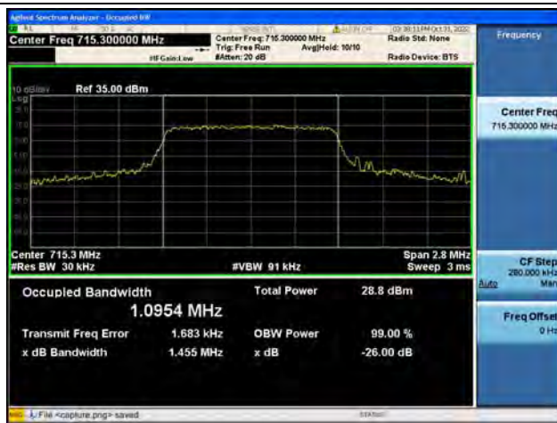
Band12 / 1.4MHz / QPSK/ High CH
