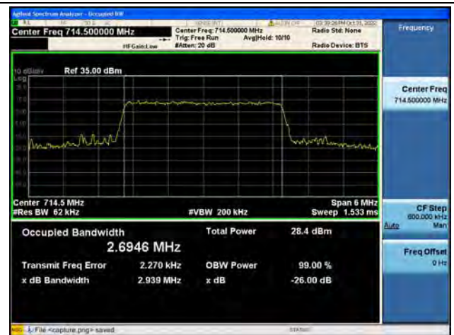
Band12 / 3MHz / 16QAM/ High CH
