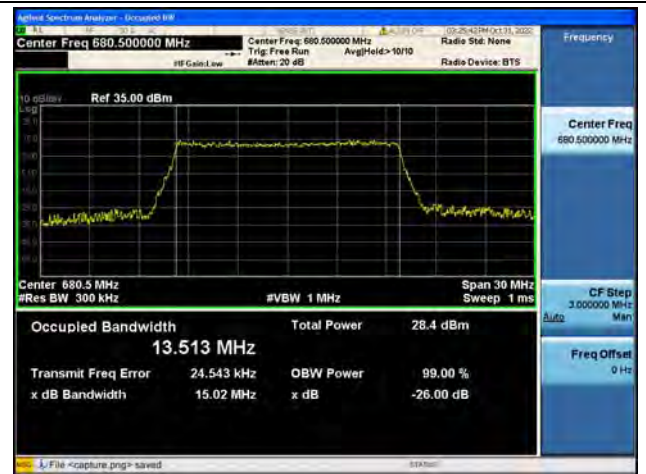
Band71 / 15MHz / 16QAM/ Mid CH
