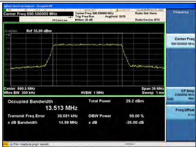
Band71 / 15MHz / QPSK/ High CH
