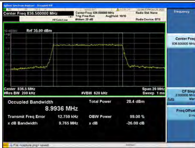
Band5 / 10MHz / QPSK/ Mid CH
