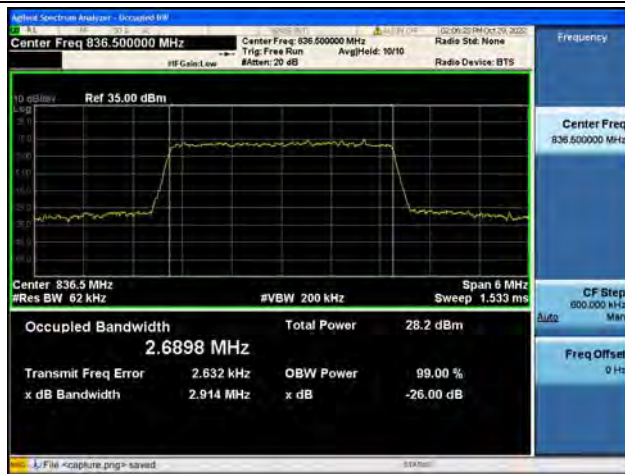
Band5 / 3MHz / QPSK/ Mid CH
