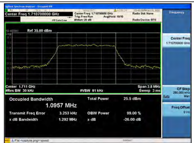
Band66 / 1.4MHz / 16QAM/ Low CH
