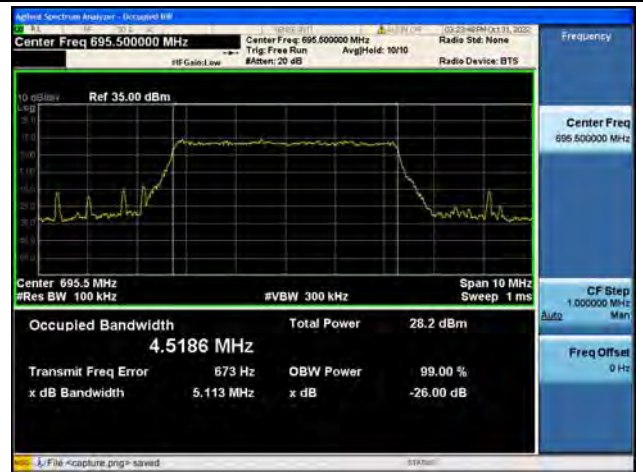
Band71 / 5MHz / 16QAM/ High CH
