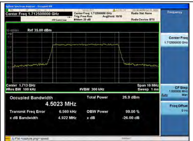
Band4 / 5MHz / 16QAM/ Low CH
