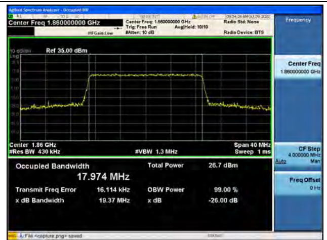
Band2 / 20MHz / 16QAM/ Low CH
