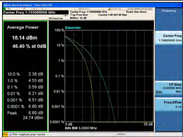
Band66 / 3MHz / Mid CH / QPSK
