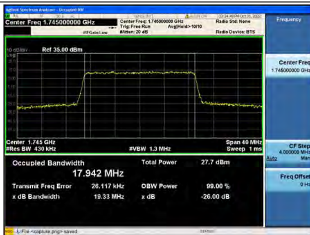
Band4 / 20MHz / QPSK/ High CH
