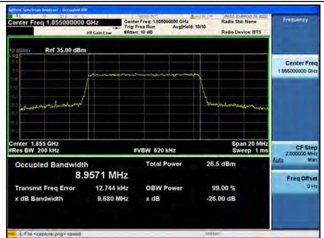
Band2 / 10MHz / 16QAM/ Low CH
