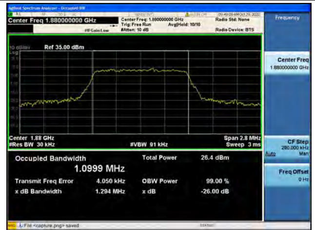
Band2 / 1.4MHz / 16QAM/ Mid CH
