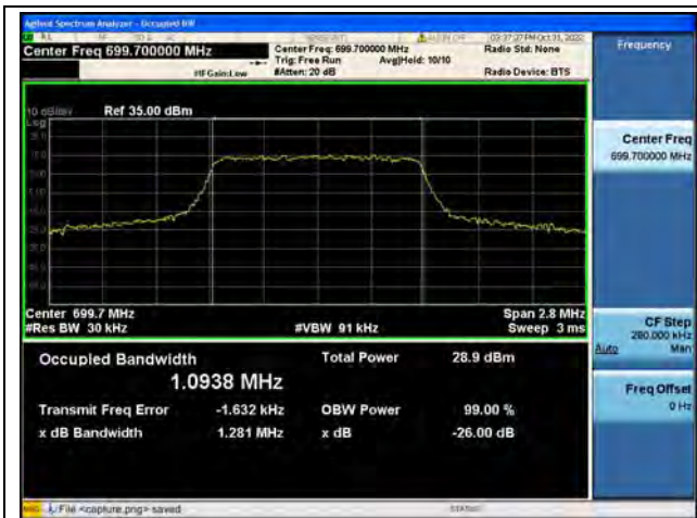
Band12 / 1.4MHz / QPSK/ Low CH
