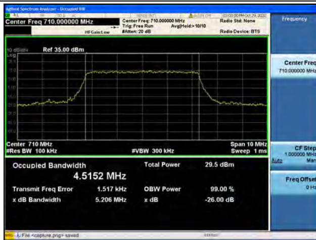
Band17 / 5MHz / QPSK/ Mid CH
