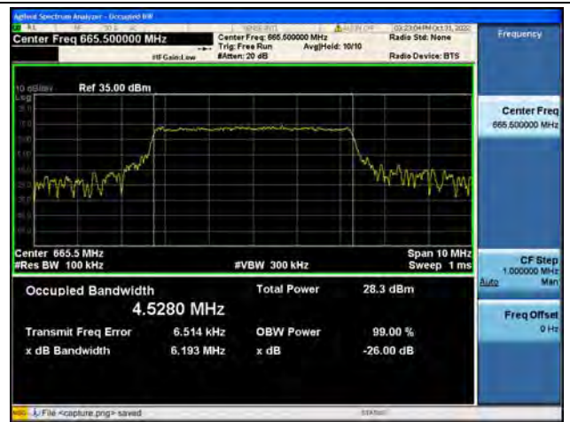
Band71 / 5MHz / 16QAM/ Low CH
