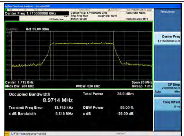
Band66 / 10MHz / 16QAM/ Low CH
