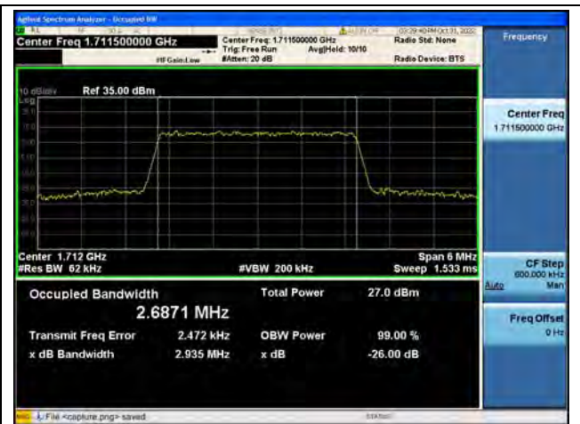
Band4 / 3MHz / 16QAM/ Low CH
