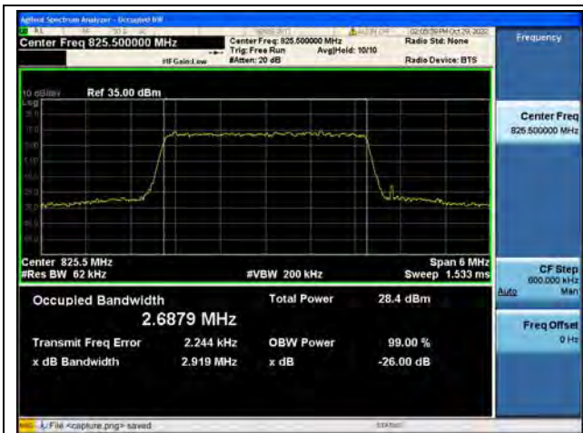
Band5 / 3MHz / QPSK/ Low CH
