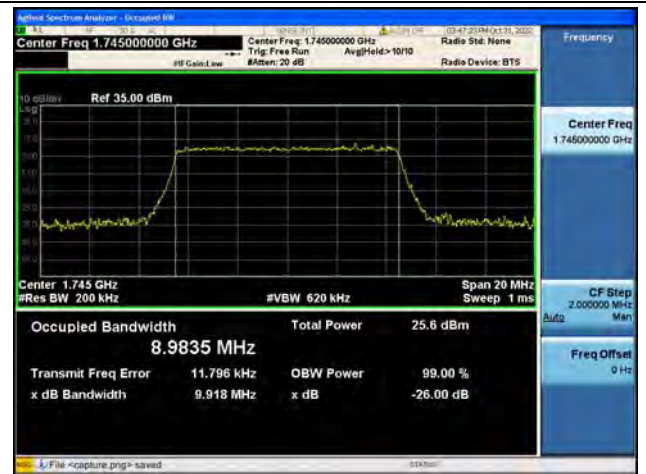
Band66 / 10MHz / 16QAM/ Mid CH
