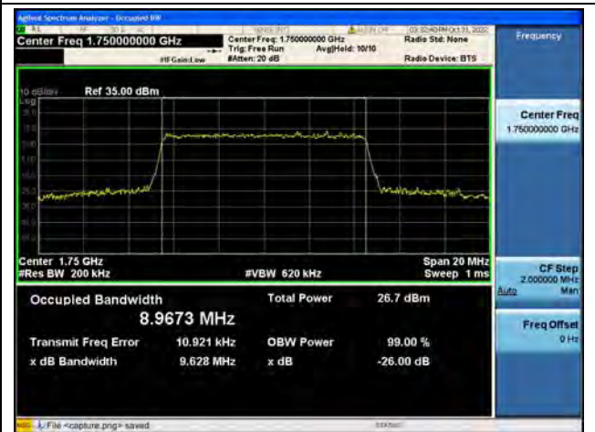
Band4 / 10MHz / 16QAM/ High CH
