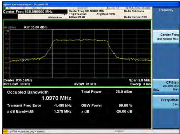
Band5 / 1.4MHz / QPSK/ Mid CH
