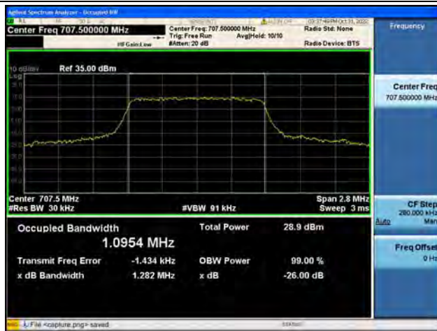
Band12 / 1.4MHz / QPSK/ Mid CH
