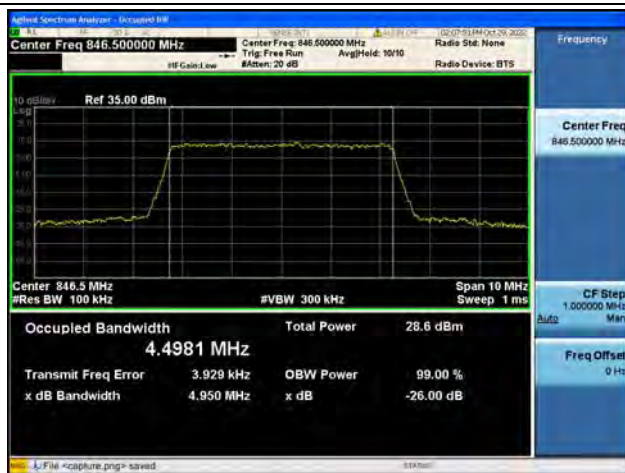
Band5 / 5MHz / QPSK/ High CH
