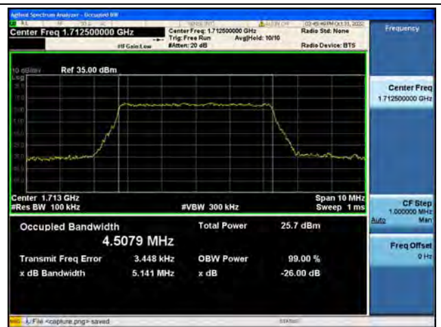
Band66 / 5MHz / 16QAM/ Low CH
