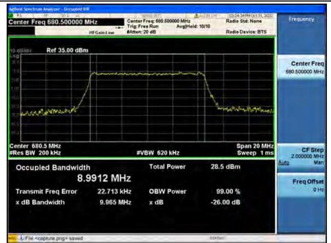
Band71 / 10MHz / 16QAM/ Mid CH
