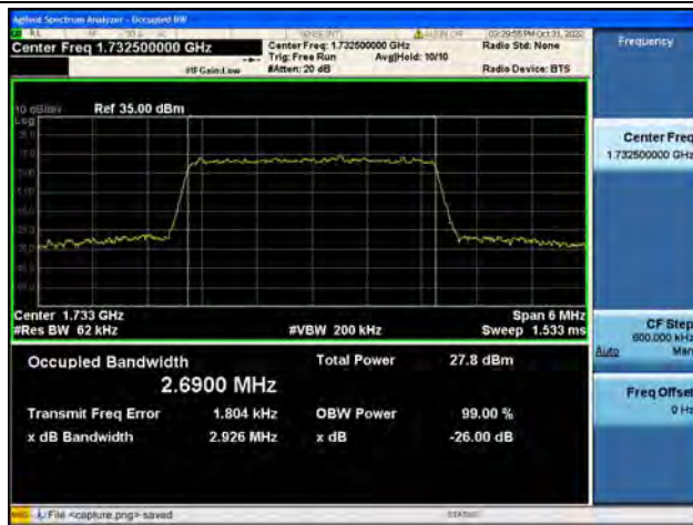
Band4 / 3MHz / QPSK/ Mid CH
