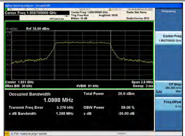
Band2 / 1.4MHz / 16QAM/ Low CH
