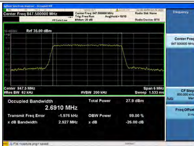
Band5 / 3MHz / QPSK/ High CH
