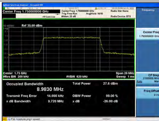
Band4 / 10MHz / QPSK/ High CH
