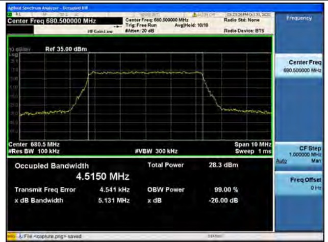
Band71 / 5MHz / 16QAM/ Mid CH
