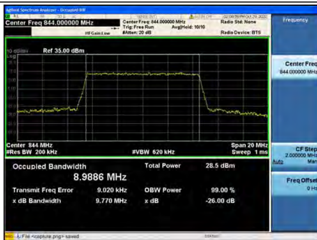
Band5 / 10MHz / QPSK/ High CH
