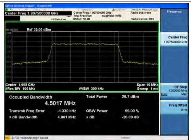
Band2 / 5MHz / 16QAM/ High CH
