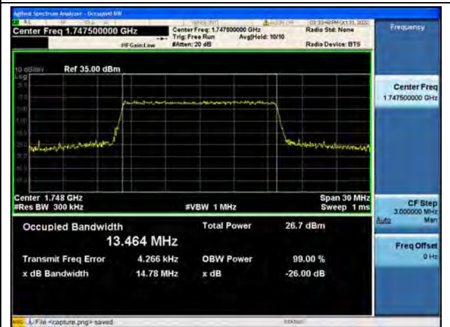
Band4 / 15MHz / 16QAM/ High CH
