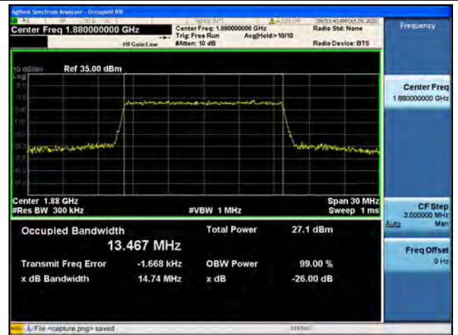
Band2 / 15MHz / 16QAM/ Mid CH
