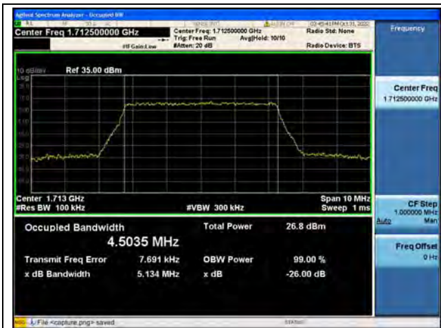
Band66 / 5MHz / QPSK/ Low CH
