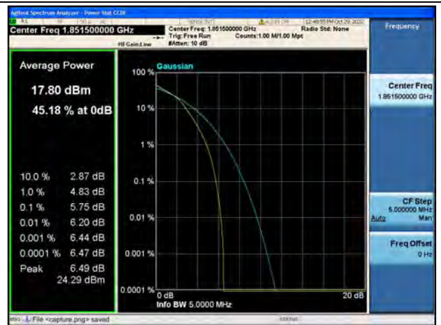
Band2 / 3MHz / Low CH / 16QAM
