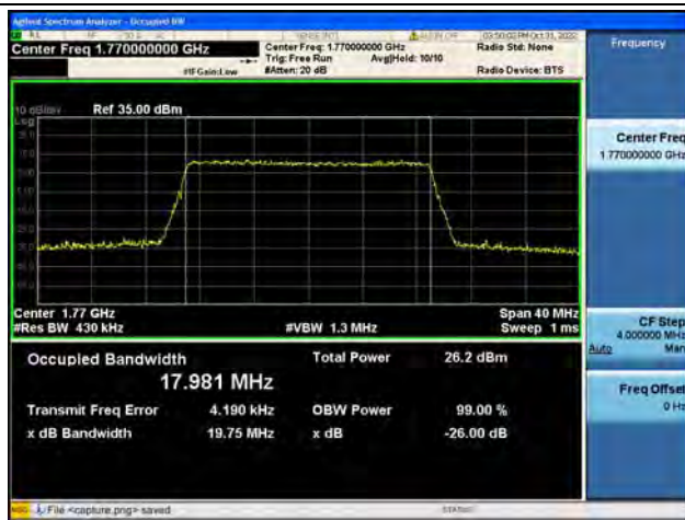
Band66 / 20MHz / QPSK/ High CH
