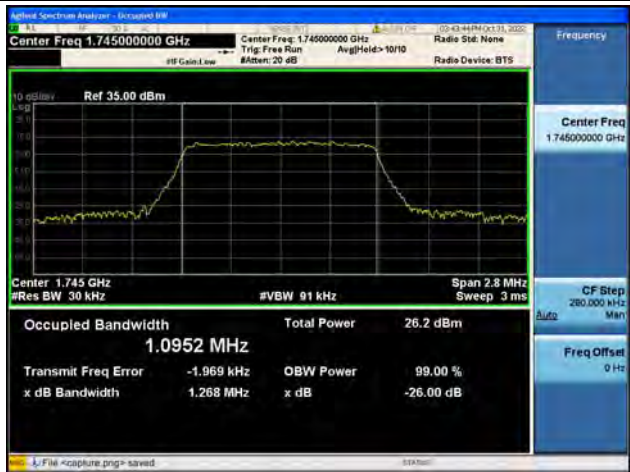
Band66 / 1.4MHz / QPSK/ Mid CH
