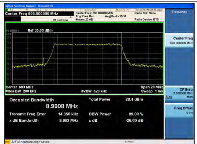
Band71 / 10MHz / 16QAM/ High CH
