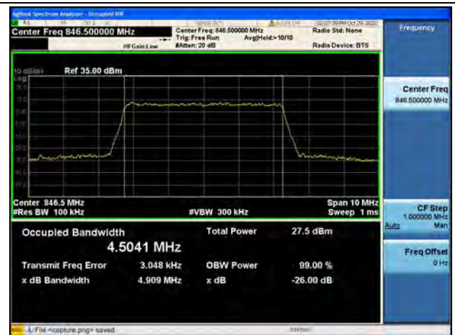
Band5 / 5MHz / 16QAM/ High CH
