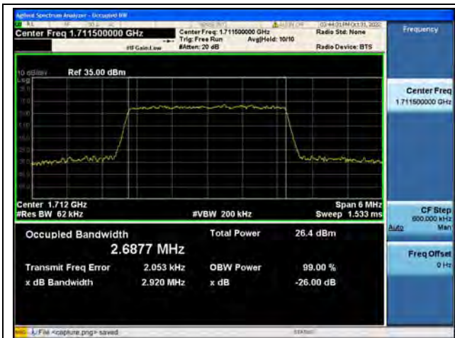
Band66 / 3MHz / QPSK/ Low CH
