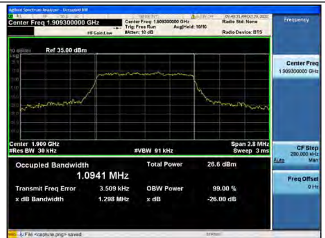
Band2 / 1.4MHz / 16QAM/ High CH
