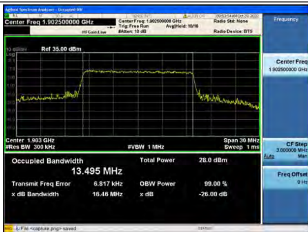
Band2 / 15MHz / QPSK/ High CH
