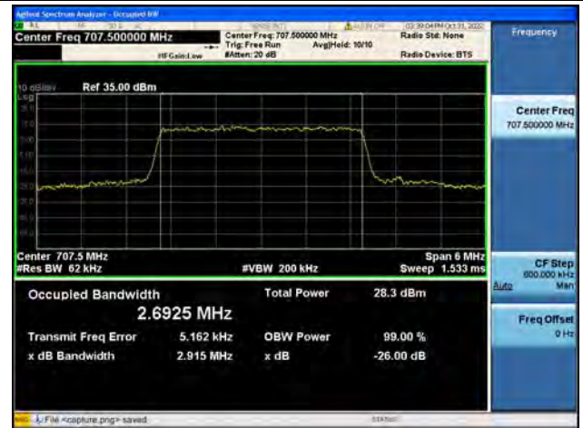
Band12 / 3MHz / 16QAM/ Mid CH
