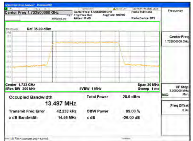
Band4 / 15MHz / QPSK/ Mid CH
