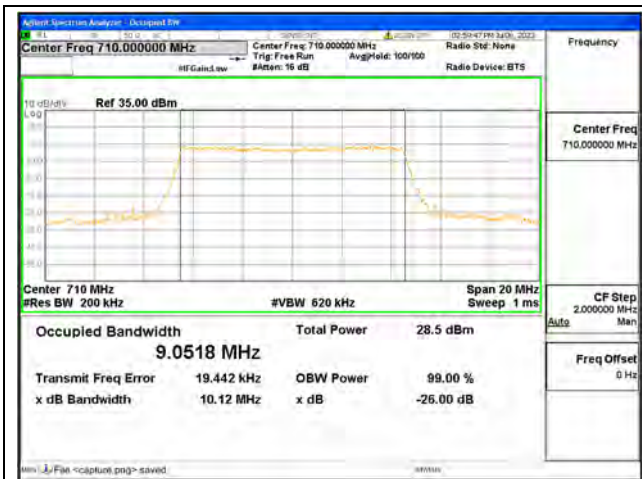
Band17 / 10MHz / QPSK/ Mid CH
