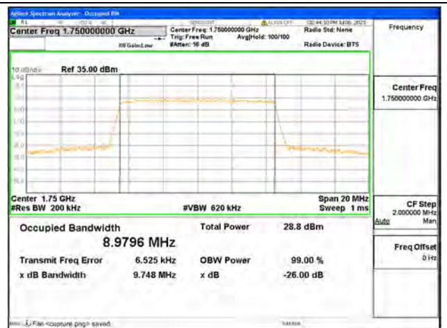
Band4 / 10MHz / 64QAM/ High CH
