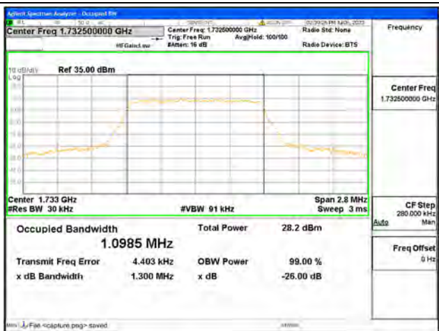
Band4 / 1.4MHz / 16QAM/ Mid CH
