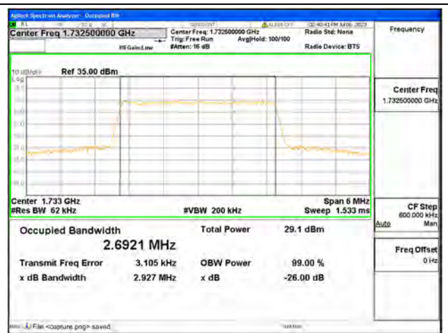
Band4 / 3MHz / 16QAM/ Mid CH
