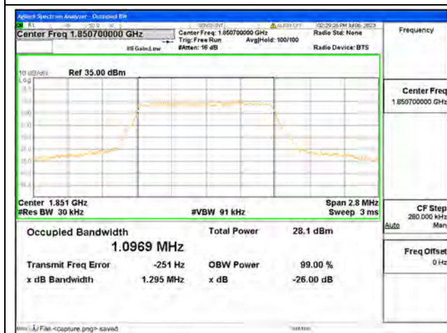
Band2 / 1.4MHz / 64QAM/ Low CH
