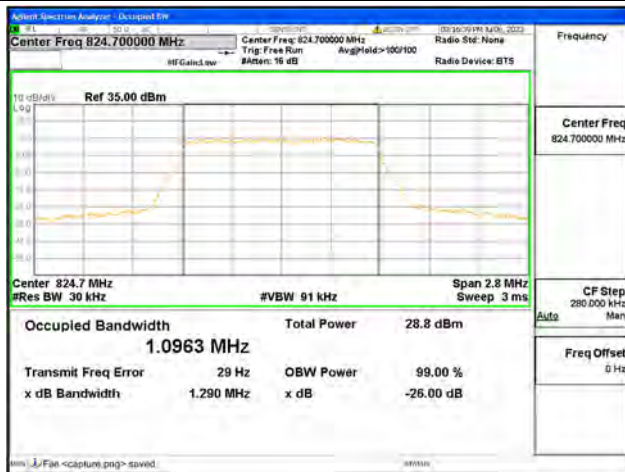
Band26 Part22 / 1.4MHz / 64QAM/ Low CH
