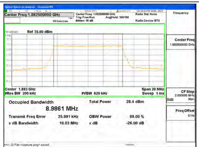
Band25 / 10MHz / 16QAM/ Mid CH
