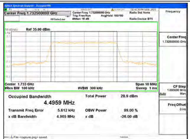
Band4 / 5MHz / 64QAM/ Mid CH
