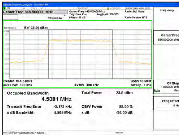
Band26 Part22 / 5MHz / 64QAM/ High CH
