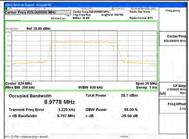
Band5 / 10MHz / 64QAM/ Low CH
