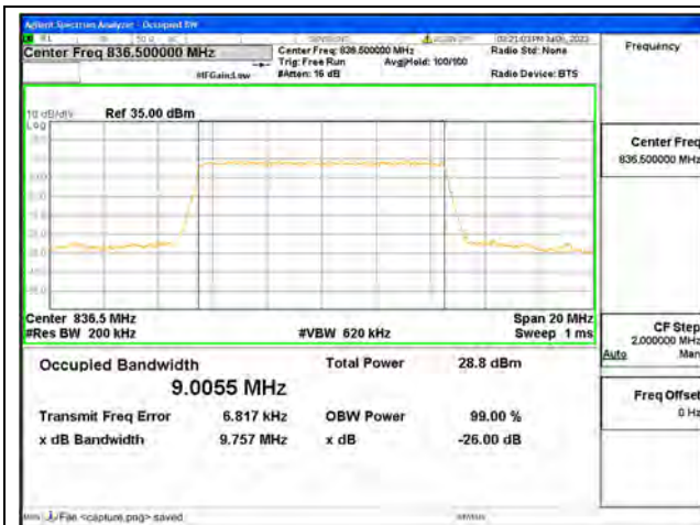
Band26 Part22 / 10MHz / QPSK/ Mid CH
