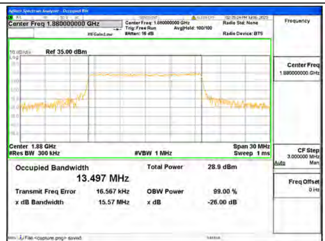
Band2 / 15MHz / 64QAM/ Mid CH
