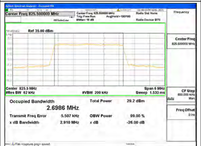
Band5 / 3MHz / 64QAM/ Low CH
