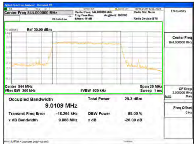
Band5 / 10MHz / QPSK/ High CH
