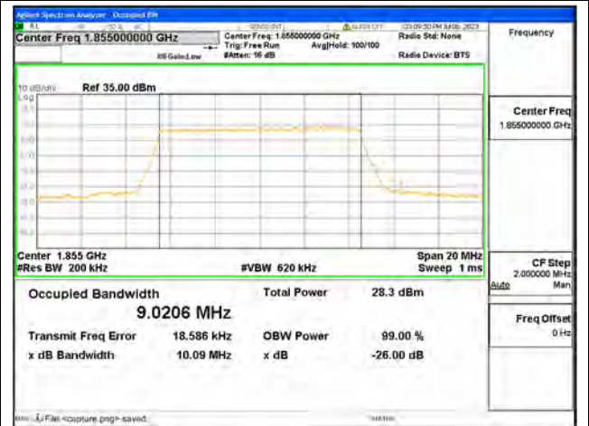
Band25 / 10MHz / QPSK/ Low CH
