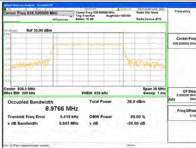
Band26 Part22 / 10MHz / 64QAM/ Mid CH
