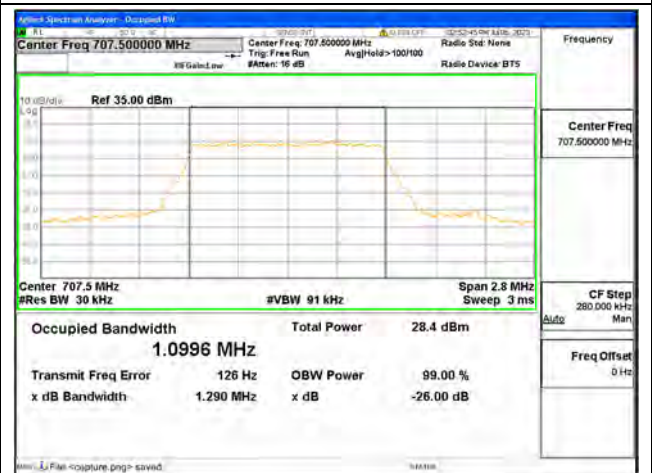
Band12 / 1.4MHz / 64QAM/ Mid CH
