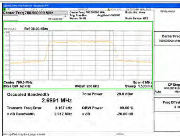
Band12 / 3MHz / 16QAM/ Low CH
