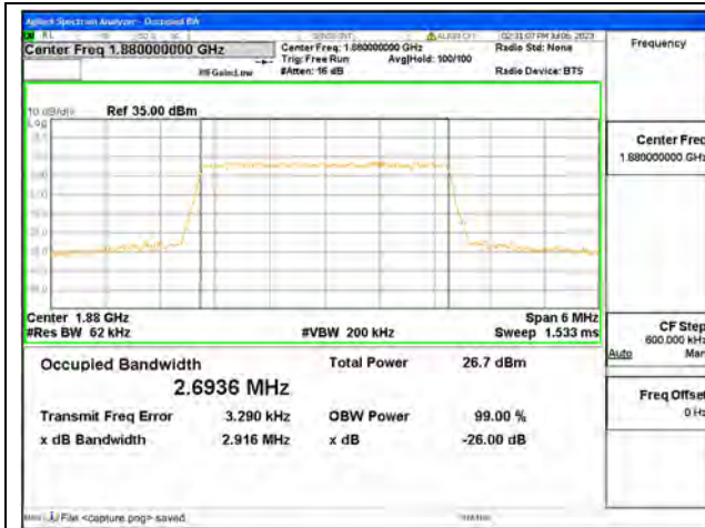
Band2 / 3MHz / QPSK/ Mid CH
