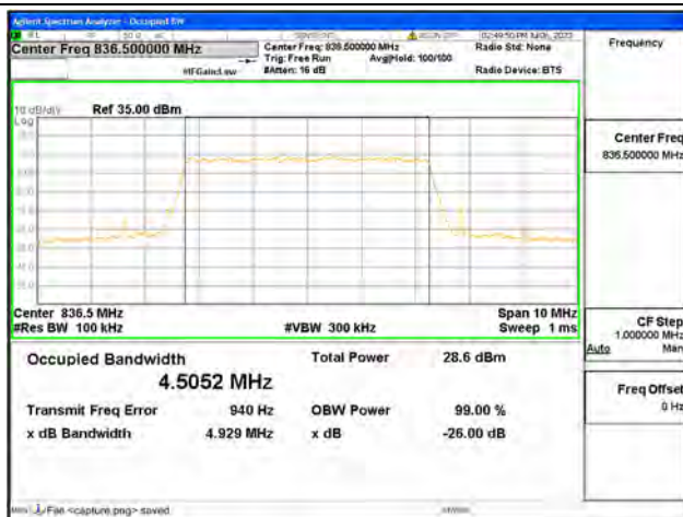
Band5 / 5MHz / 16QAM/ Mid CH
