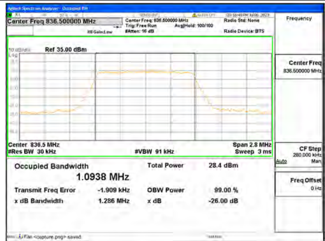
Band26 Part22 / 1.4MHz / QPSK/ Mid CH
