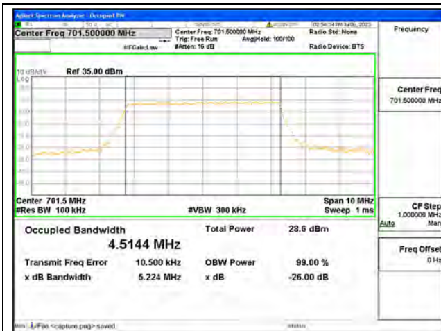
Band12 / 5MHz / QPSK/ Low CH
