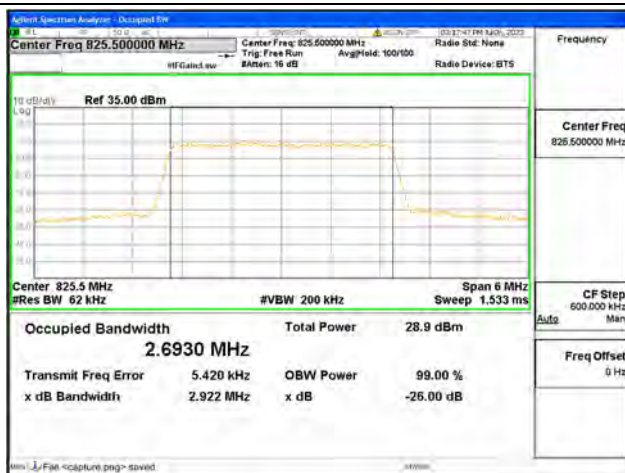
Band26 Part22 / 3MHz / 16QAM/ Low CH
