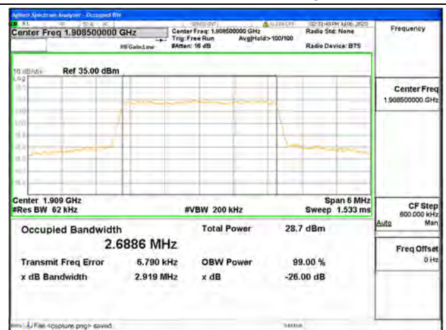
Band2 / 3MHz / 64QAM/ High CH
