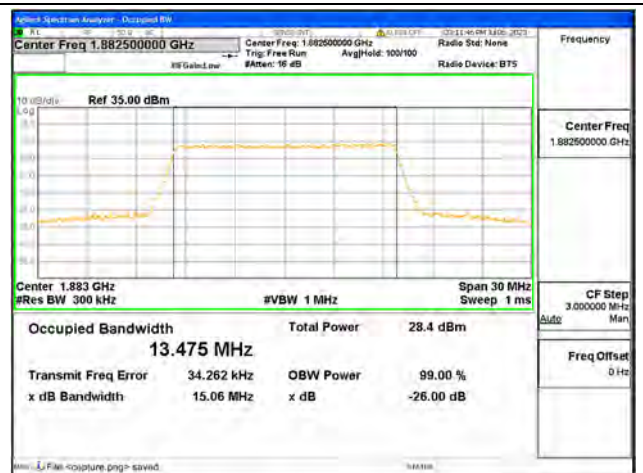
Band25 / 15MHz / 64QAM/ Mid CH
