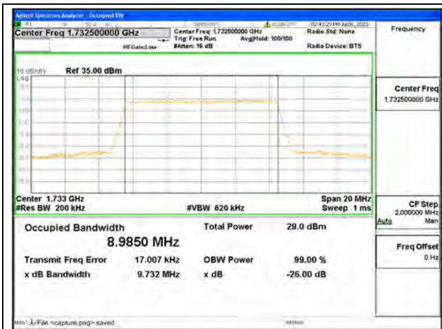
Band4 / 10MHz / QPSK/ Mid CH
