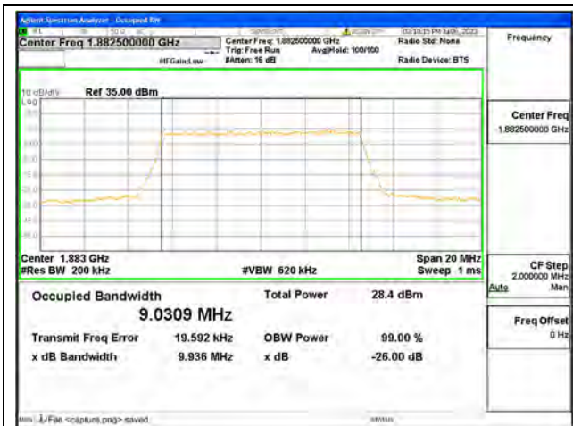
Band25 / 10MHz / QPSK/ Mid CH
