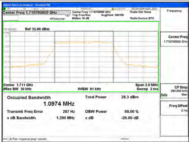
Band4 / 1.4MHz / 64QAM/ Low CH
