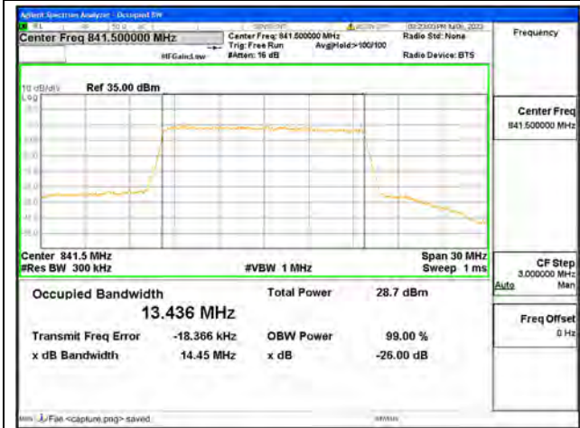
Band26 Part22 / 15MHz / 64QAM/ High CH
