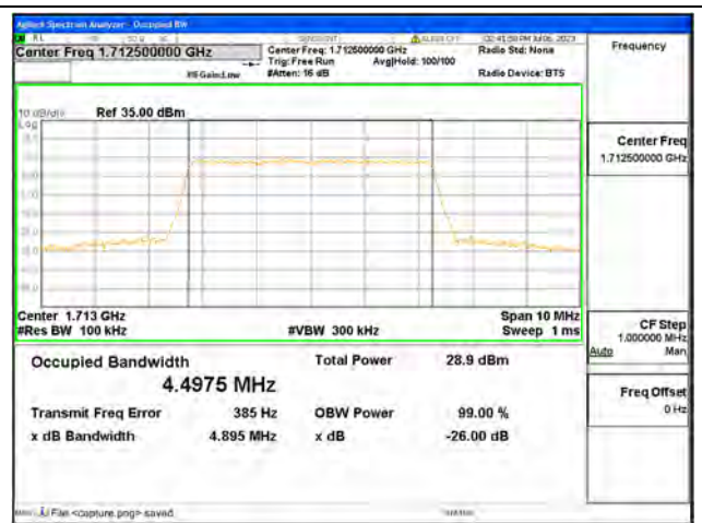
Band4 / 5MHz / 16QAM/ Low CH
