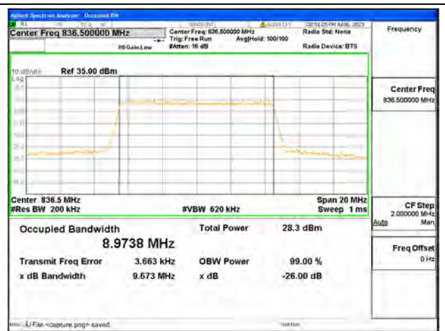
Band5 / 10MHz / 16QAM/ Mid CH
