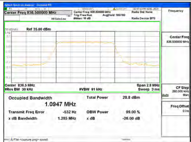
Band5 / 1.4MHz / QPSK/ Mid CH
