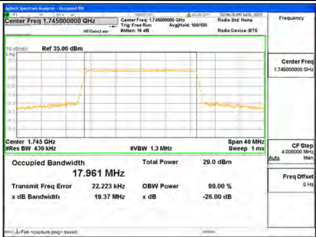
Band4 / 20MHz / 16QAM/ High CH
