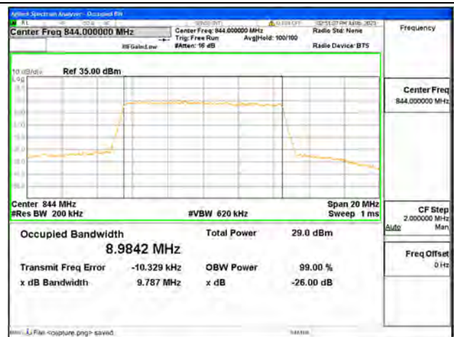
Band5 / 10MHz / 64QAM/ High CH
