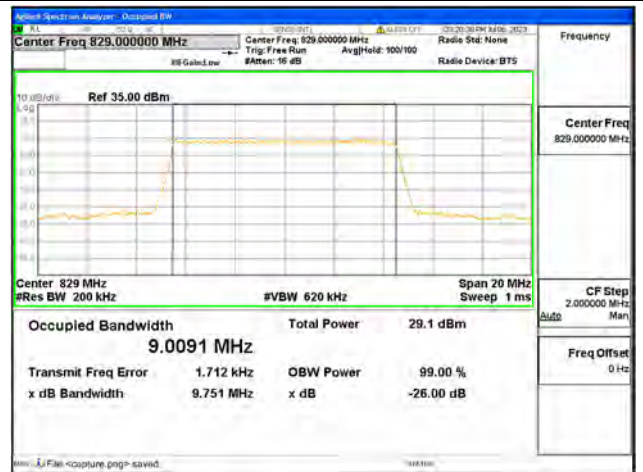
Band26 Part22 / 10MHz / QPSK/ Low CH
