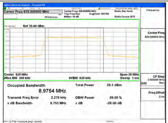
Band26 Part22 / 10MHz / 64QAM/ Low CH
