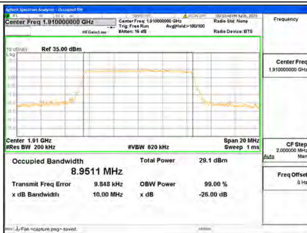
Band25 / 10MHz / 16QAM/ High CH
