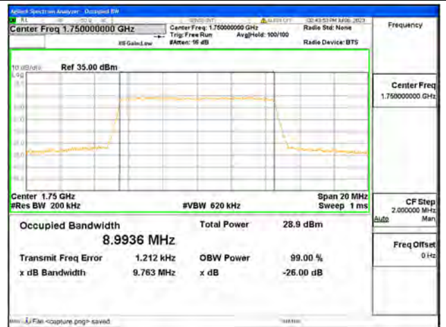
Band4 / 10MHz / QPSK/ High CH
