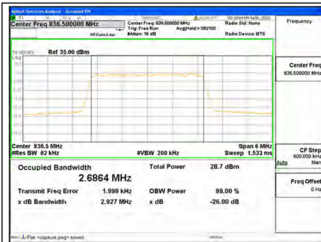
Band26 Part22 / 3MHz / QPSK/ Mid CH
