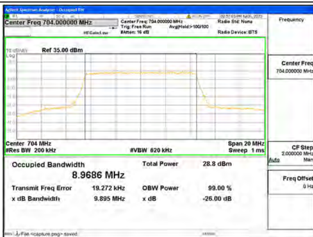
Band12 / 10MHz / 16QAM/ Low CH
