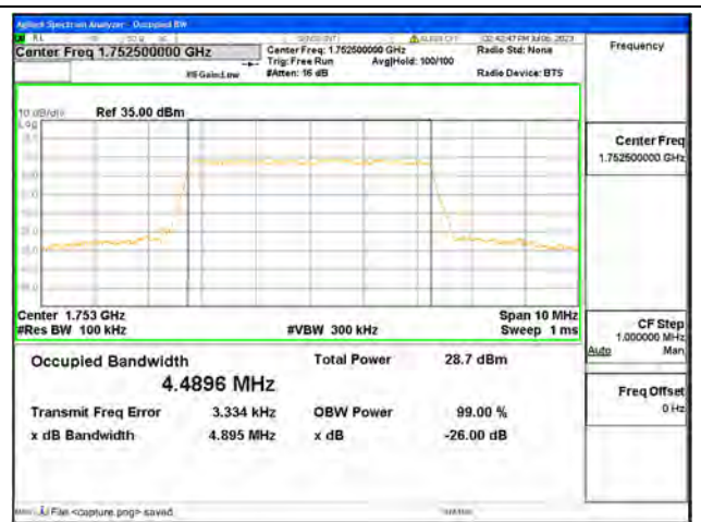
Band4 / 5MHz / 16QAM / High CH
