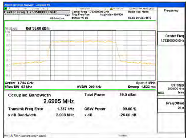
Band4 / 3MHz / QPSK/ High CH
