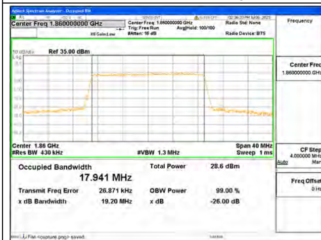
Band2 / 20MHz / 16QAM/ Low CH
