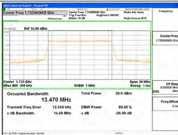
Band4 / 15MHz / 16QAM/ Mid CH
