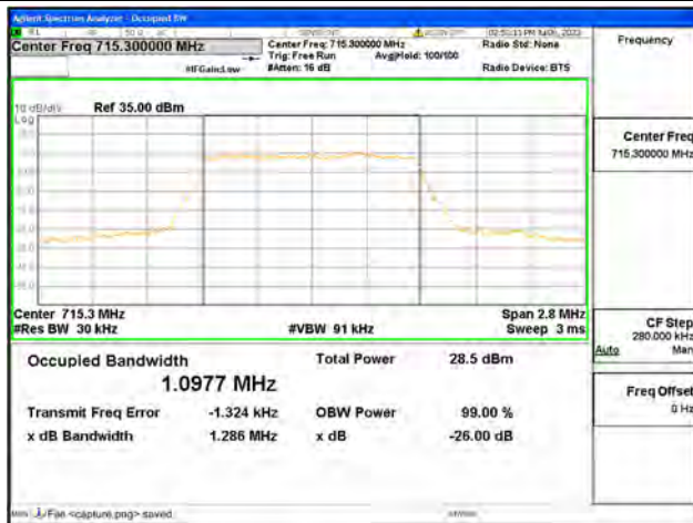
Band12 / 1.4MHz / 64QAM/ High CH
