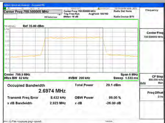
Band12 / 3MHz / 64QAM/ Low CH
