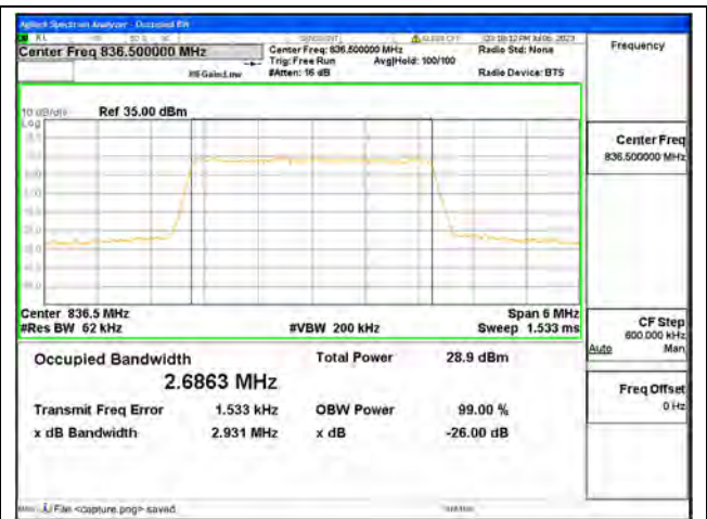
Band26 Part22 / 3MHz / 16QAM/ Mid CH
