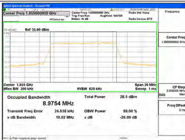
Band25 / 10MHz / 16QAM/ Low CH
