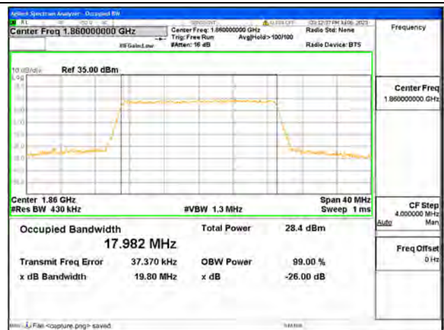
Band25 / 20MHz / 64QAM/ Low CH
