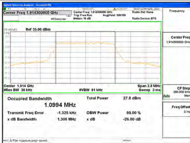
Band25 / 1.4MHz / 64QAM/ High CH
