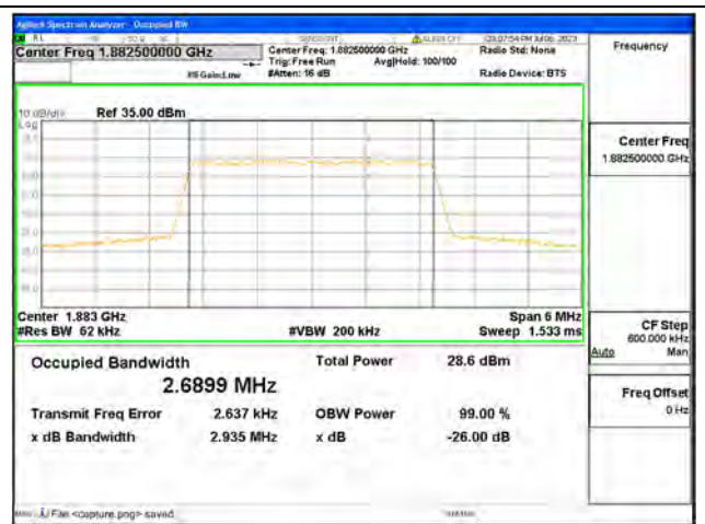
Band25 / 3MHz / 16QAM/ Mid CH
