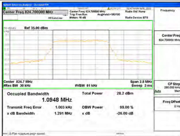
Band5 / 1.4MHz / 64QAM/ Low CH
