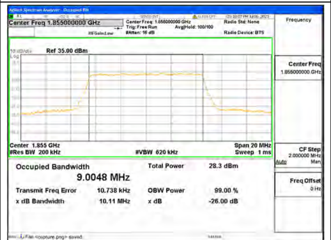
Band25 / 10MHz / 64QAM/ Low CH
