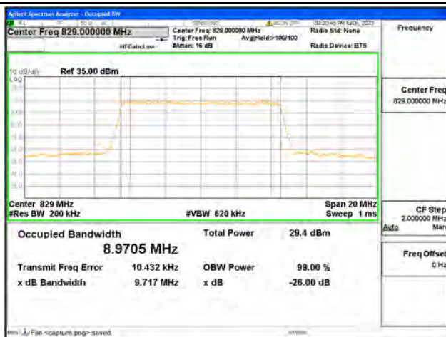
Band26 Part22 / 10MHz / 16QAM/ Low CH
