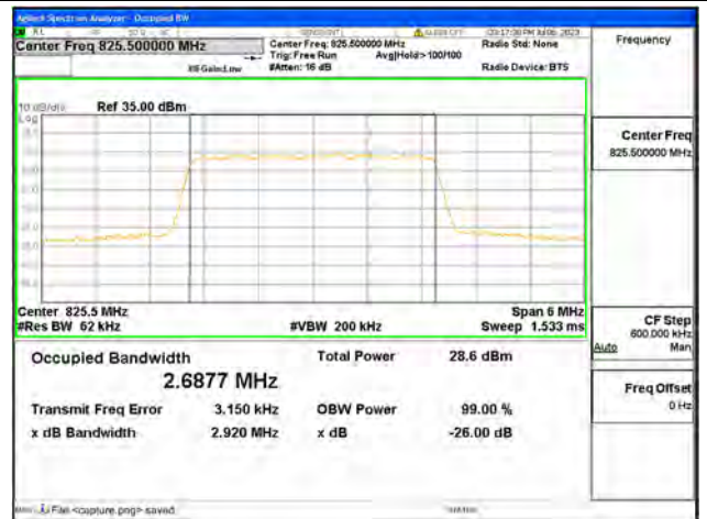
Band26 Part22 / 3MHz / QPSK/ Low CH
