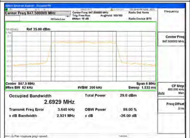
Band26 Part22 / 3MHz / 64QAM/ High CH
