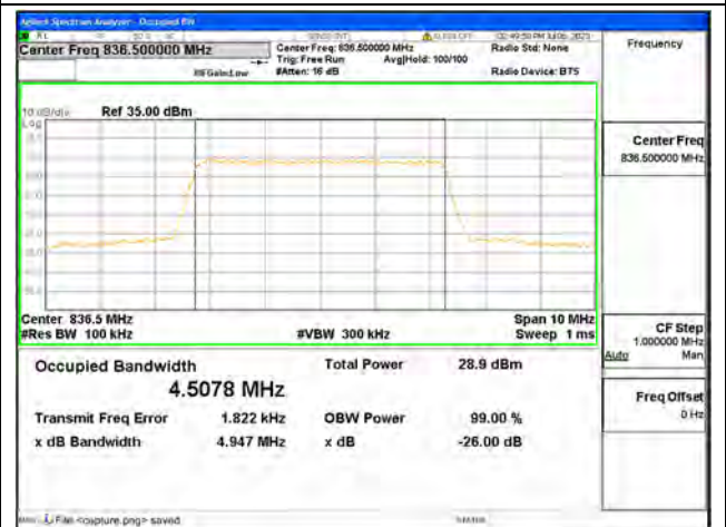
Band5 / 5MHz / 64QAM/ Mid CH
