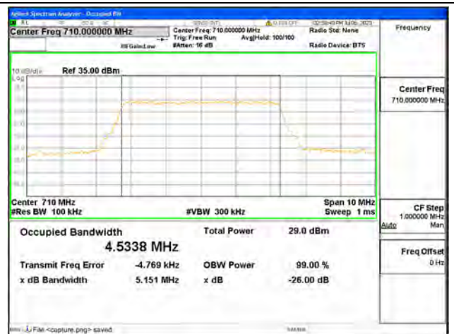
Band17 / 5MHz / 64QAM/ Mid CH
