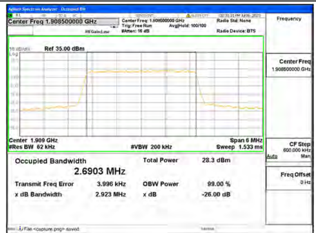
Band2 / 3MHz / QPSK/ High CH
