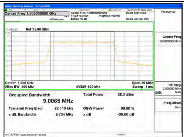
Band2 / 10MHz / QPSK/ High CH
