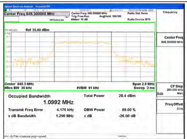
Band26 Part22 / 1.4MHz / 16QAM/ High CH
