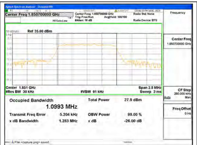
Band25 / 1.4MHz / 16QAM/ Low CH
