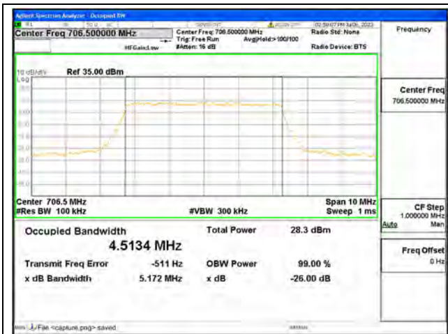
Band17 / 5MHz / QPSK/ Low CH
