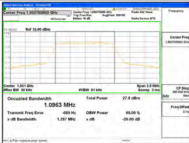
Band25 / 1.4MHz / 64QAM/ Low CH
