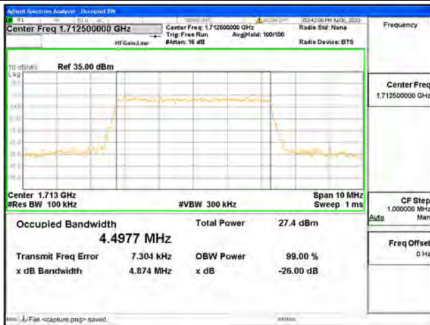
Band4 / 5MHz / 64QAM/ Low CH
