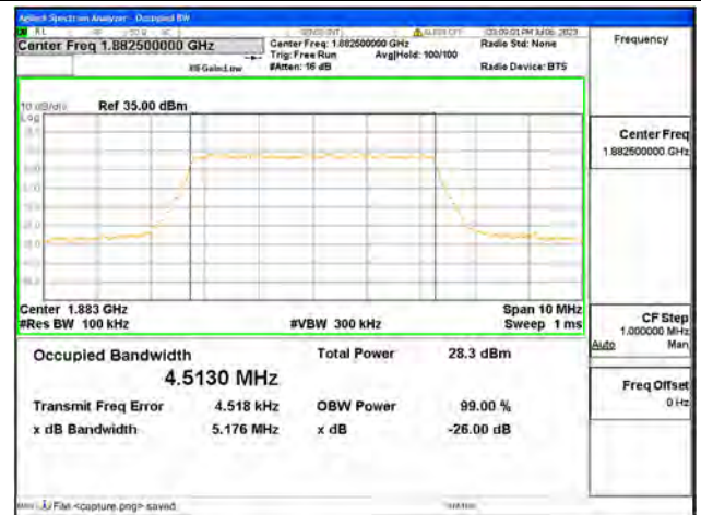
Band25 / 5MHz / QPSK/ Mid CH
