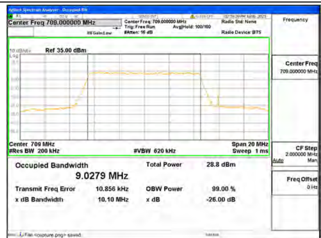
Band17 / 10MHz / 64QAM/ Low CH
