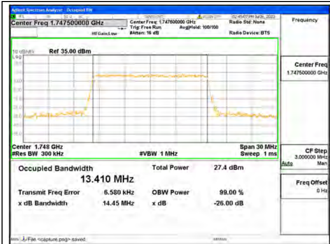
Band4 / 15MHz / QPSK/ High CH
