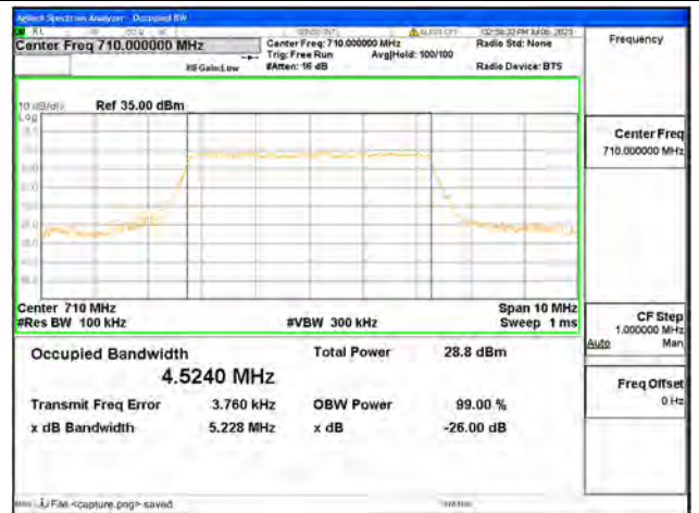
Band17 / 5MHz / QPSK/ Mid CH
