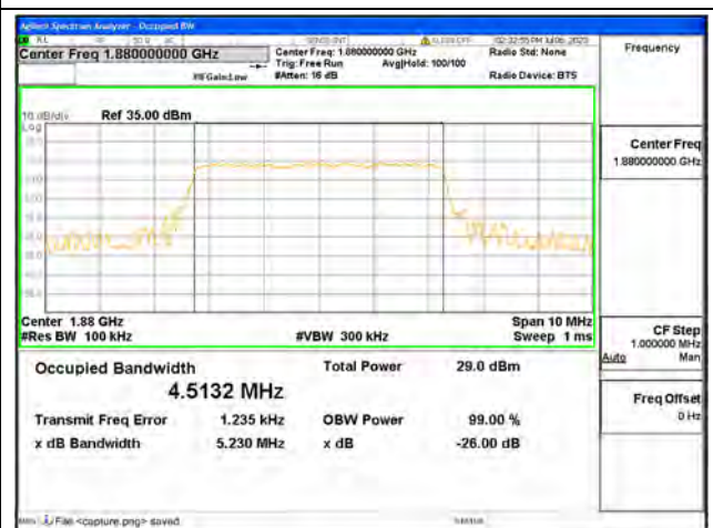
Band2 / 5MHz / 64QAM/ Mid CH
