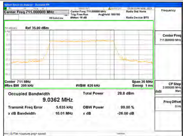
Band17 / 10MHz / QPSK/ High CH
