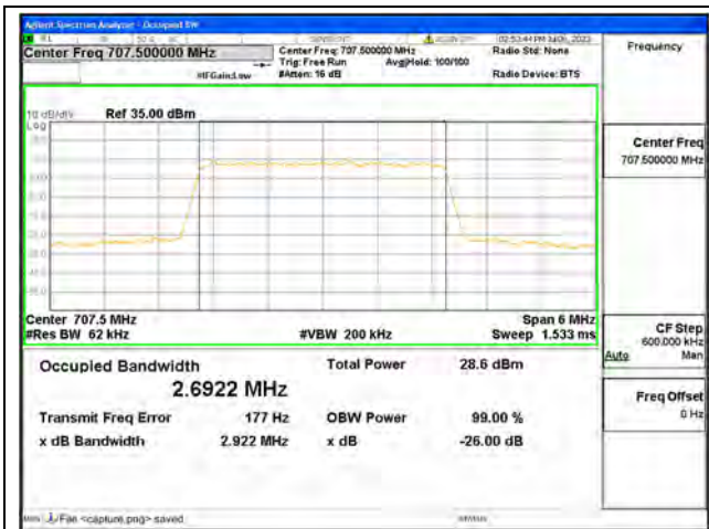
Band12 / 3MHz / QPSK/ Mid CH
