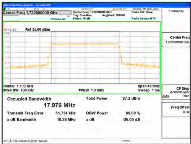
Band4 / 20MHz / 64QAM/ Mid CH
