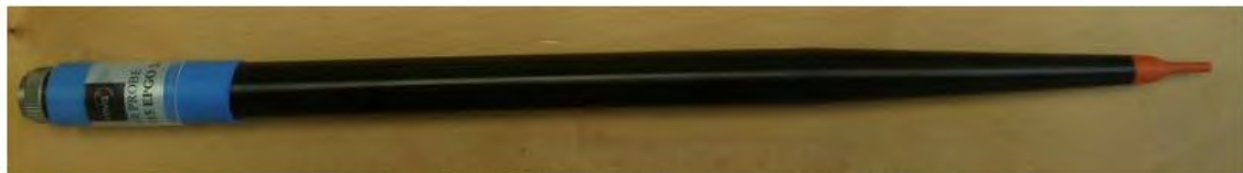
Figure 1 – MVG COMOSAR Dosimetric E field Dipole
