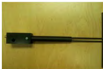
Figure 1 – MVG COMOSAR Validation Dipole
