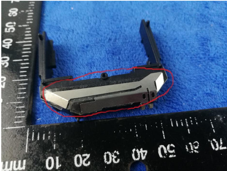
GSM/PCS - Antenna View
