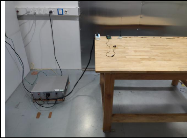
Conducted Emissions Test Setup Front View
