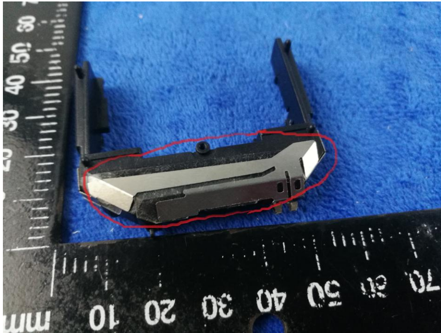
GSM/PCS - Antenna View
