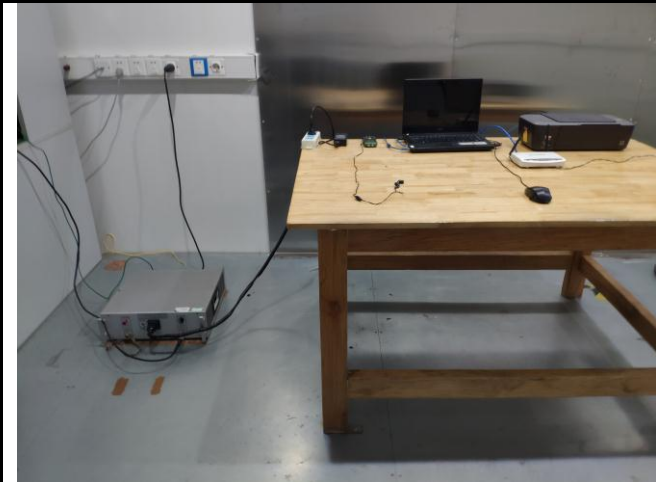
Conducted Emissions Test Setup – Front View
