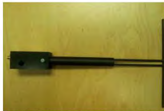
Figure 1 – MVG COMOSAR Validation Dipole
