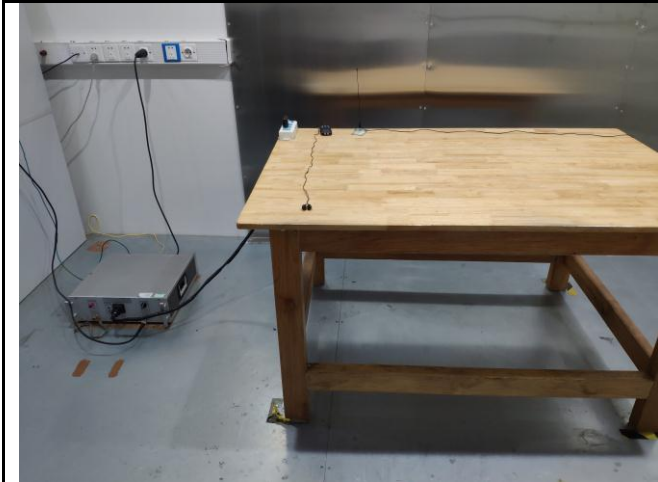
Conducted Emissions Test Setup Front View
