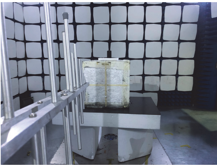
Radiation Emission Test Setup (30MHz to1GHz)
