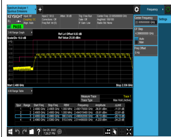
1-N41-PC3-30-40-L-6-CP-QPSK-Outer_Full-106@0-Ant1-1-X:2490.17MHz Y:-36.814dBm Margin:11.814-PASS-see graph
