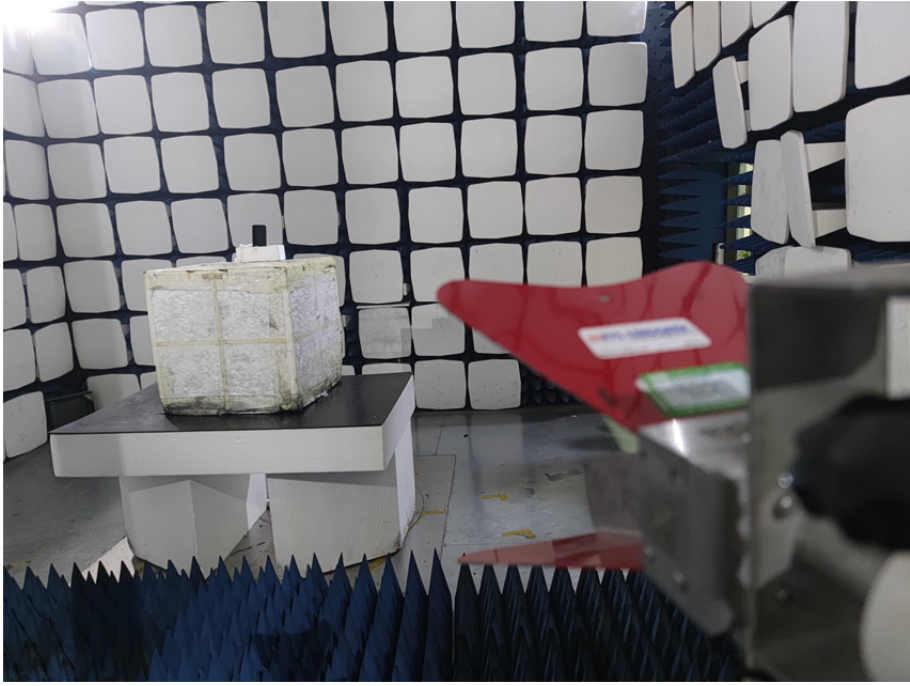
Radiation Emission Test Setup (1GHz to 18GHz)
