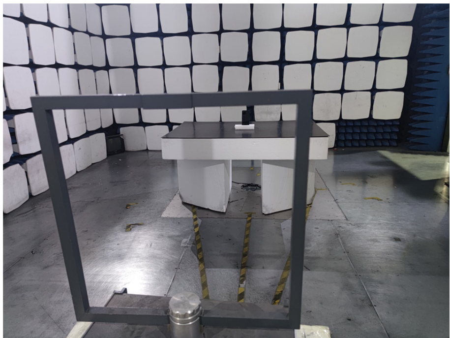
Radiation Emission Test Setup (Below 30MHz)
