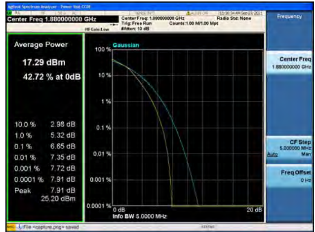
Band2 / 3MHz / High CH / QPSK
