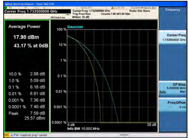
Band4 / 10MHz / High CH / QPSK
