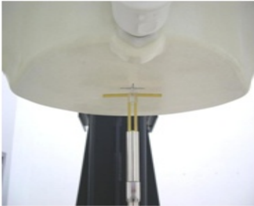
Fig 8.1 Photo of Dipole Setup Evaluation
