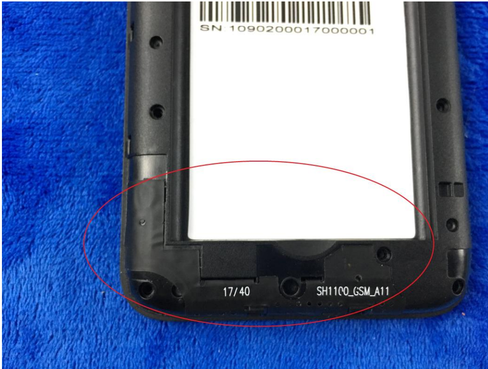
GSM/PCS/UMTS-FDD/LTE Antenna View
