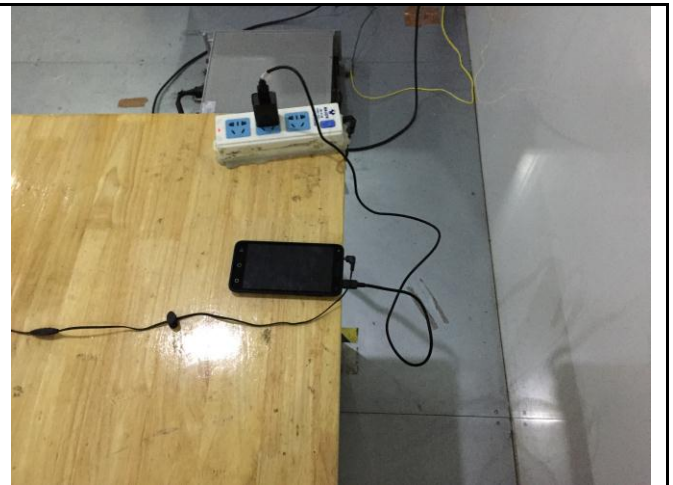
Conducted Emissions Test Setup Side View
