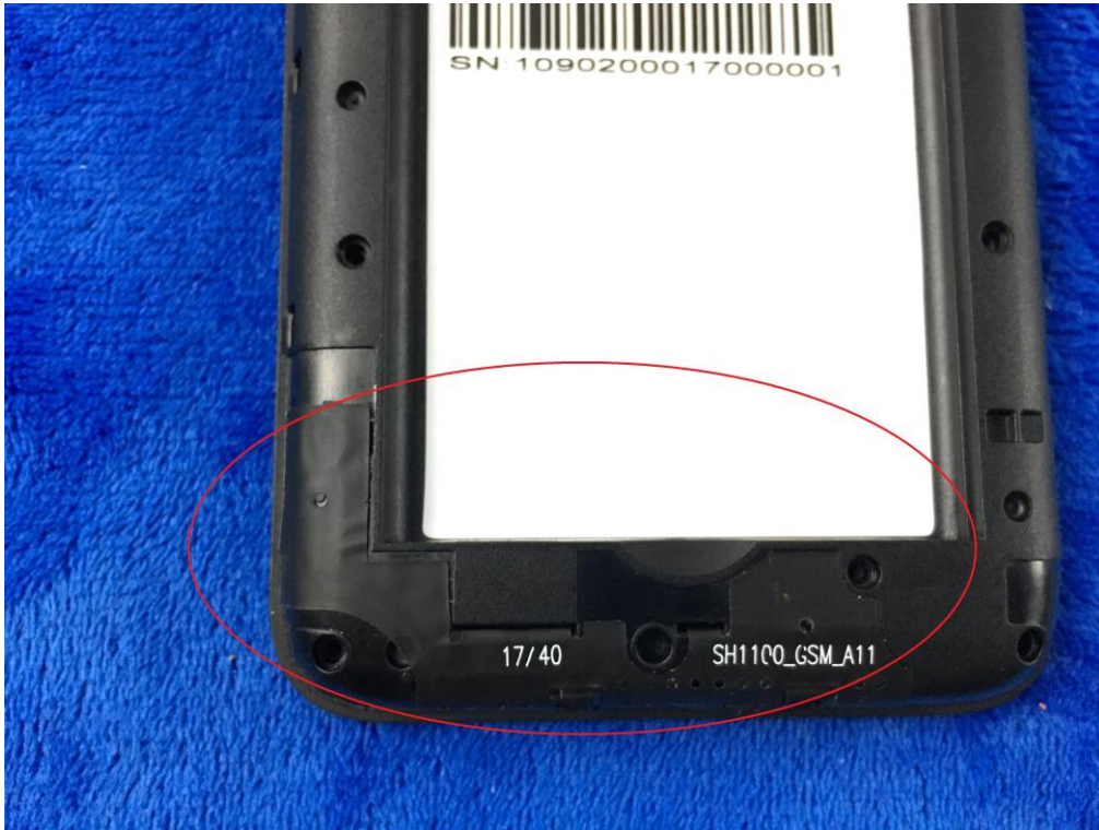
GSM/PCS/UMTS-FDD/ LTE Antenna View
