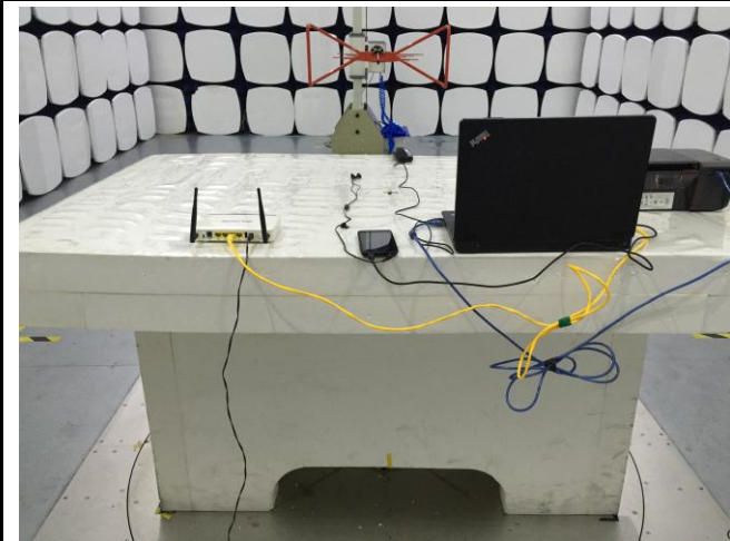
Radiated Emissions Test Setup Below 1GHz
