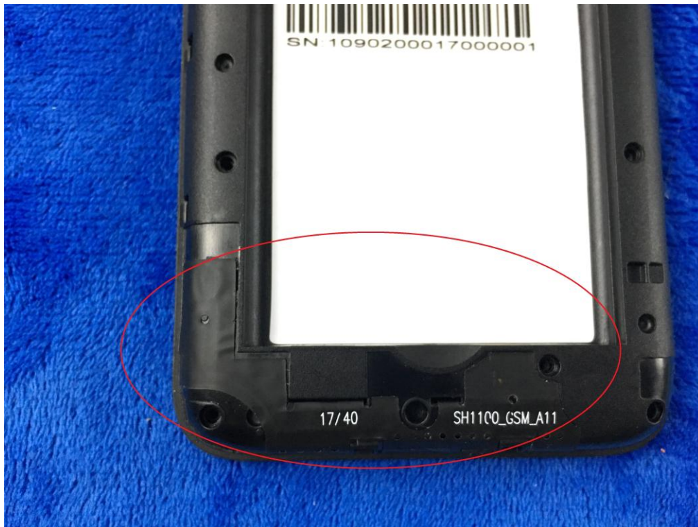
GSM/PCS/UMTS-FDD/LTE Antenna View
