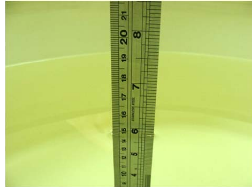
Fig 6.2 Photo of Liquid Height for Body SAR
