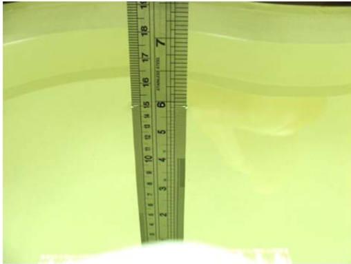
Fig 6.1 Photo of Liquid Height for Head SAR
