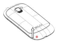
① Along the handle position(groove) of the Battery Cover
