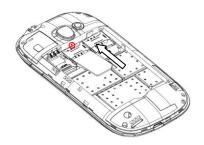
According to the diagram insert the SIM/USIM card 1
