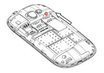
According to the diagram to insert SIM card 2
