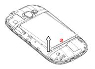
According to the diagram to remove the battery
