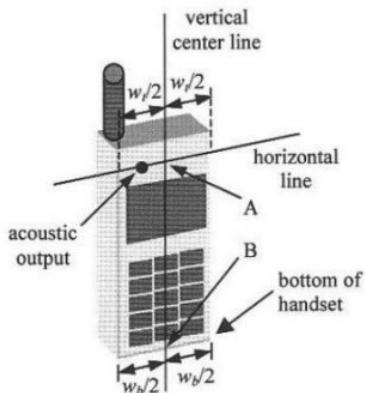
Fig 9.2.1 Handset vertical and horizontal reference lines—"fixed case"
