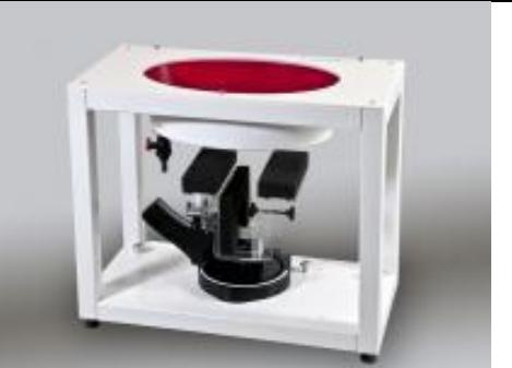
A photograph of the ELI Phantom. It is a white rectangular phantom with a red circular opening on top. A black device holder is positioned inside, and a black robotic arm is attached to the holder. The phantom is mounted on a white base. |
