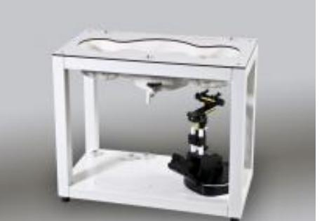
A photograph of the SAM Twin Phantom. It is a white rectangular phantom housed in a clear acrylic frame. A black device holder is positioned inside, and a black robotic arm is attached to the holder. The phantom is mounted on a white base with adjustable feet. |
