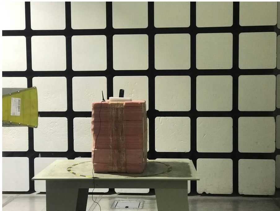
Radiated Emissions View (Above 1 GHz)
