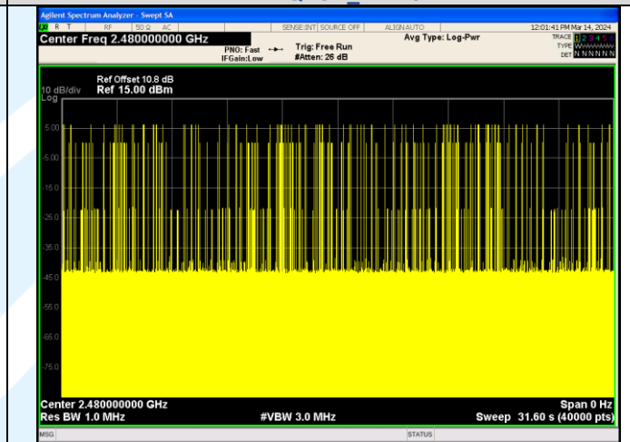
Number of Pulses in 31.6 seconds \pi/4 DQPSK 2-DH5
