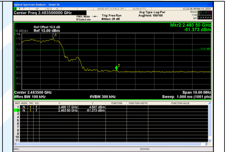
Out Of Band Emission(Right) 8DPSK_3-DH5_Channel Hopping
