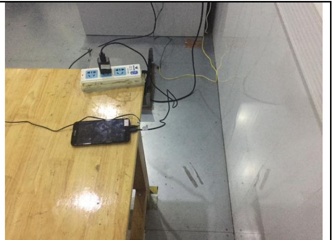
Conducted Emissions Test Setup Side View
