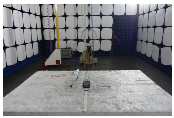
3. Radiated emission (9KHz-30MHz)
