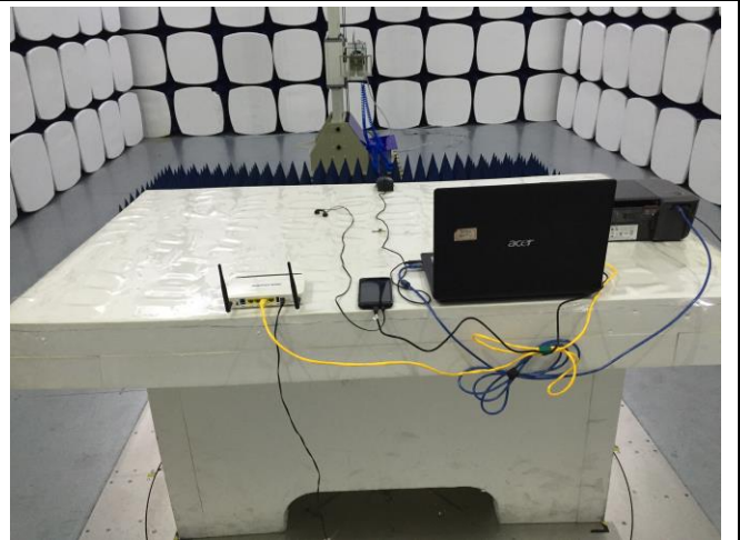
Radiated Emissions Test Setup Above 1GHz
