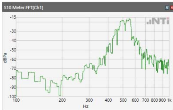
ANSI/TIA 5050-2018 \ 8N HAC OFF \ NB 12.2kbps\ 5.2 Receive path – distortion and noise\LTE Band 2
