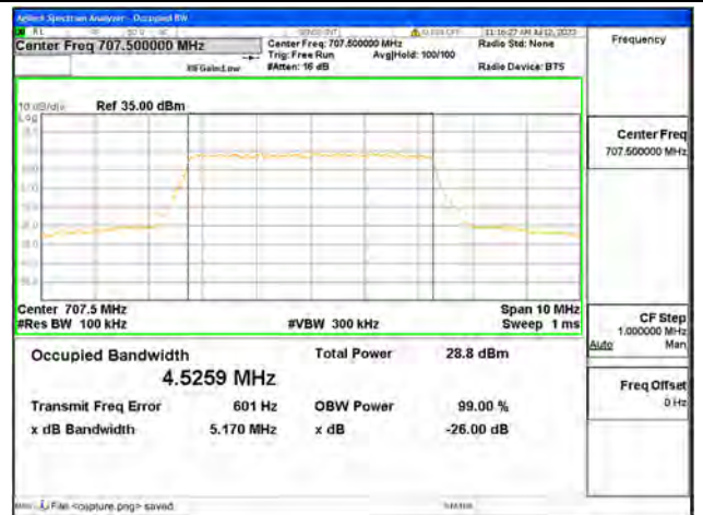
Band12 / 5MHz / 64QAM/ Mid CH
