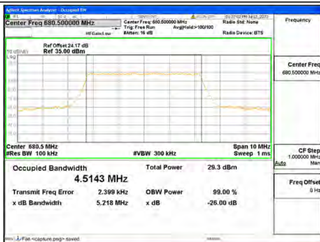
Band71 / 5MHz / 16QAM/ Mid CH
