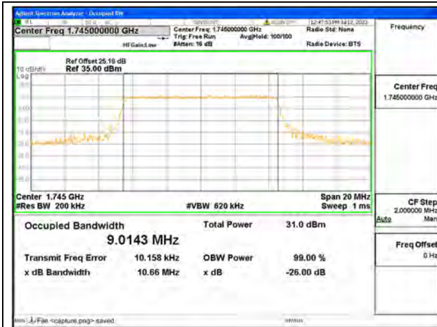
Band66 / 10MHz / QPSK/ Mid CH
