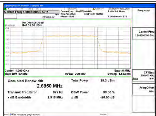
Band2 / 3MHz / QPSK/ High CH
