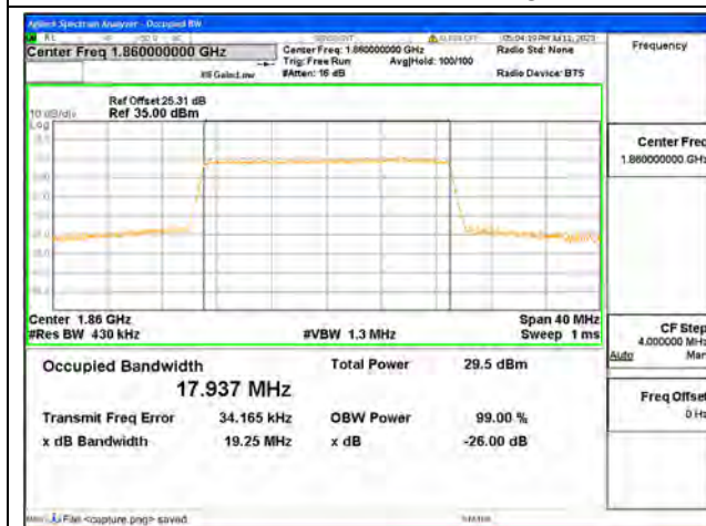
Band2 / 20MHz / 16QAM/ Low CH
