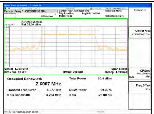
Band4 / 3MHz / 16QAM/ Mid CH
