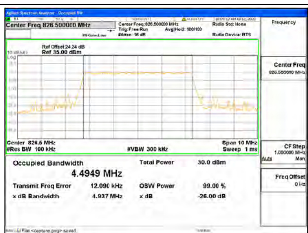
Band5 / 5MHz / 16QAM/ Low CH
