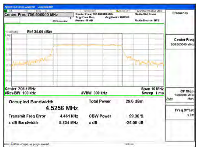
Band17 / 5MHz / 16QAM/ Low CH
