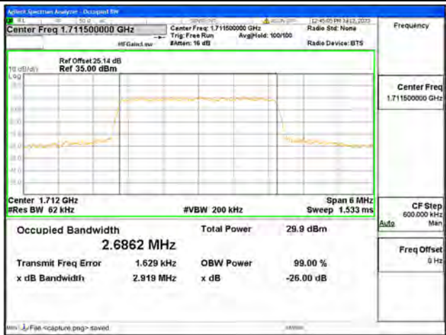
Band66 / 3MHz / 16QAM/ Low CH
