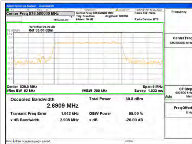
Band5 / 3MHz / QPSK/ Mid CH
