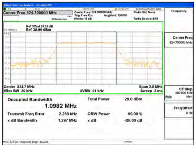
Band5 / 1.4MHz / 64QAM/ Low CH
