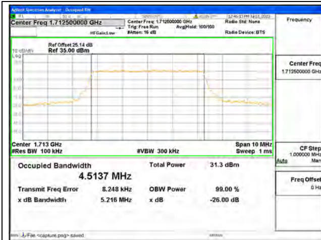
Band66 / 5MHz / QPSK/ Low CH
