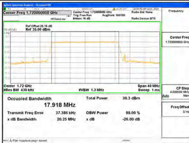
Band4 / 20MHz / 16QAM/ Low CH
