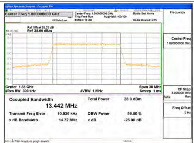
Band2 / 15MHz / 64QAM/ Mid CH
