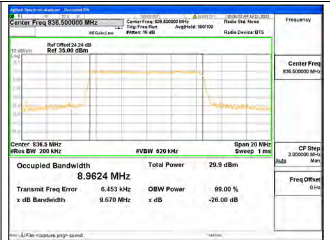
Band5 / 10MHz / 16QAM/ Mid CH
