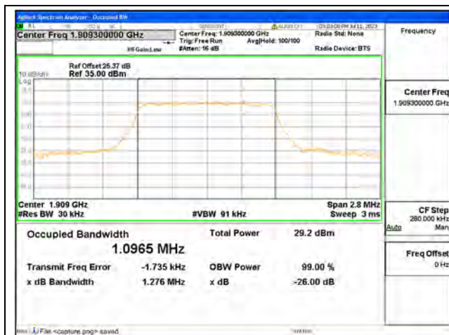
Band2 / 1.4MHz / QPSK/ High CH
