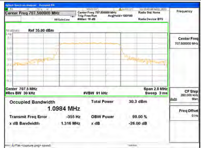
Band12 / 1.4MHz / QPSK/ Mid CH
