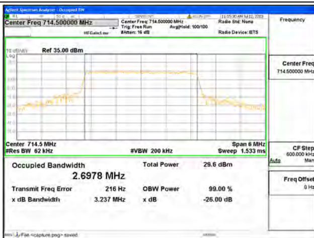
Band12 / 3MHz / 16QAM/ High CH
