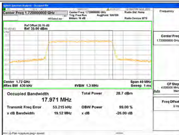
Band66 / 20MHz / 16QAM/ Low CH
