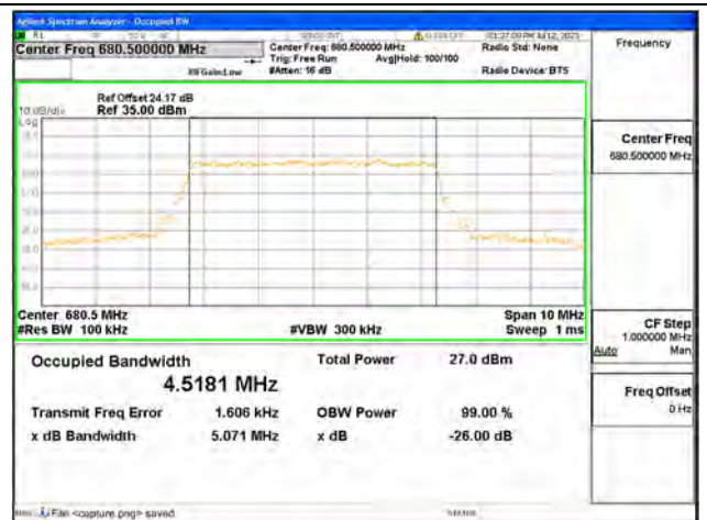
Band71 / 5MHz / 64QAM/ Mid CH
