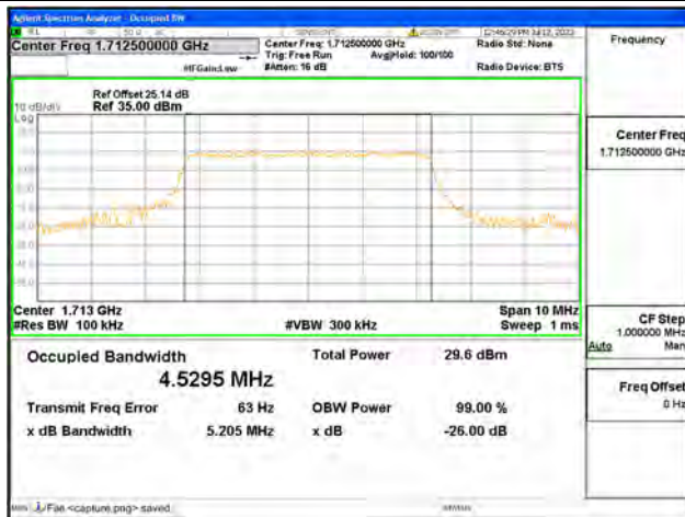
Band66 / 5MHz / 64QAM/ Low CH
