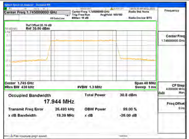
Band4 / 20MHz / QPSK/ High CH
