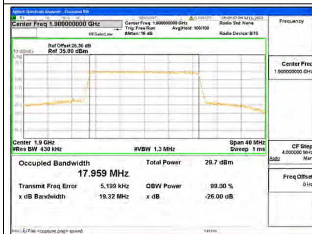
Band2 / 20MHz / 16QAM/ High CH
