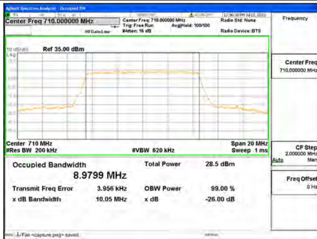
Band17 / 10MHz / 64QAM/ Mid CH
