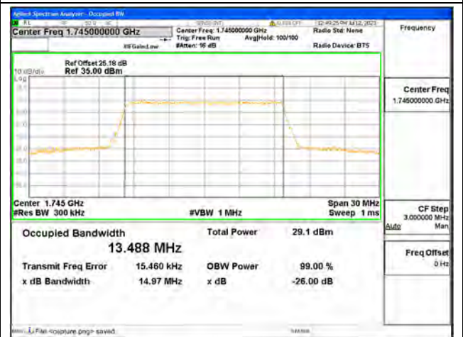
Band66 / 15MHz / 64QAM/ Mid CH
