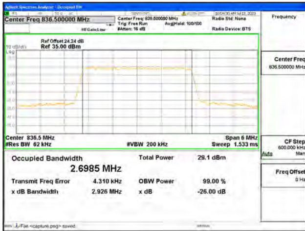
Band5 / 3MHz / 64QAM/ Mid CH
