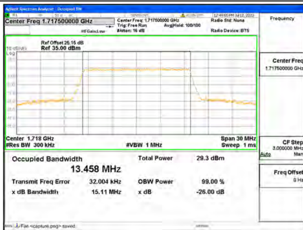
Band66 / 15MHz / 64QAM/ Low CH
