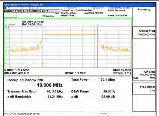
Band66 / 20MHz / 16QAM/ Mid CH
