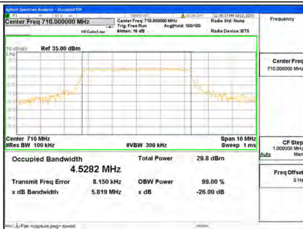
Band17 / 5MHz / 16QAM/ Mid CH
