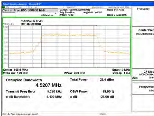
Band71 / 5MHz / 64QAM/ High CH
