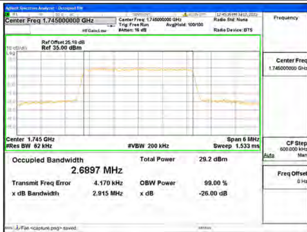
Band66 / 3MHz / 64QAM/ Mid CH
