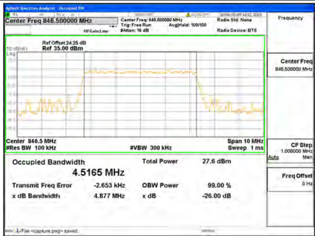
Band5 / 5MHz / 64QAM/ High CH
