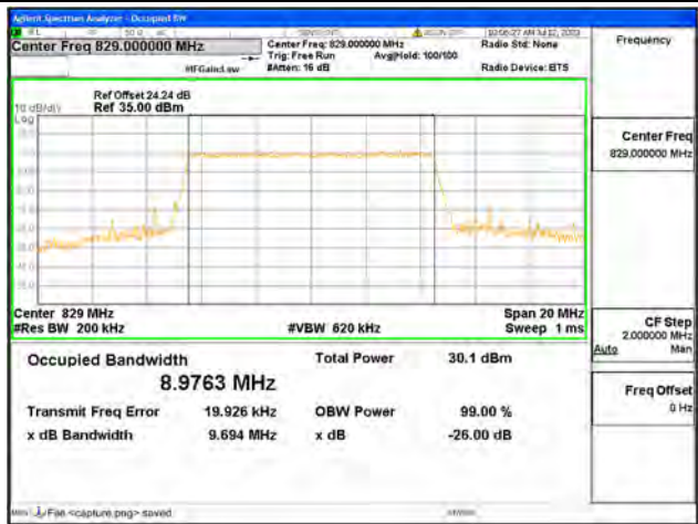
Band5 / 10MHz / 16QAM/ Low CH
