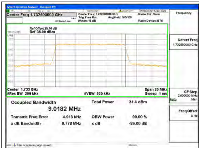
Band4 / 10MHz / QPSK/ Mid CH
