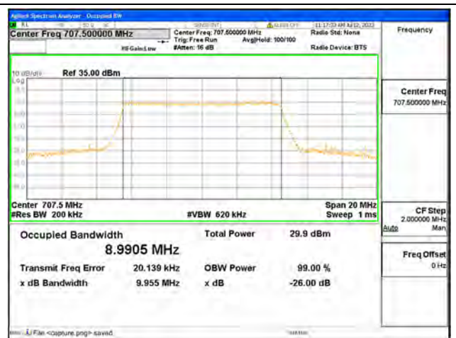
Band12 / 10MHz / 16QAM/ Mid CH
