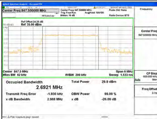
Band5 / 3MHz / 16QAM/ High CH
