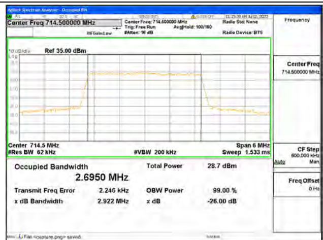
Band12 / 3MHz / 64QAM/ High CH
