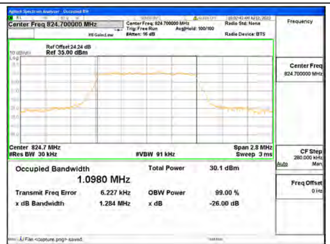
Band5 / 1.4MHz / 16QAM/ Low CH
