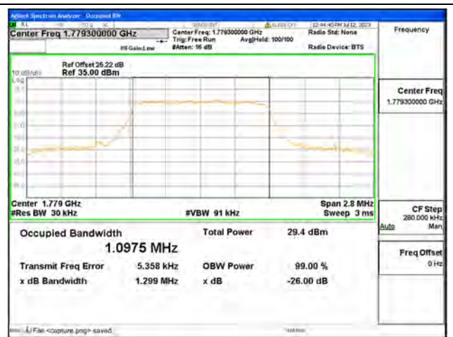
Band66 / 1.4MHz / 16QAM/ High CH
