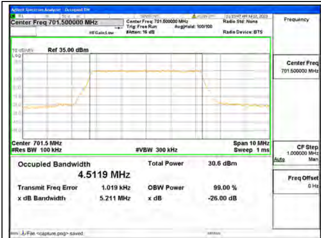
Band12 / 5MHz / QPSK/ Low CH
