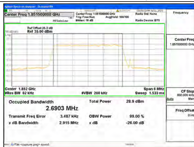
Band2 / 3MHz / QPSK/ Low CH
