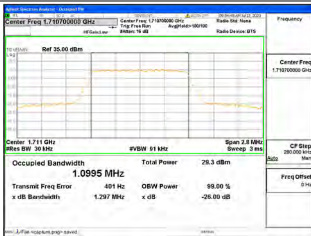
Band4 / 1.4MHz / 64QAM/ Low CH
