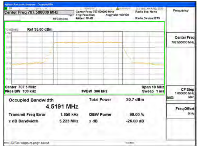
Band12 / 5MHz / QPSK/ Mid CH
