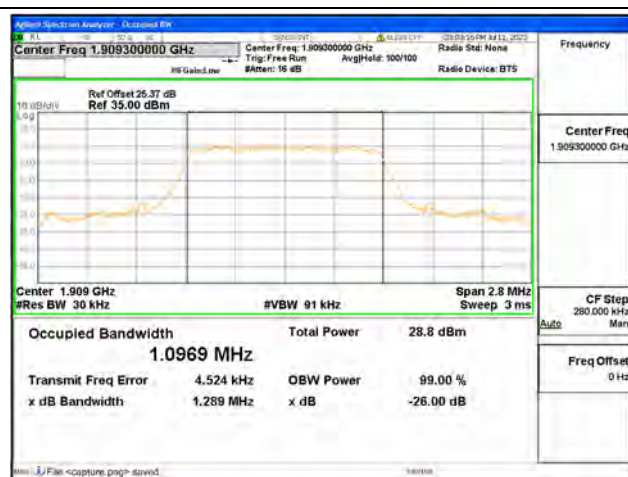
Band2 / 1.4MHz / 16QAM/ High CH
