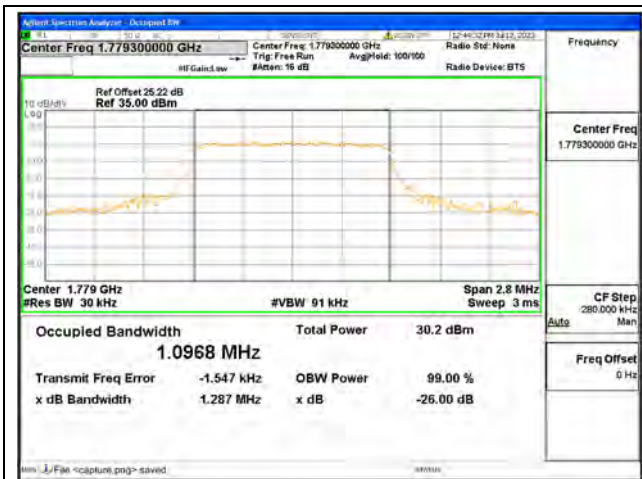
Band66 / 1.4MHz / QPSK/ High CH
