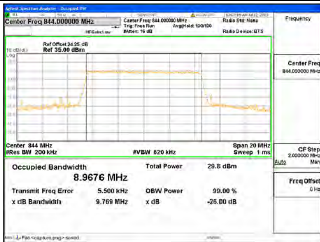
Band5 / 10MHz / 16QAM/ High CH
