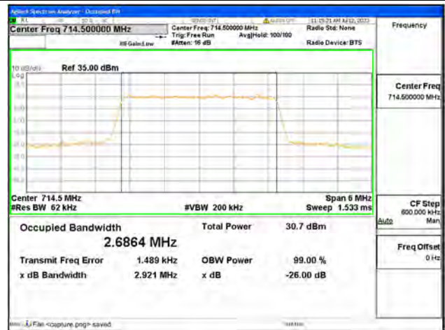
Band12 / 3MHz / QPSK/ High CH
