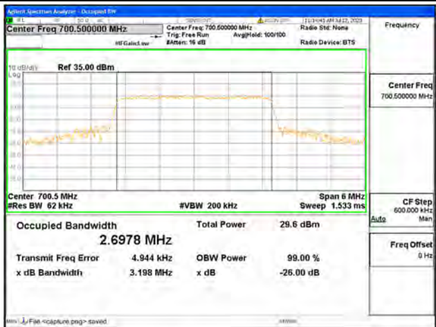
Band12 / 3MHz / 16QAM/ Low CH
