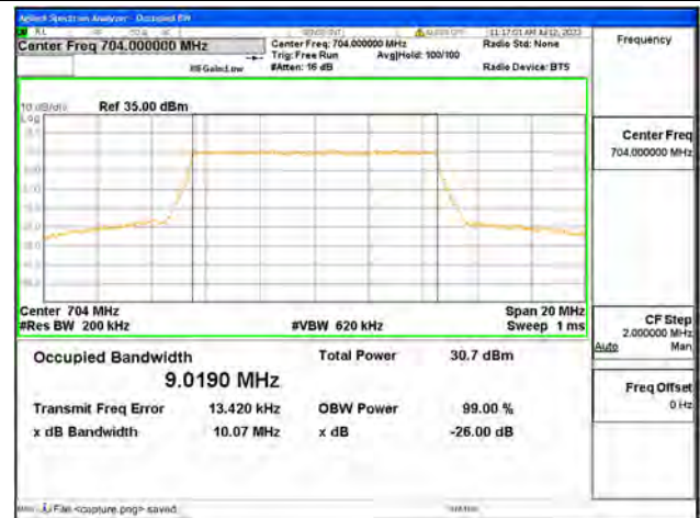
Band12 / 10MHz / QPSK/ Low CH
