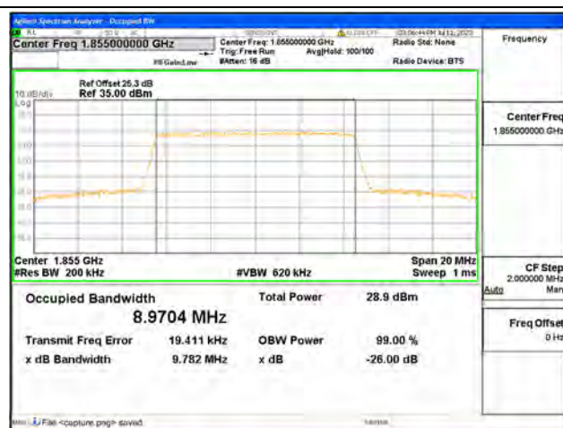
Band2 / 10MHz / 64QAM/ Low CH
