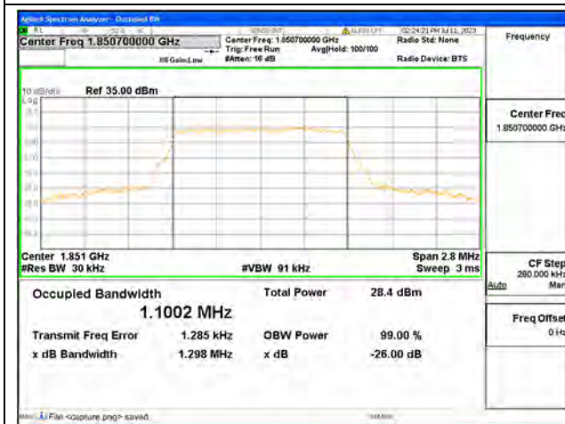
Band2 / 1.4MHz / 64QAM/ Low CH
