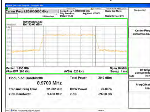
Band2 / 10MHz / 16QAM/ Low CH
