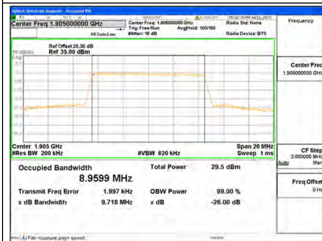
Band2 / 10MHz / 16QAM/ High CH
