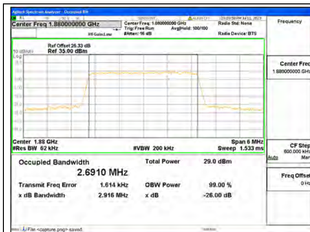
Band2 / 3MHz / QPSK/ Mid CH
