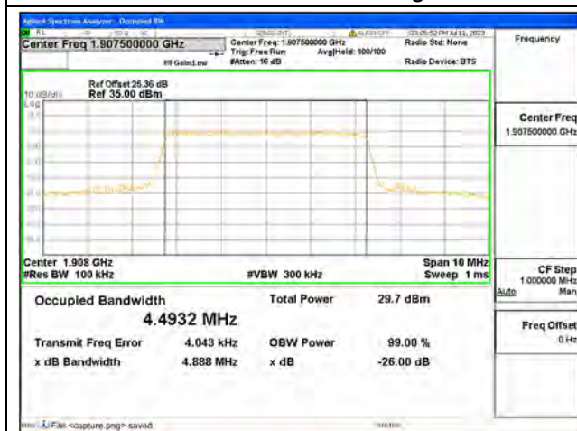
Band2 / 5MHz / 64QAM/ High CH
