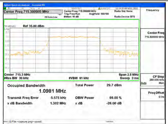
Band12 / 1.4MHz / 16QAM/ High CH
