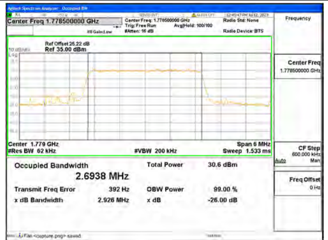
Band66 / 3MHz / QPSK/ High CH
