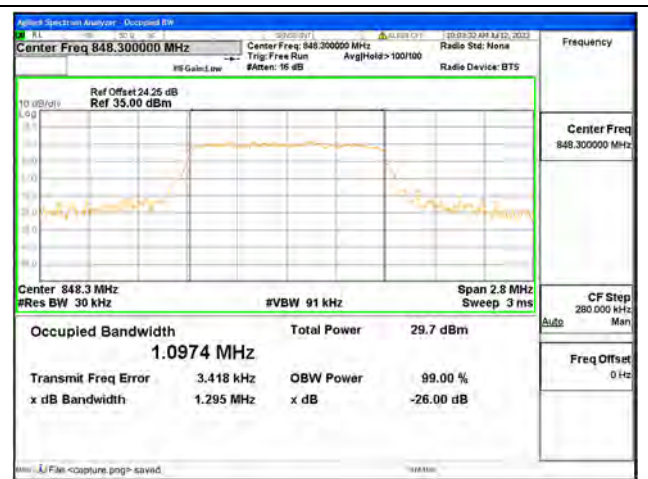
Band5 / 1.4MHz / 16QAM/ High CH
