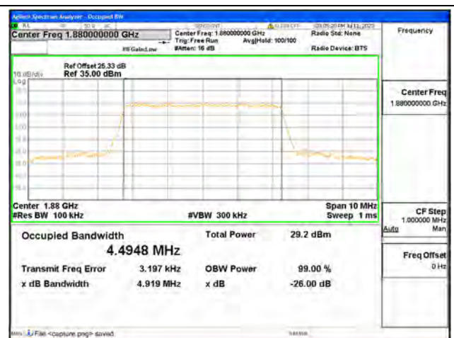
Band2 / 5MHz / 64QAM/ Mid CH
