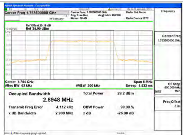
Band4 / 3MHz / 64QAM/ High CH
