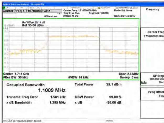
Band66 / 1.4MHz / 64QAM/ Low CH
