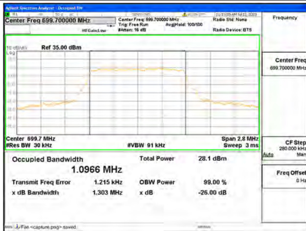
Band12 / 1.4MHz / 64QAM/ Low CH
