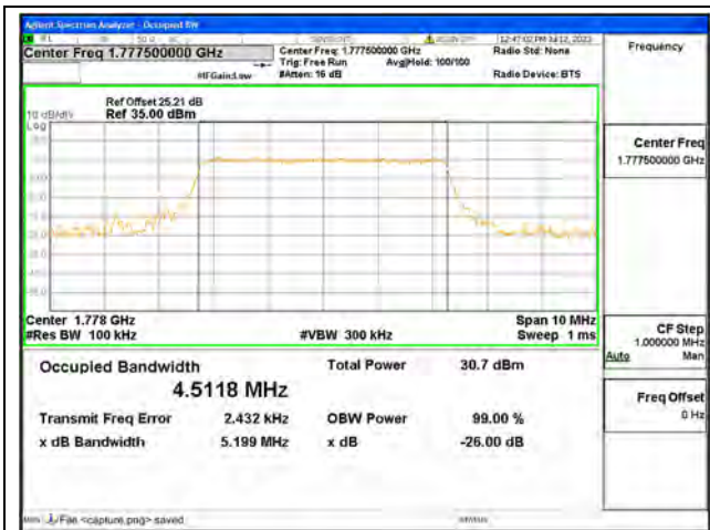
Band66 / 5MHz / QPSK/ High CH
