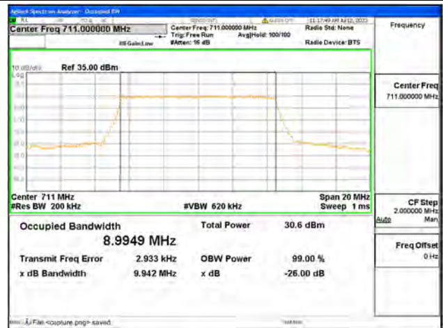
Band12 / 10MHz / QPSK/ High CH
