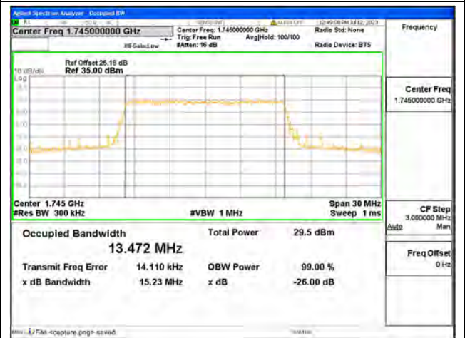
Band66 / 15MHz / QPSK/ Mid CH
