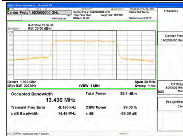
Band2 / 15MHz / 64QAM/ High CH
