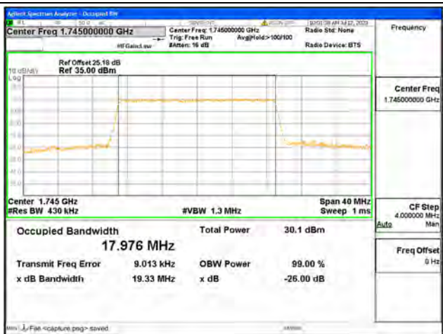
Band4 / 20MHz / 16QAM/ High CH
