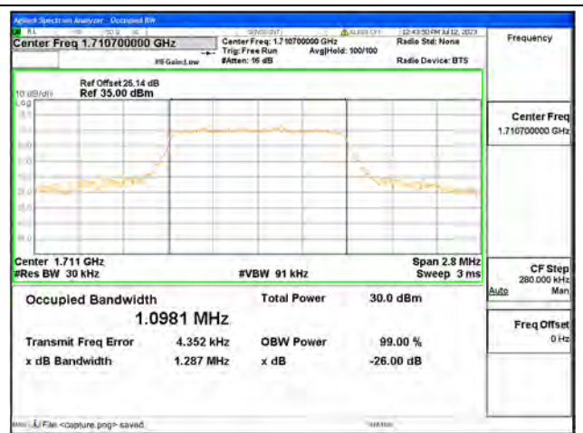
Band66 / 1.4MHz / 16QAM/ Low CH
