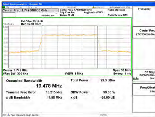
Band4 / 15MHz / 64QAM/ High CH
