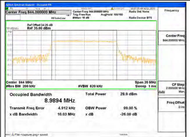
Band5 / 10MHz / 64QAM/ High CH
