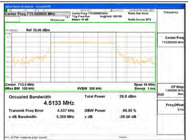
Band17 / 5MHz / 16QAM/ High CH
