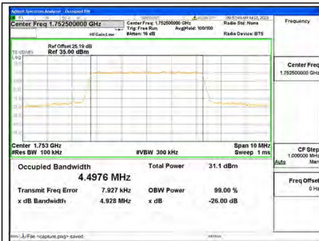
Band4 / 5MHz / QPSK/ High CH
