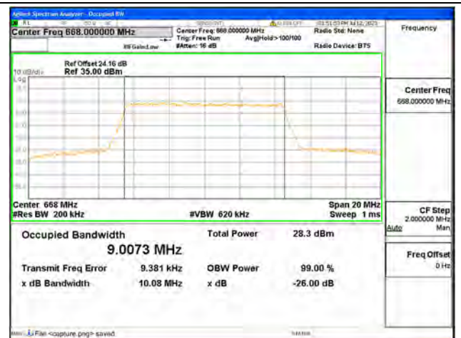
Band71 / 10MHz / 64QAM/ Low CH
