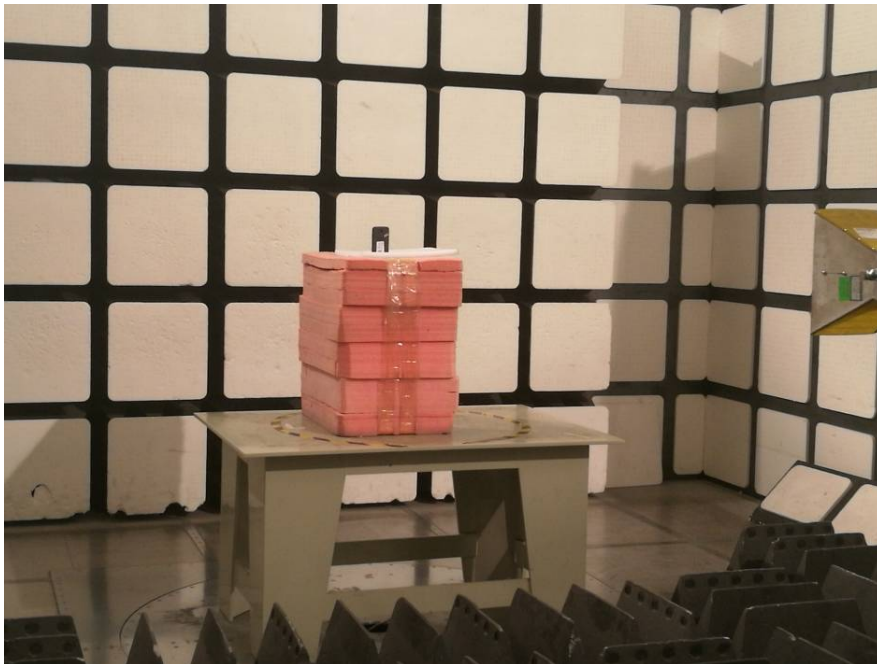
Radiated Emissions View (Above 1 GHz)
