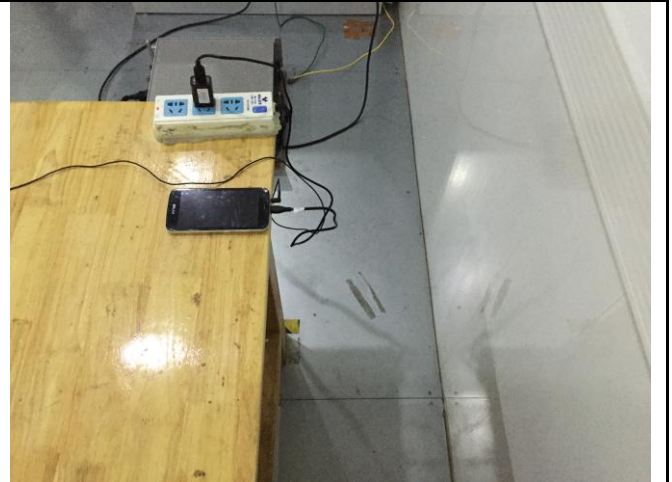
Conducted Emissions Test Setup Side View
