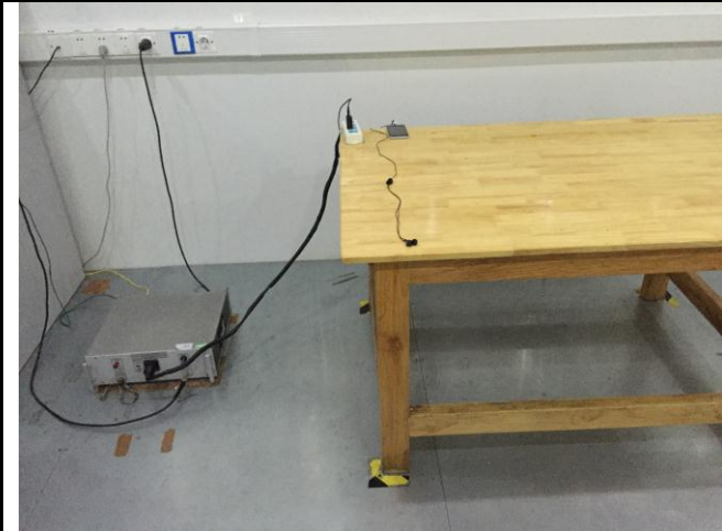
Conducted Emissions Test Setup Front View
