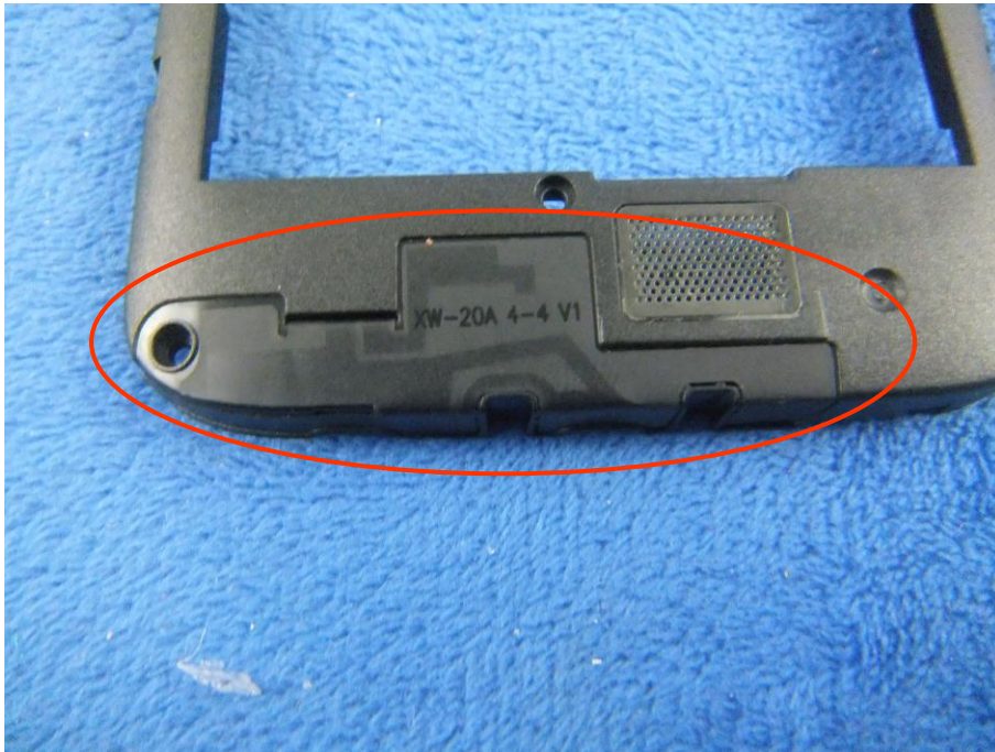
GSM/PCS/UMTS-FDD - Antenna View
