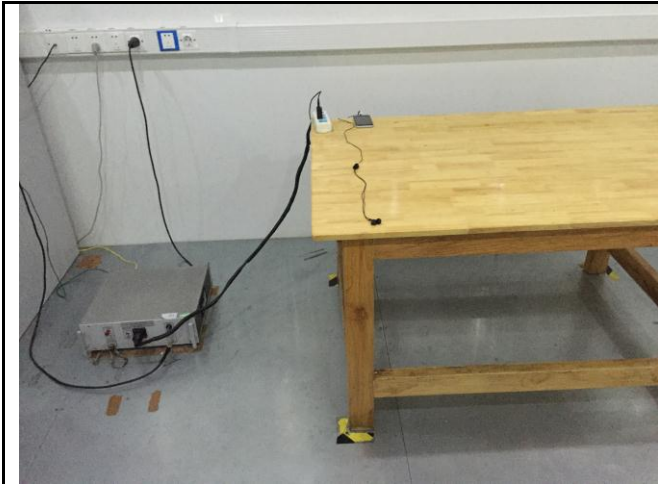
Conducted Emissions Test Setup Front View
