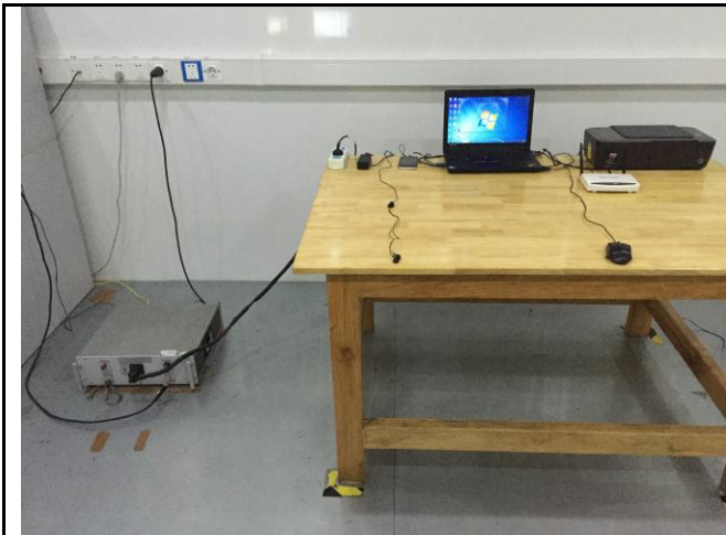
Conducted Emissions Test Setup – Front View
