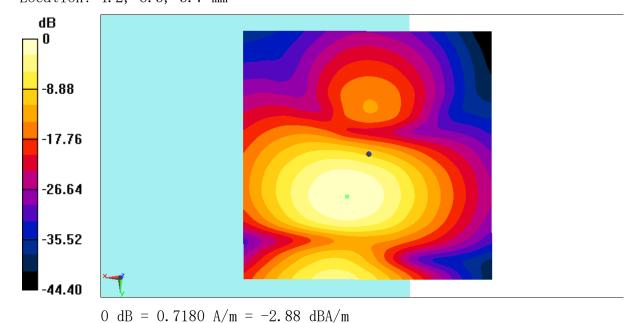
Fig B.1 T-Coil LTEB13
