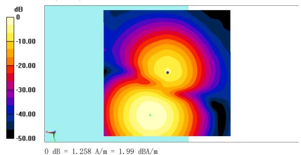
Fig B.2 T-Coil LTEB12
