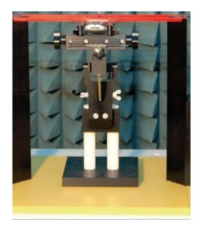
Figure 5.4 HAC Phantom & Device Holder
