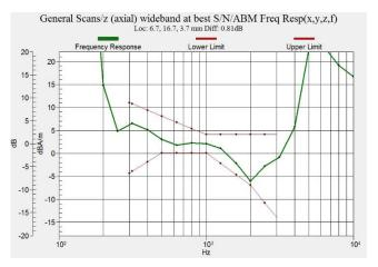
Figure C.1 Frequency Response of LTEB12
