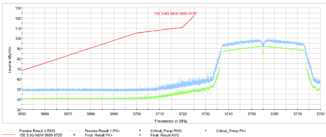
Fig. 80 Band Edges (802.11ac-HT20 Ch165, 5825MHz)
