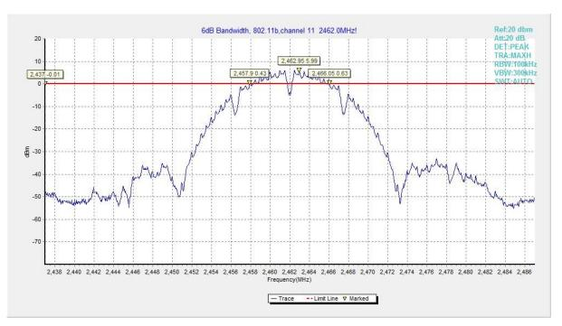
Fig.12 6dB Bandwidth (802.11b, CH 11)
