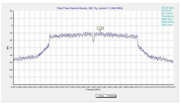
Fig.6 Power Spectral Density (802.11g, CH 11)
