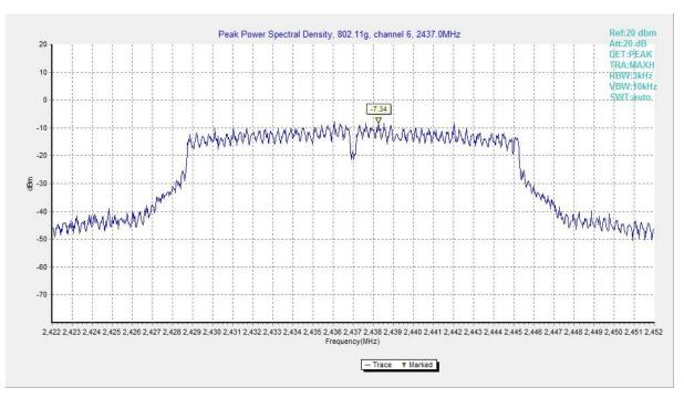
Fig.5 Power Spectral Density (802.11g, CH 6)
