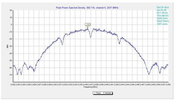
Fig.2 Power Spectral Density (802.11b, CH 6)
