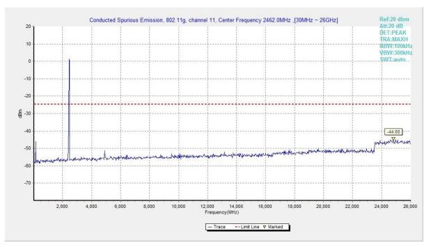
Fig.30 Conducted Spurious Emission (802.11g, CH11)
