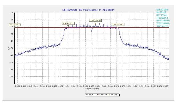
Fig.18 6dB Bandwidth (802.11n HT20, CH 11)
