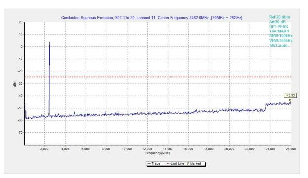
Fig.33 Conducted Spurious Emission (802.11n HT20, CH11)
