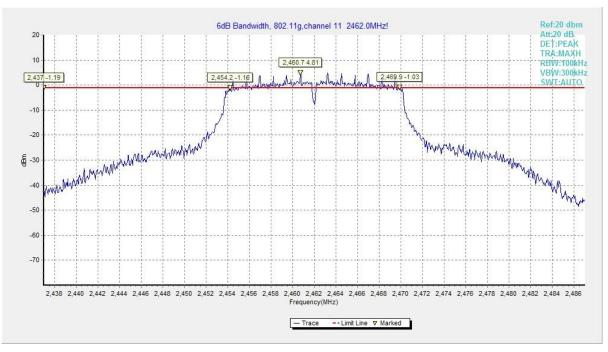
Fig.15 6dB Bandwidth (802.11g, CH 11)
