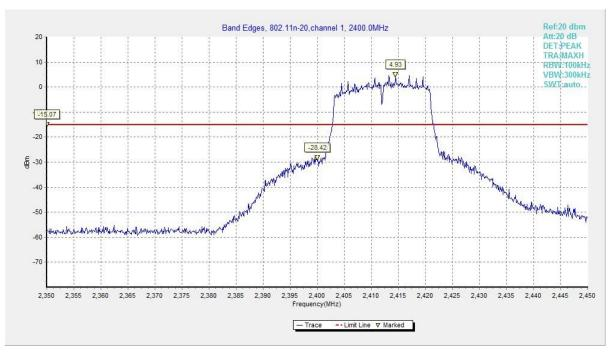
Fig.23 Band Edges (802.11n HT20, CH 1)
