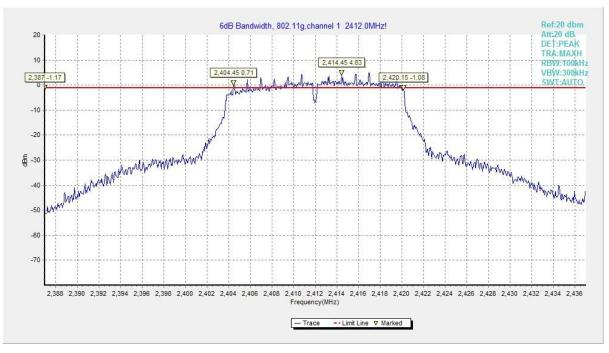
Fig.13 6dB Bandwidth (802.11g, CH 1)
