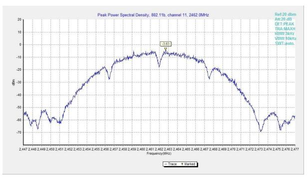
Fig.3 Power Spectral Density (802.11b, CH 11)
