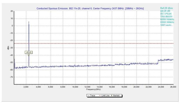
Fig.32 Conducted Spurious Emission (802.11n HT20, CH6)
