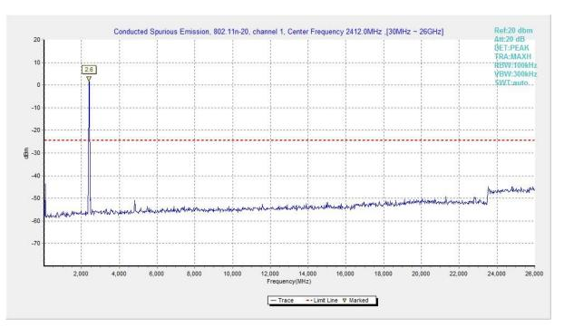
Fig.31 Conducted Spurious Emission (802.11n HT20, CH1)
