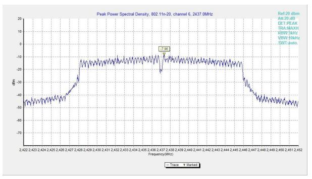
Fig.8 Power Spectral Density (802.11n HT20, CH 6)
