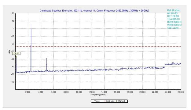
Fig.27 Conducted Spurious Emission (802.11b, CH11)
