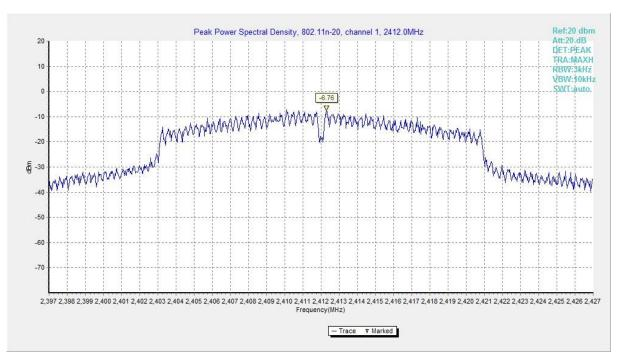
Fig.7 Power Spectral Density (802.11n HT20, CH 1)
