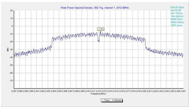
Fig.4 Power Spectral Density (802.11g, CH 1)
