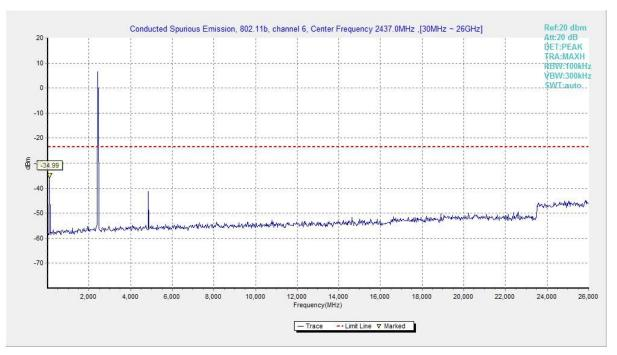
Fig.26 Conducted Spurious Emission (802.11b, CH6)
