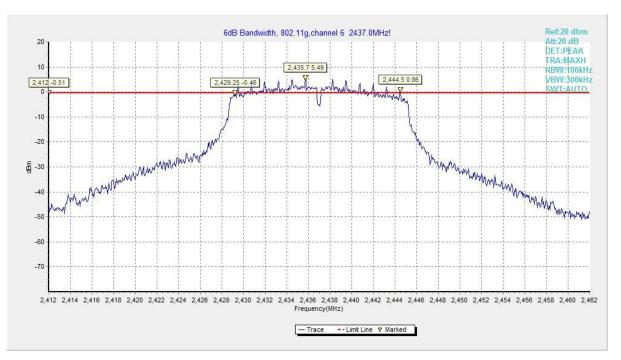
Fig.14 6dB Bandwidth (802.11g, CH 6)
