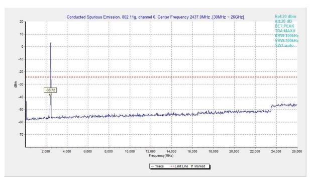
Fig.29 Conducted Spurious Emission (802.11g, CH6)
