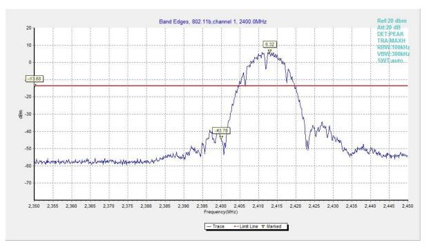
Fig.19 Band Edges (802.11b, CH 1)
