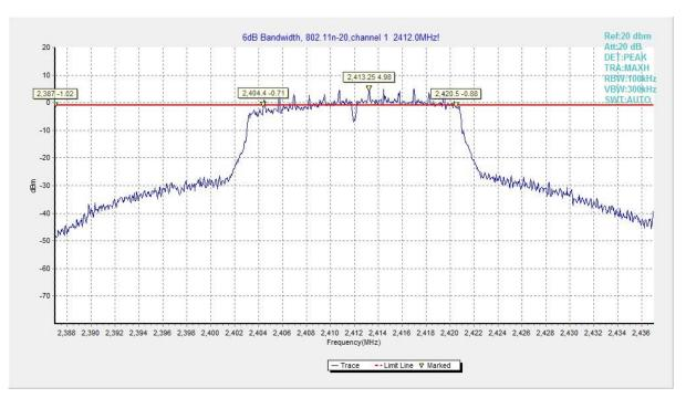
Fig.16 6dB Bandwidth (802.11n HT20, CH 1)
