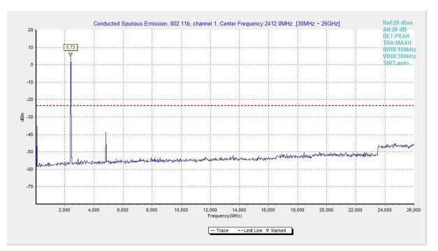
Fig.25 Conducted Spurious Emission (802.11b, CH1)
