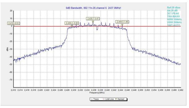
Fig.17 6dB Bandwidth (802.11n HT20, CH 6)
