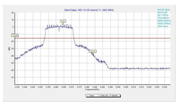
Fig.24 Band Edges (802.11n HT20, CH 11)
