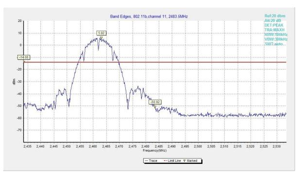
Fig.20 Band Edges (802.11b, CH 11)
