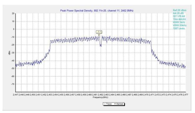
Fig.9 Power Spectral Density (802.11n HT20, CH 11)
