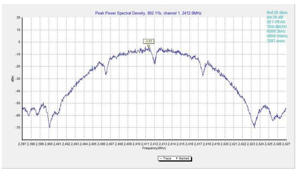
Fig.1 Power Spectral Density (802.11b, CH 1)
