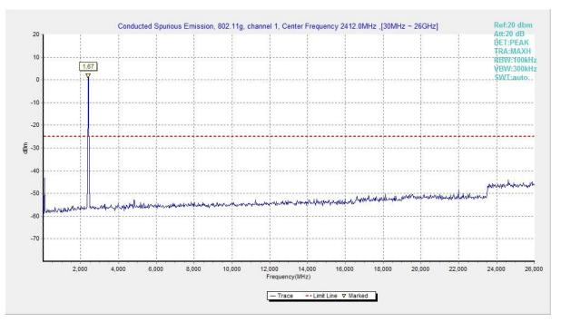
Fig.28 Conducted Spurious Emission (802.11g, CH1)
