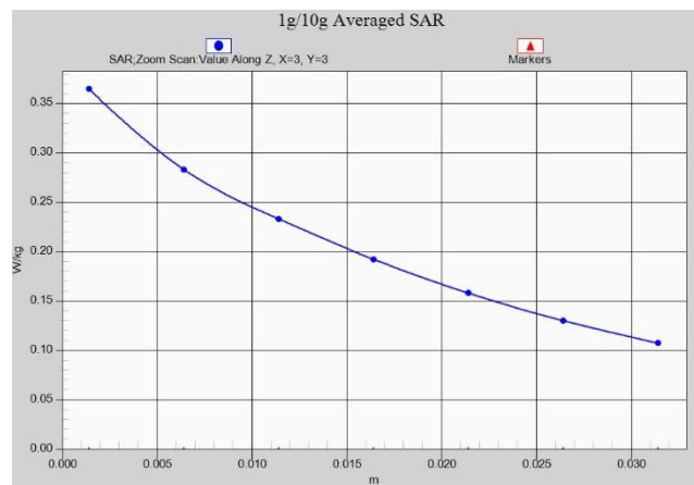
Fig. A-30 Z-Scan at power reference point (LTE Band71)
