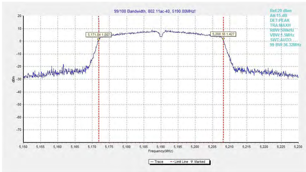
Fig.66 99% Occupied bandwidth (802.11ac-HT40, 5190MHz)
