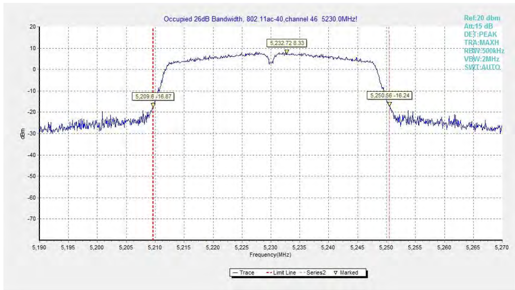
Fig.22 Occupied 26dB Bandwidth (802.11ac-HT40, 5230MHz)
