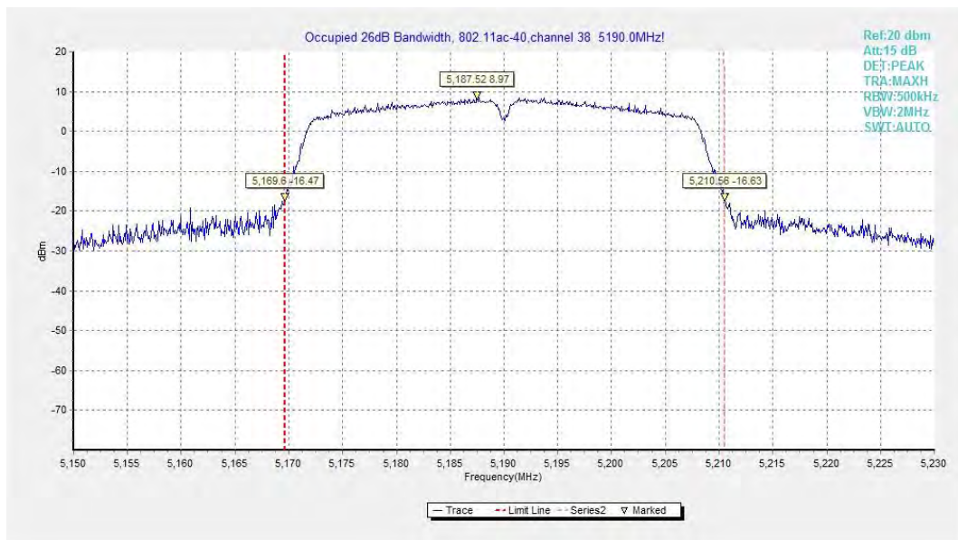
Fig.21 Occupied 26dB Bandwidth (802.11ac-HT40, 5190MHz)
