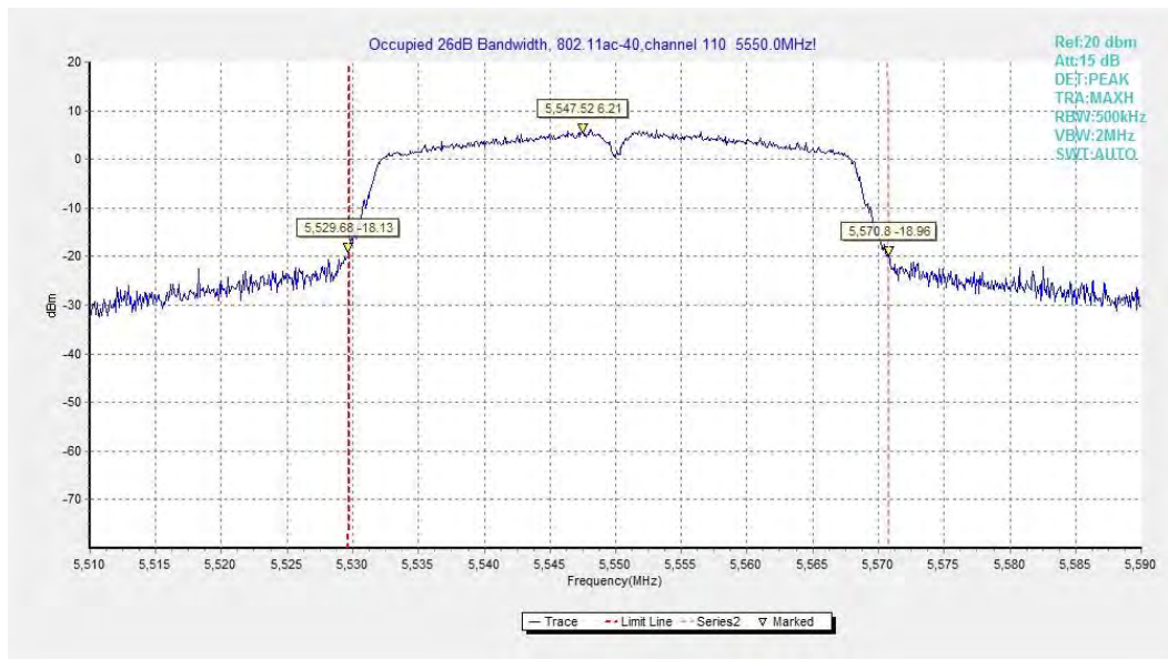
Fig.26 Occupied 26dB Bandwidth (802.11ac-HT40, 5550MHz)
