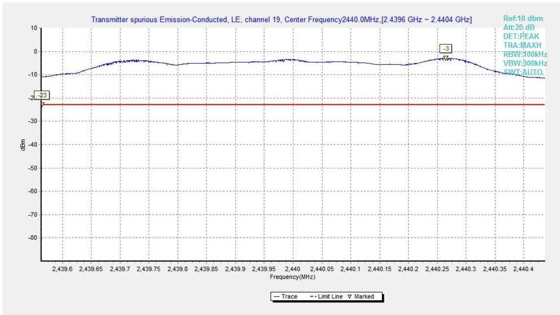
Fig.10. Transmitter Spurious Emission - Conducted: GFSK, 2440MHz
