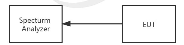
The EUT which is powered by the Battery, is connected to the Spectrum Analyzer; the RF load attached to the EUT antenna terminal is 50 Ohm; the path loss as the factor is calibrated to correct the reading. Make the measurement with the spectrum analyzer's resolution bandwidth(RBW) = 100 kHz. In order to make an accurate measurement, set the span greater than RBW.
