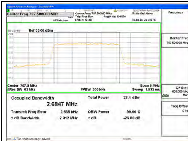
B12 / 3MHz / QPSK/ Mid CH
