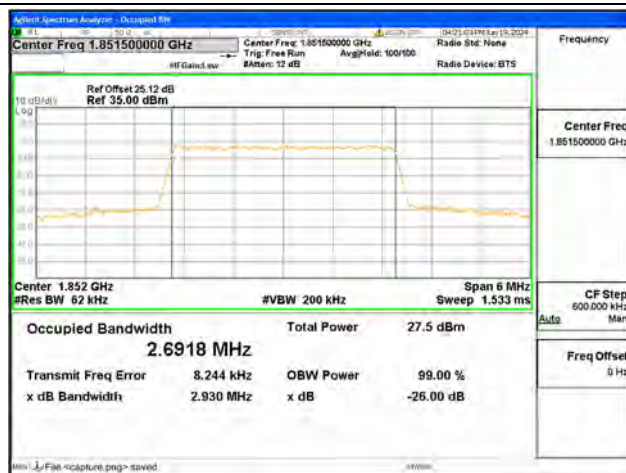
B2 / 3MHz / 16QAM/ Low CH
