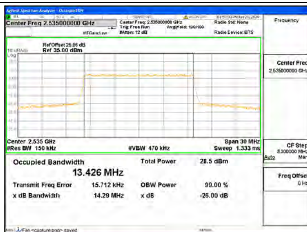
B7 / 15MHz / 16QAM/ Mid CH
