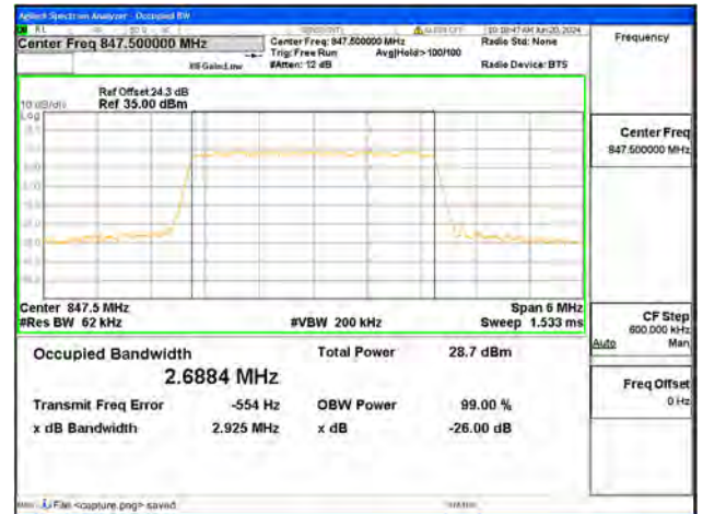
B5 / 3MHz / QPSK/ High CH
