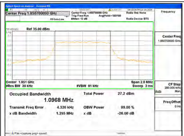
B2 / 1.4MHz / 16QAM/ Low CH
