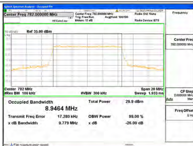
B13 / 10MHz / 16QAM/ Mid CH
