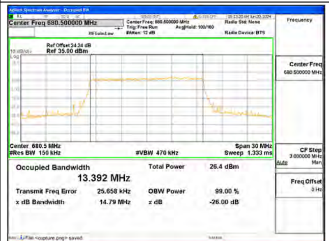
B71 / 15MHz / 64QAM/ Mid CH
