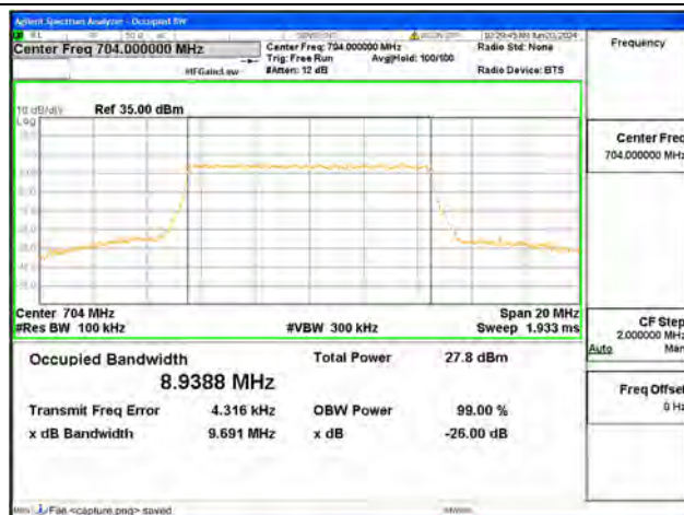
B12 / 10MHz / 16QAM/ Low CH
