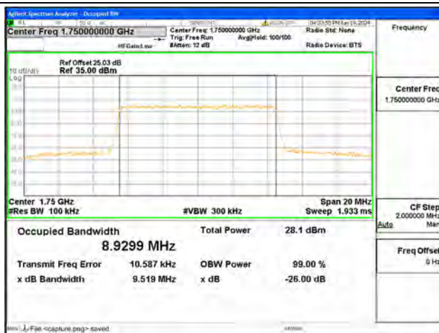
B4 / 10MHz / 16QAM/ High CH
