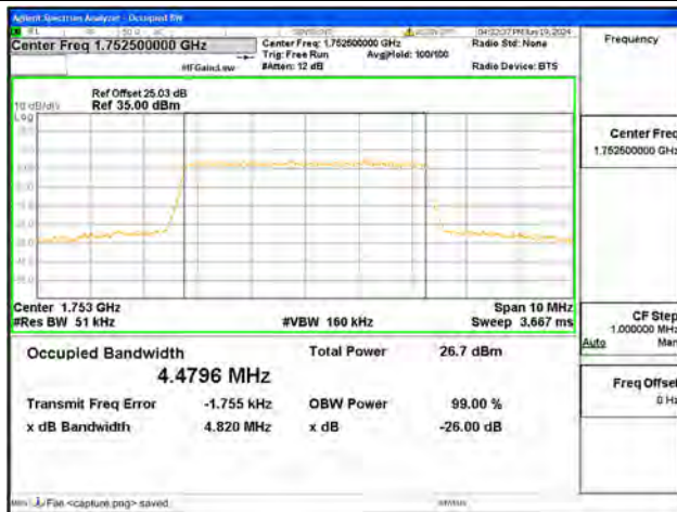
B4 / 5MHz / 64QAM/ High CH
