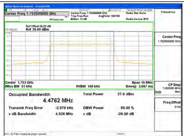
B4 / 5MHz / 16QAM/ High CH
