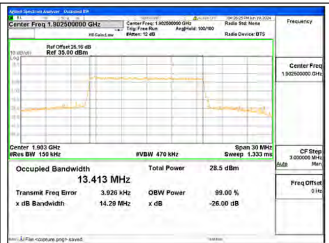
B2 / 15MHz / 16QAM/ High CH
