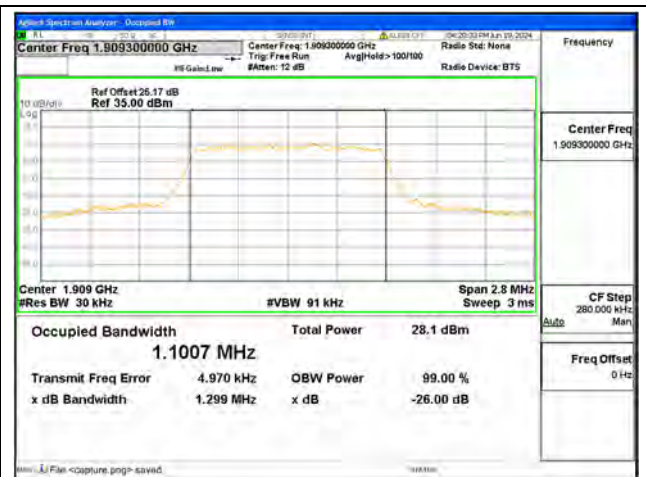
B2 / 1.4MHz / 16QAM/ High CH
