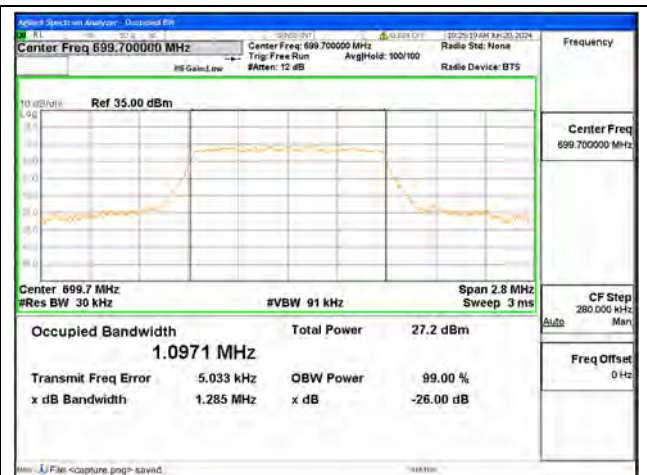
B12 / 1.4MHz / 16QAM/ Low CH
