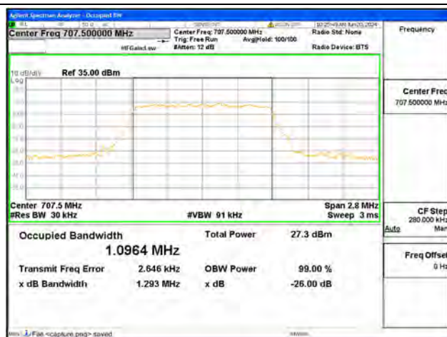
B12 / 1.4MHz / 16QAM/ Mid CH
