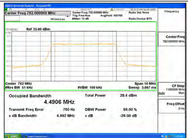
B13 / 5MHz / 64QAM/ Mid CH
