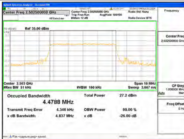
B7 / 5MHz / 64QAM/ Low CH
