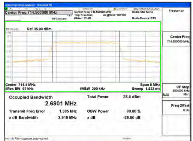
B12 / 3MHz / QPSK/ High CH
