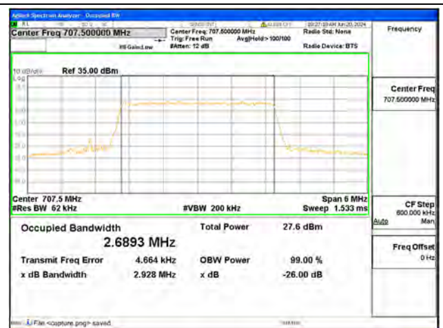
B12 / 3MHz / 16QAM/ Mid CH
