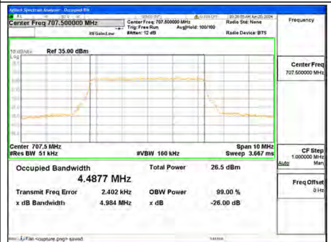
B12 / 5MHz / 64QAM/ Mid CH
