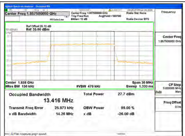
B2 / 15MHz / 16QAM/ Low CH
