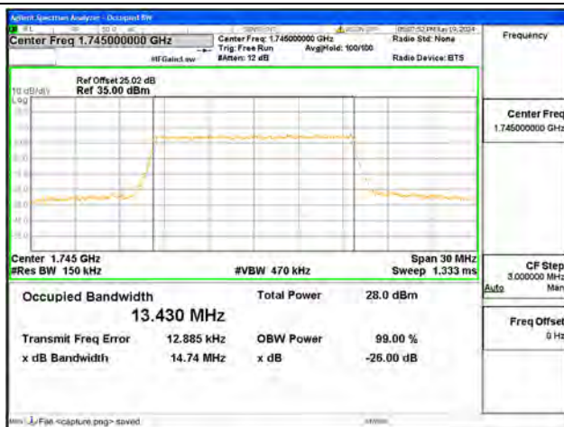
B66 / 15MHz / 16QAM/ Mid CH
