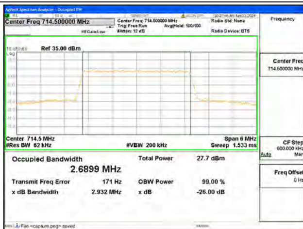
B12 / 3MHz / 16QAM/ High CH
