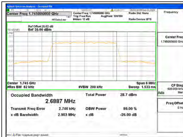
B66 / 3MHz / QPSK/ Mid CH
