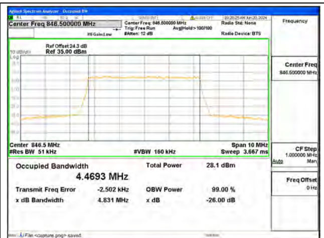
B5 / 5MHz / 16QAM/ High CH
