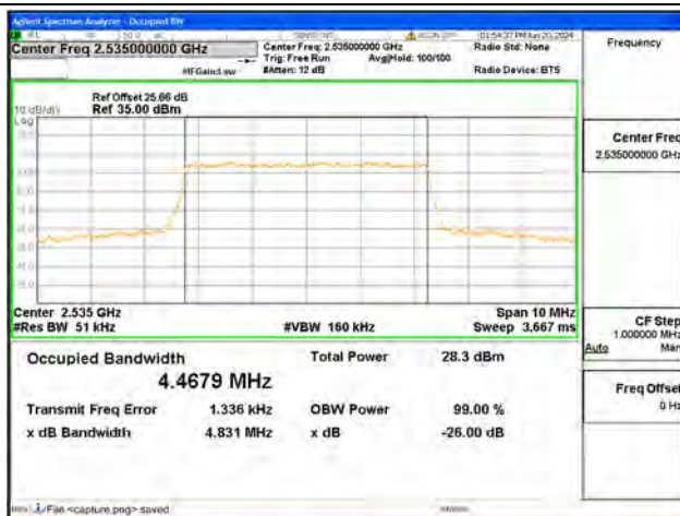
B7 / 5MHz / 16QAM/ Mid CH
