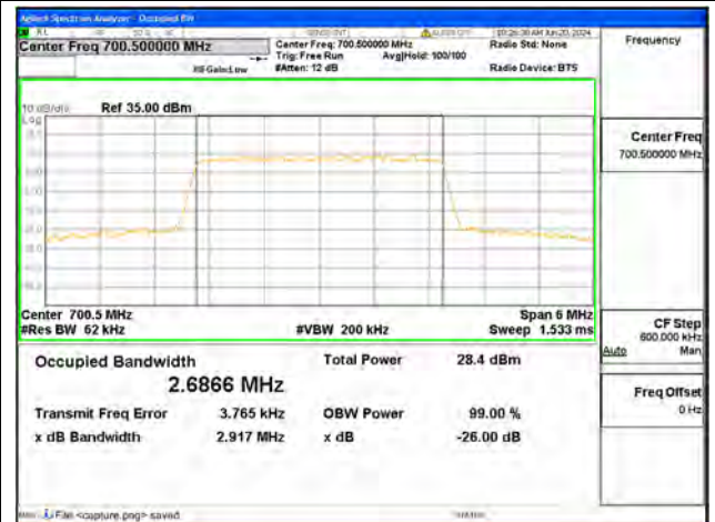
B12 / 3MHz / QPSK/ Low CH
