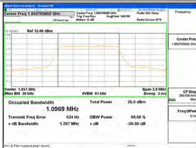
B2 / 1.4MHz / 64QAM/ Low CH
