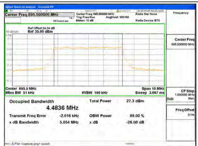
B71 / 5MHz / 16QAM/ High CH
