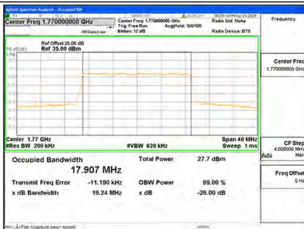
B66 / 20MHz / 16QAM/ High CH
