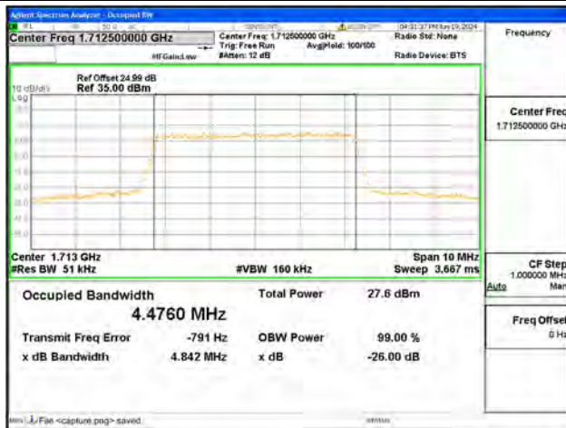
B4 / 5MHz / 64QAM/ Low CH
