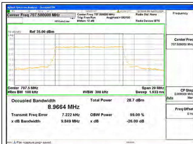
B12 / 10MHz / QPSK/ Mid CH
