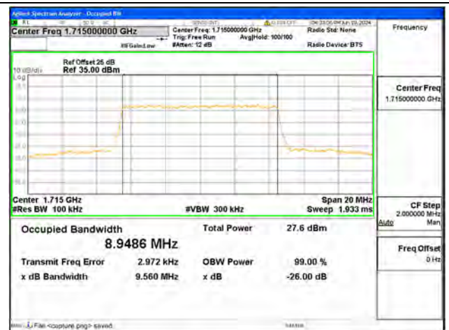
B4 / 10MHz / 64QAM/ Low CH
