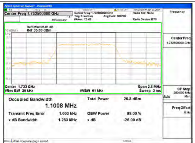
B4 / 1.4MHz / 64QAM/ Mid CH
