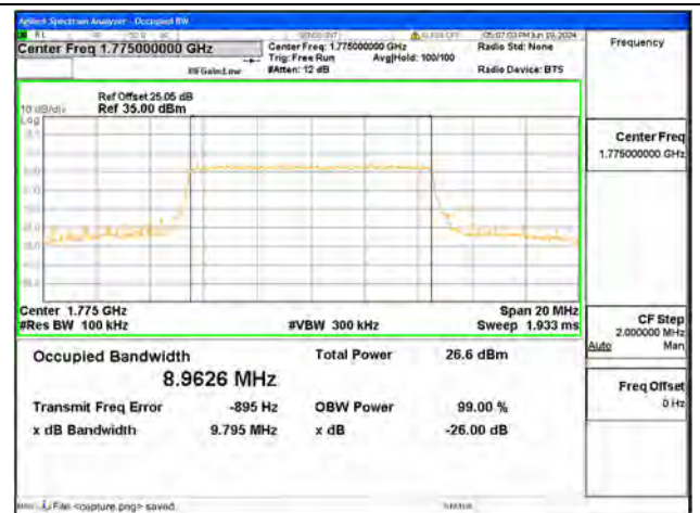
B66 / 10MHz / 64QAM/ High CH
