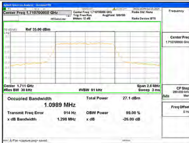
B66 / 1.4MHz / 64QAM/ Low CH
