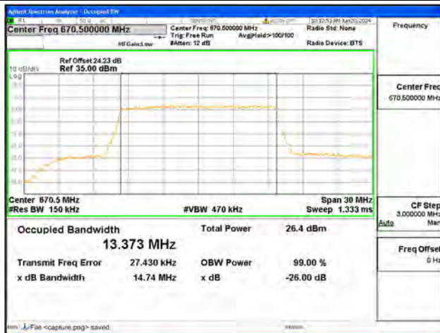
B71 / 15MHz / 64QAM/ Low CH
