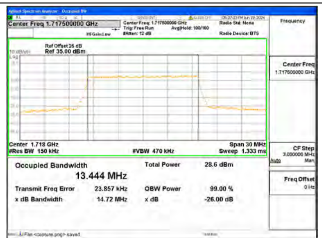
B66 / 15MHz / 16QAM/ Low CH
