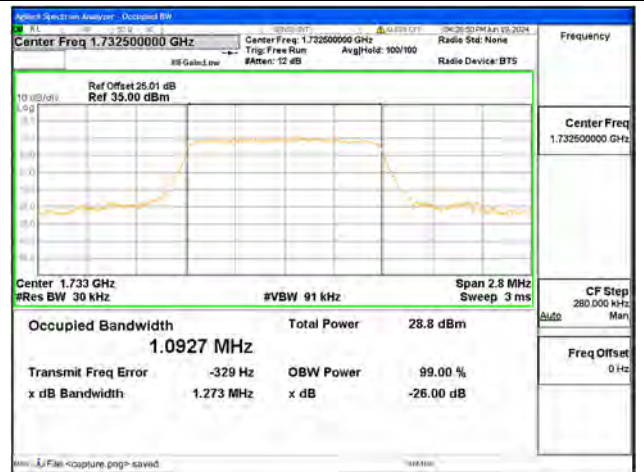
B4 / 1.4MHz / QPSK/ Mid CH
