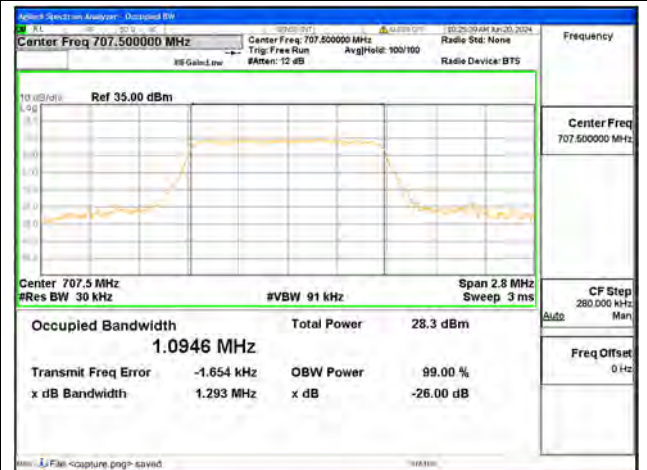
B12 / 1.4MHz / QPSK/ Mid CH
