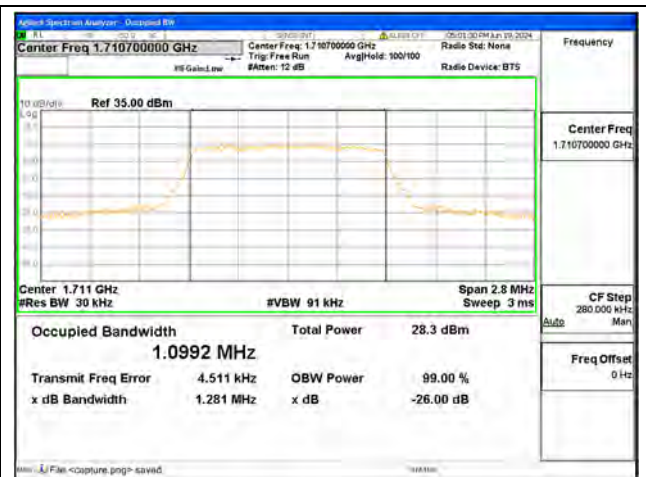
B66 / 1.4MHz / 16QAM/ Low CH
