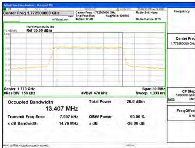
B66 / 15MHz / 64QAM/ High CH
