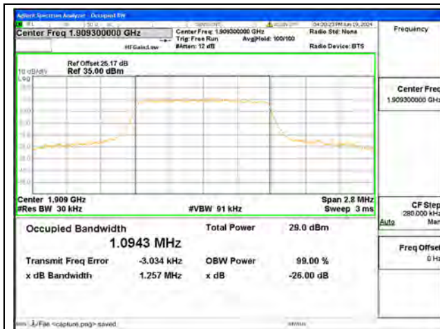
B2 / 1.4MHz / QPSK/ High CH
