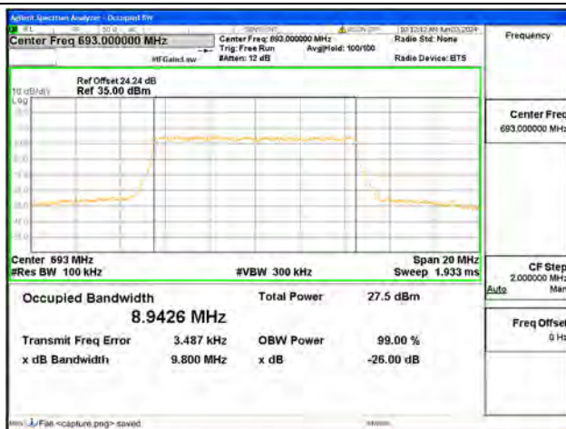
B71 / 10MHz / 16QAM/ High CH
