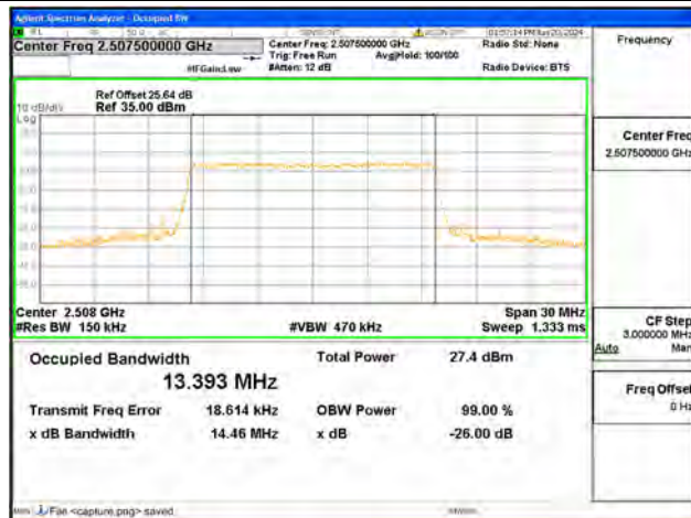
B7 / 15MHz / 64QAM/ Low CH
