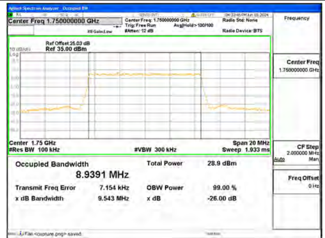
B4 / 10MHz / QPSK/ High CH
