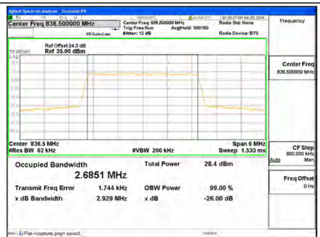
B5 / 3MHz / 16QAM/ Mid CH
