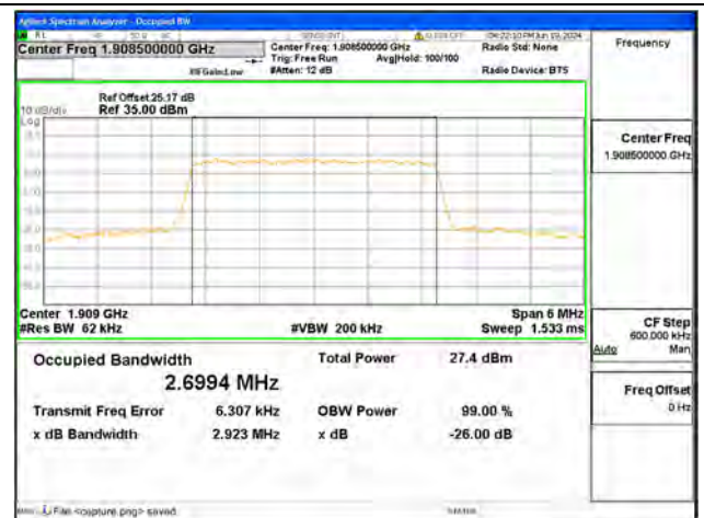
B2 / 3MHz / 64QAM/ High CH
