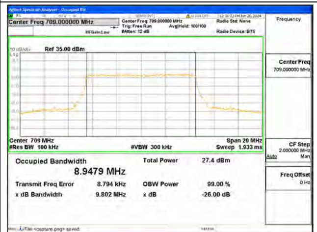
B17 / 10MHz / 64QAM/ Low CH
