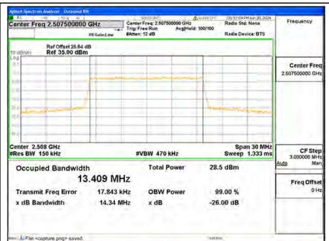
B7 / 15MHz / 16QAM/ Low CH
