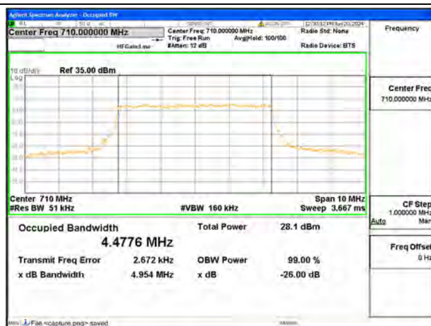
B17 / 5MHz / 16QAM/ Mid CH
