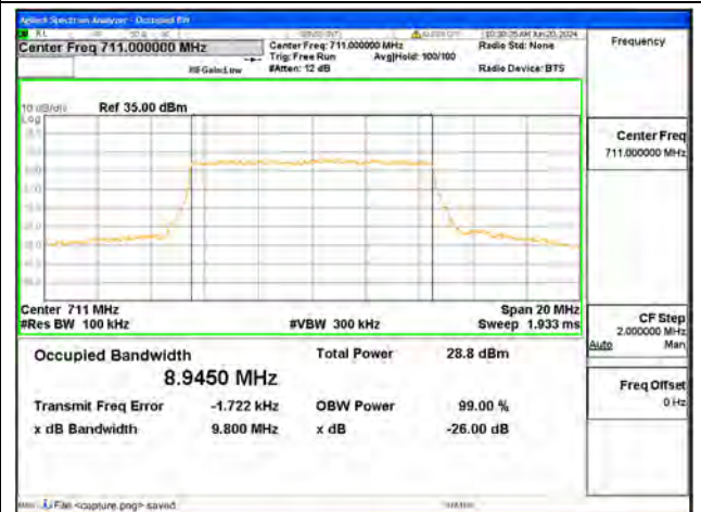
B12 / 10MHz / QPSK/ High CH
