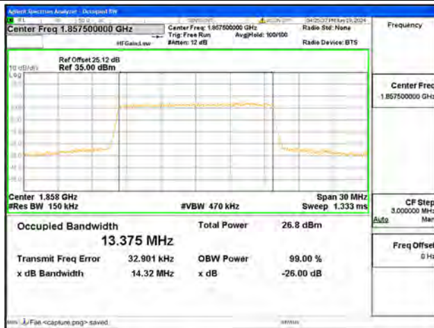
B2 / 15MHz / 64QAM/ Low CH
