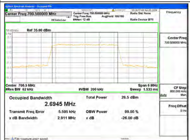
B12 / 3MHz / 64QAM/ Low CH
