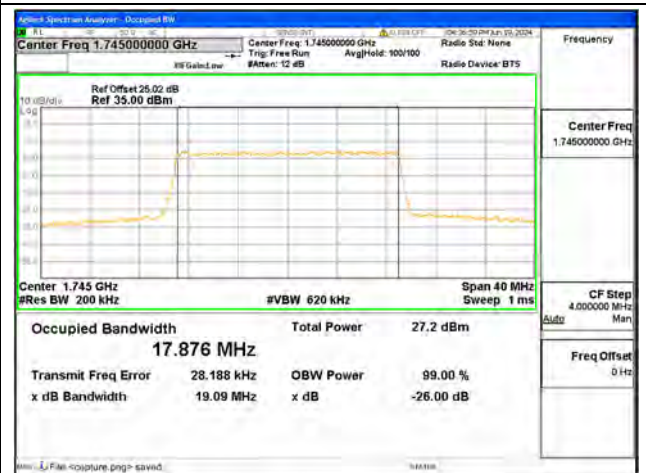
B4 / 20MHz / 64QAM/ High CH
