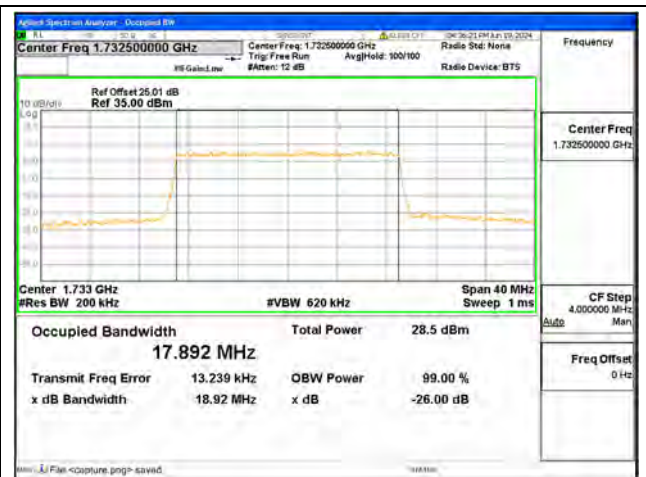
B4 / 20MHz / 16QAM/ Mid CH
