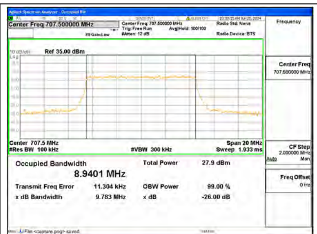
B12 / 10MHz / 16QAM/ Mid CH
