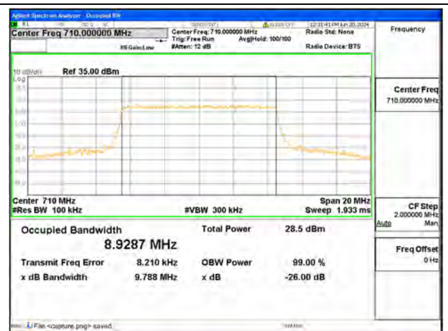
B17 / 10MHz / 16QAM/ Mid CH
