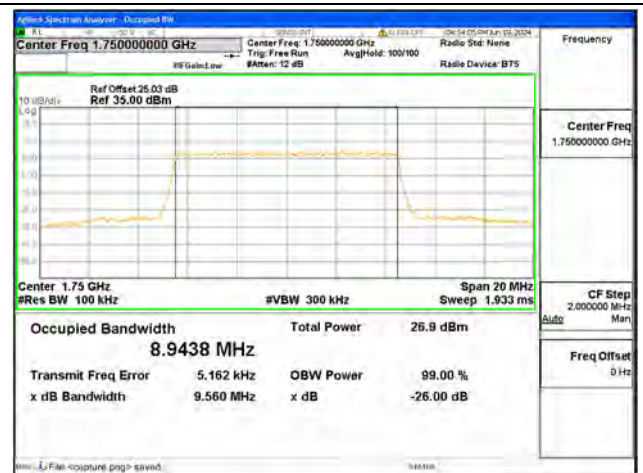
B4 / 10MHz / 64QAM/ High CH
