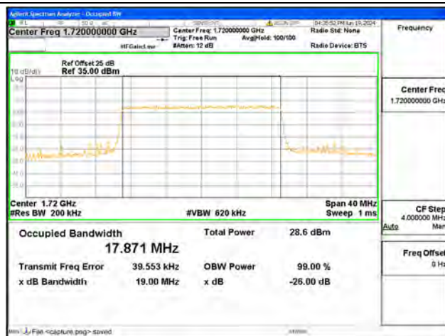
B4 / 20MHz / 16QAM/ Low CH
