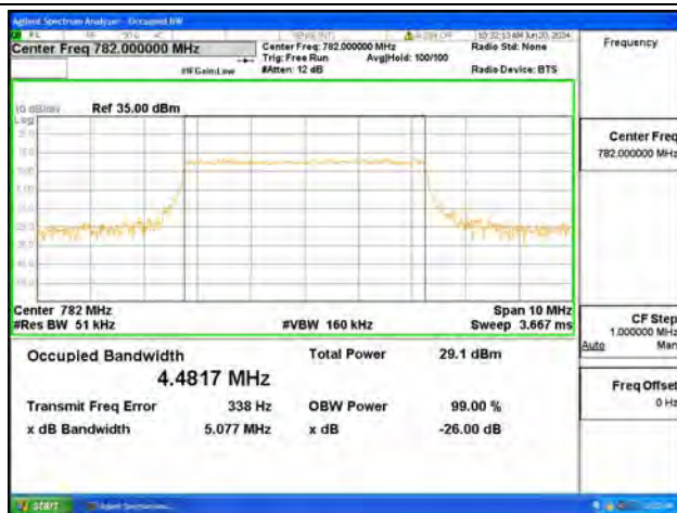
B13 / 5MHz / 16QAM/ Mid CH
