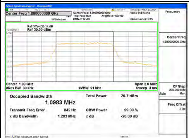
B2 / 1.4MHz / 64QAM/ Mid CH
