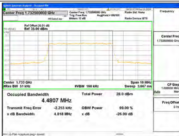
B4 / 5MHz / 16QAM/ Mid CH
