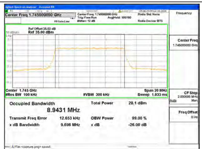
B66 / 10MHz / 16QAM/ Mid CH
