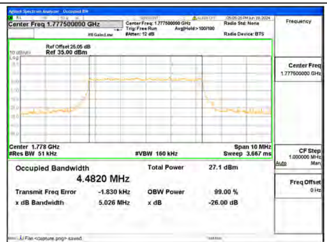
B66 / 5MHz / 16QAM/ High CH
