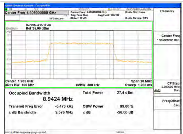
B2 / 10MHz / 64QAM/ High CH
