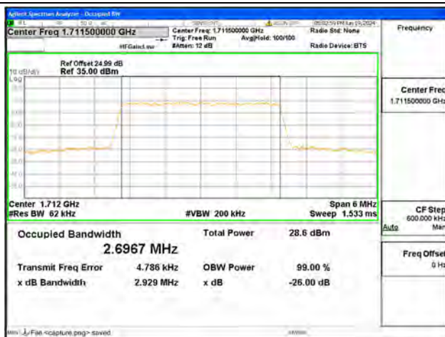
B66 / 3MHz / 16QAM/ Low CH
