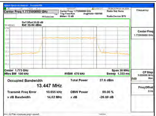
B66 / 15MHz / 16QAM/ High CH
