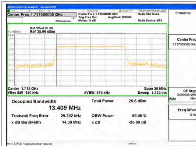
B4 / 15MHz / QPSK/ Low CH
