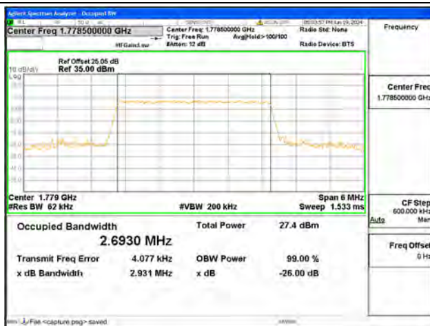
B66 / 3MHz / 16QAM/ High CH
