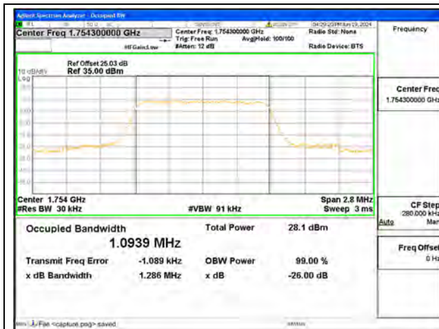
B4 / 1.4MHz / QPSK/ High CH
