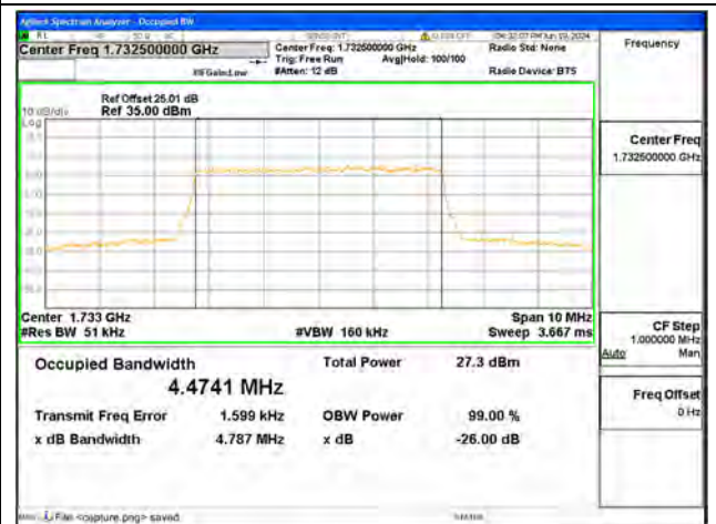
B4 / 5MHz / 64QAM/ Mid CH
