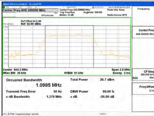
B5 / 1.4MHz / 64QAM/ High CH
