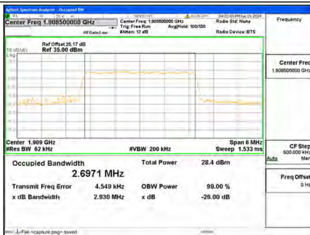
B2 / 3MHz / 16QAM/ High CH
