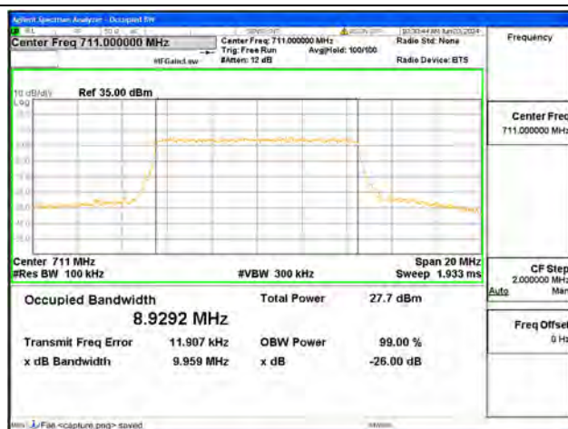
B12 / 10MHz / 16QAM/ High CH
