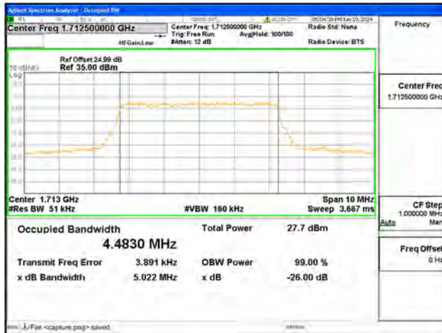
B66 / 5MHz / 64QAM/ Low CH
