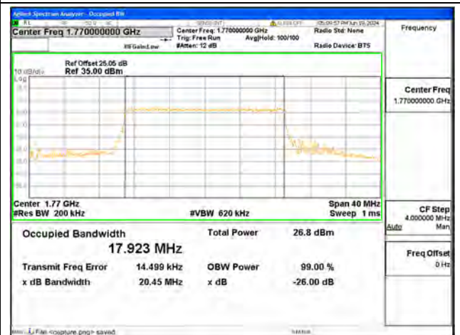
B66 / 20MHz / 64QAM/ High CH
