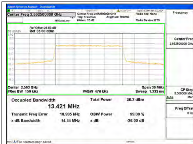
B7 / 15MHz / QPSK/ High CH
