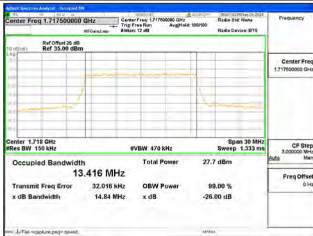
B66 / 15MHz / 64QAM/ Low CH
