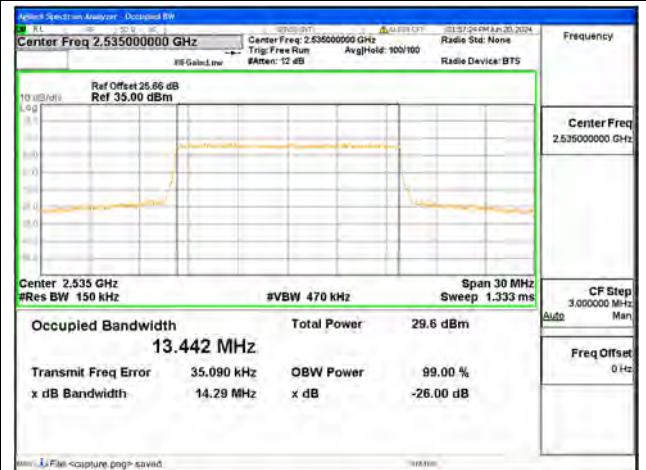
B7 / 15MHz / QPSK/ Mid CH
