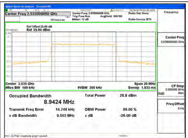
B7 / 10MHz / 16QAM/ Mid CH
