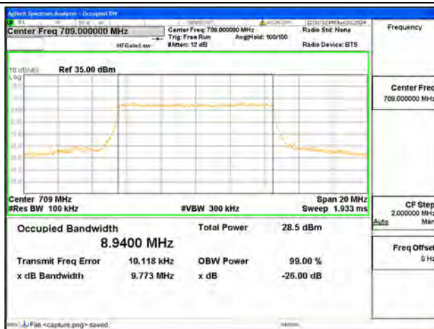
B17 / 10MHz / 16QAM/ Low CH
