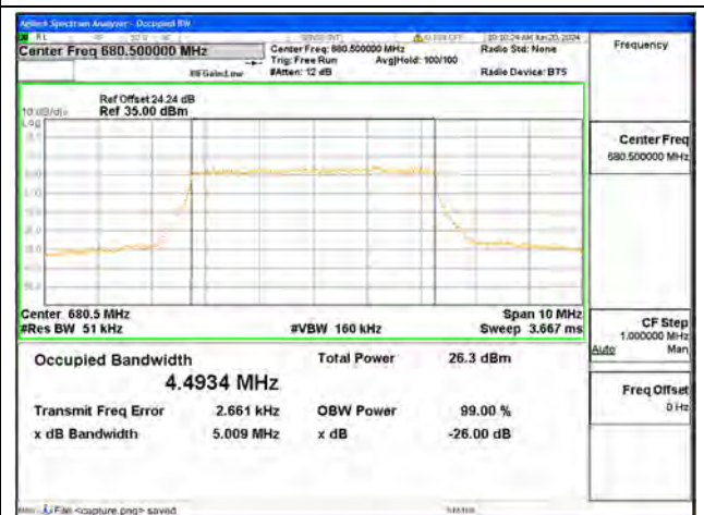
B71 / 5MHz / 64QAM/ Mid CH
