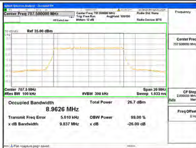
B12 / 10MHz / 64QAM/ Mid CH
