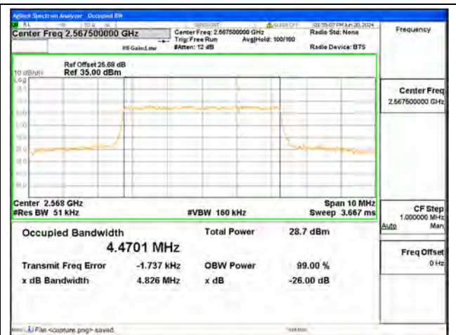
B7 / 5MHz / 16QAM/ High CH
