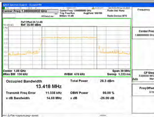
B2 / 15MHz / 16QAM/ Mid CH
