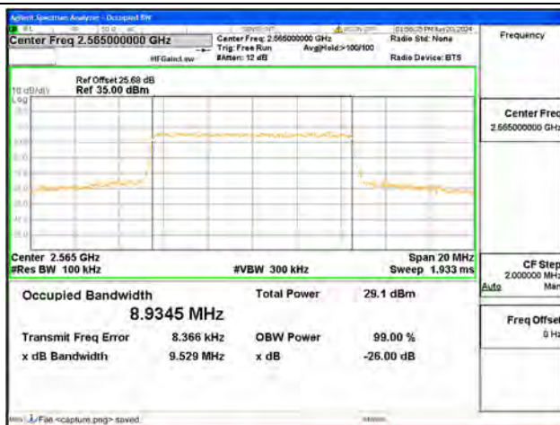
B7 / 10MHz / 16QAM/ High CH
