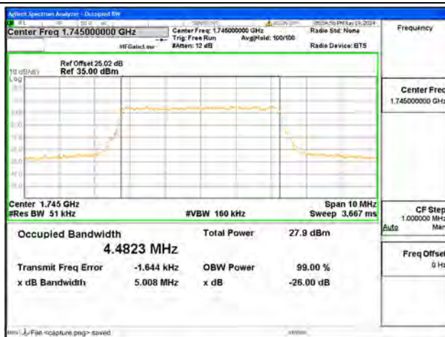
B66 / 5MHz / 16QAM/ Mid CH
