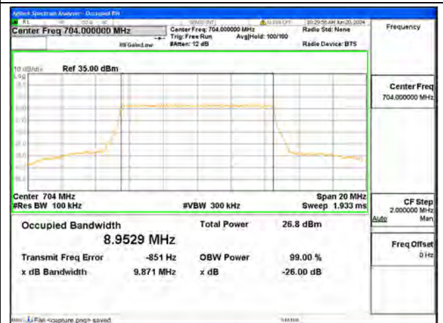
B12 / 10MHz / 64QAM/ Low CH
