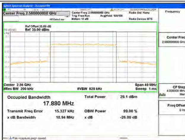
B7 / 20MHz / 16QAM/ High CH
