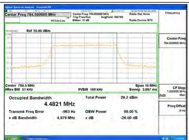
B13 / 5MHz / 16QAM/ High CH
