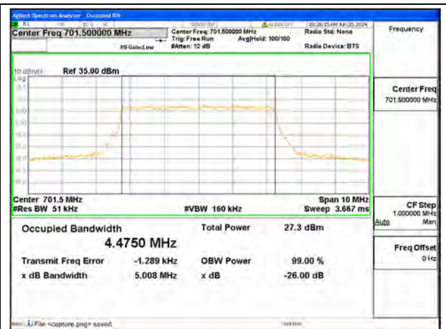
B12 / 5MHz / 16QAM/ Low CH
