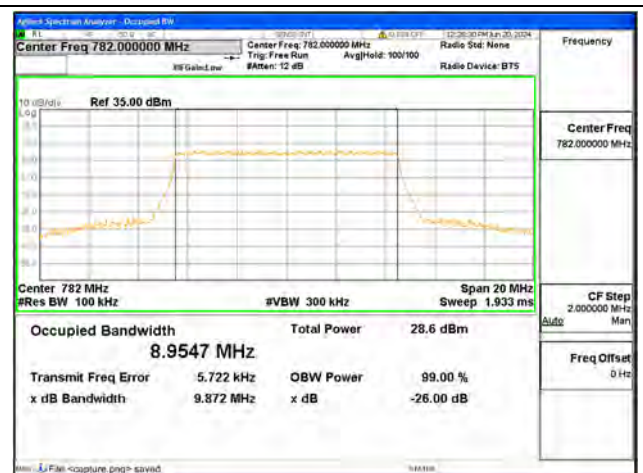
B13 / 10MHz / 64QAM/ Mid CH
