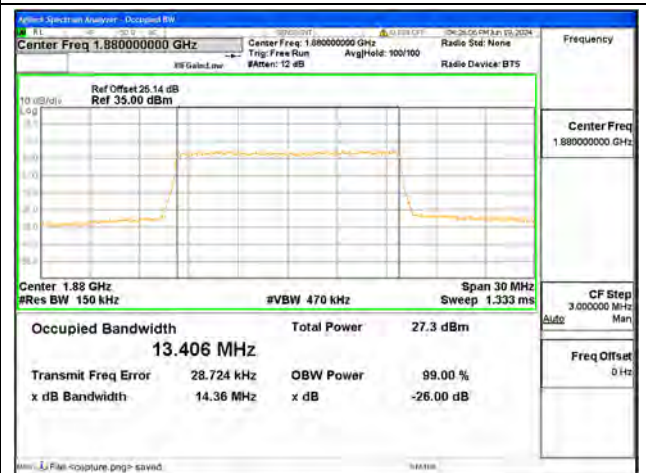
B2 / 15MHz / 64QAM/ Mid CH
