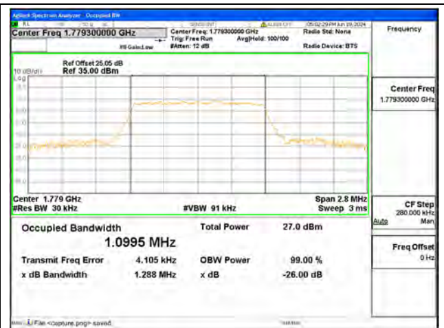
B66 / 1.4MHz / 16QAM/ High CH
