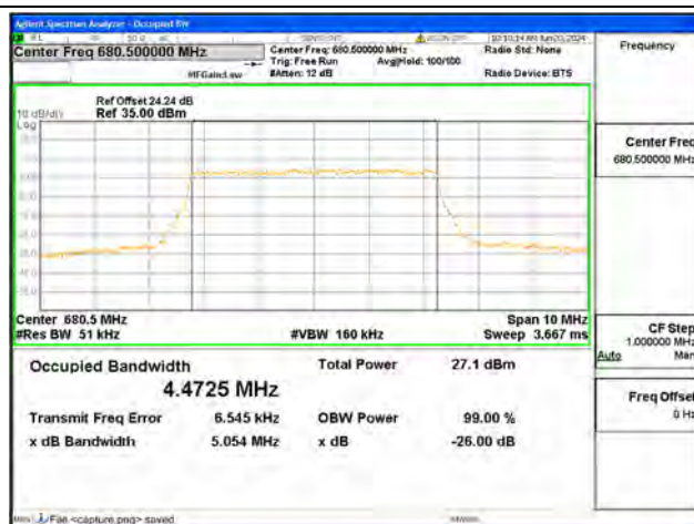
B71 / 5MHz / 16QAM/ Mid CH
