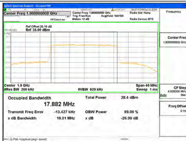
B2 / 20MHz / 16QAM/ High CH
