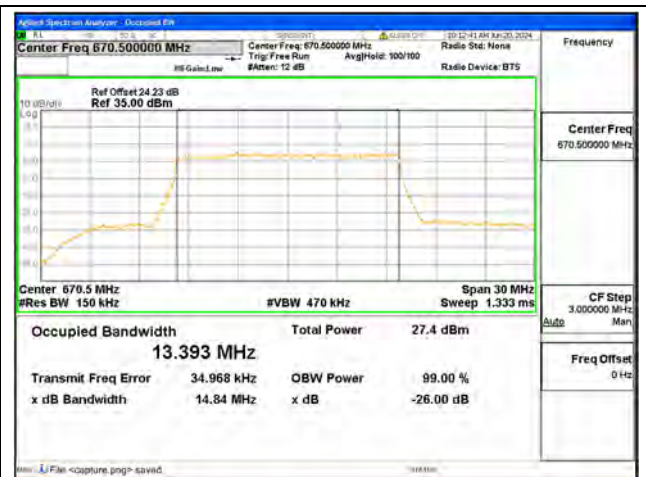
B71 / 15MHz / 16QAM/ Low CH
