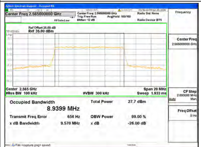
B7 / 10MHz / 64QAM/ High CH
