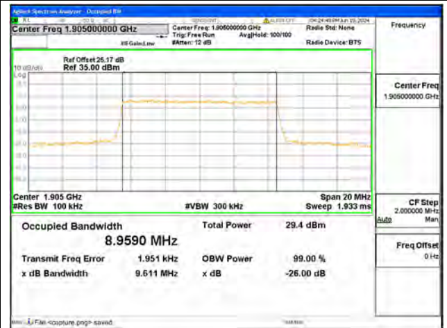
B2 / 10MHz / QPSK/ High CH
