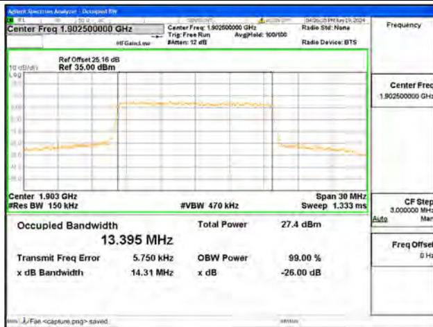
B2 / 15MHz / 64QAM/ High CH
