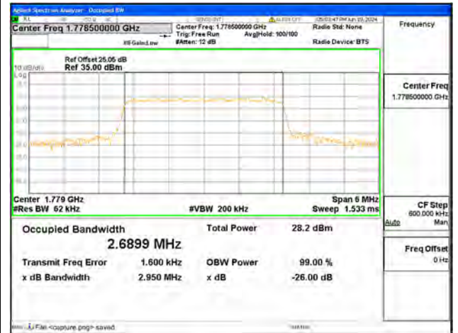
B66 / 3MHz / QPSK/ High CH
