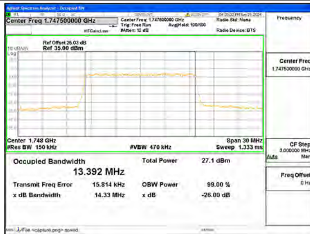
B4 / 15MHz / 64QAM/ High CH
