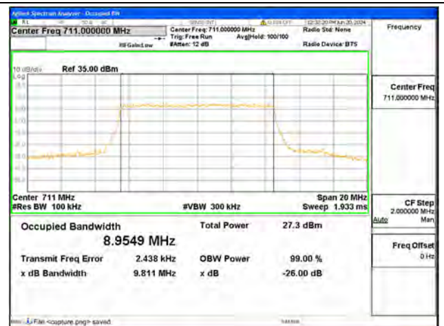
B17 / 10MHz / 64QAM/ High CH
