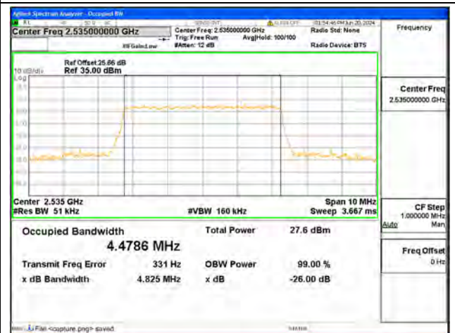
B7 / 5MHz / 64QAM/ Mid CH
