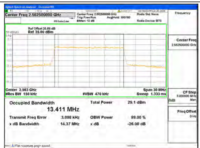
B7 / 15MHz / 16QAM/ High CH
