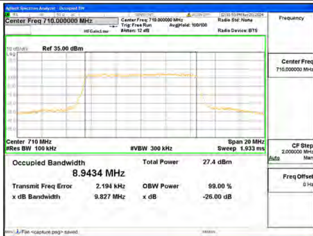
B17 / 10MHz / 64QAM/ Mid CH
