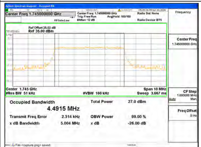
B66 / 5MHz / 64QAM/ Mid CH
