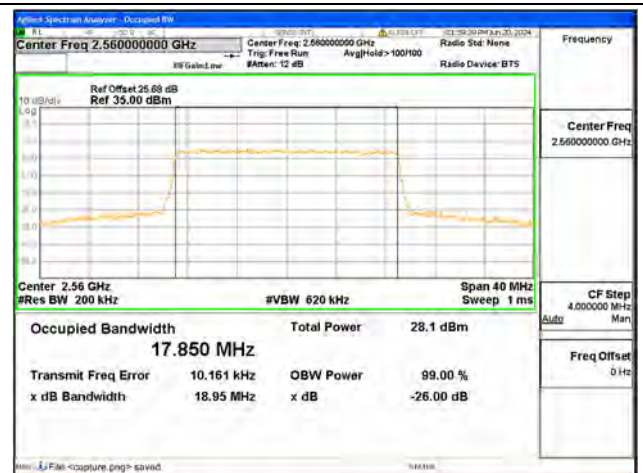
B7 / 20MHz / 64QAM/ High CH
