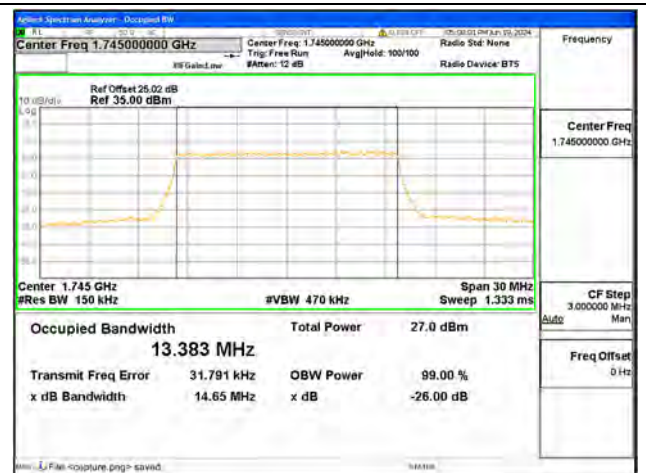
B66 / 15MHz / 64QAM/ Mid CH
