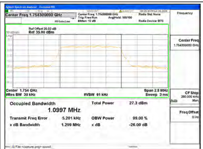
B4 / 1.4MHz / 16QAM/ High CH
