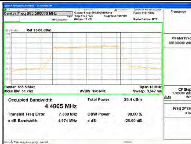
B71 / 5MHz / 64QAM/ Low CH
