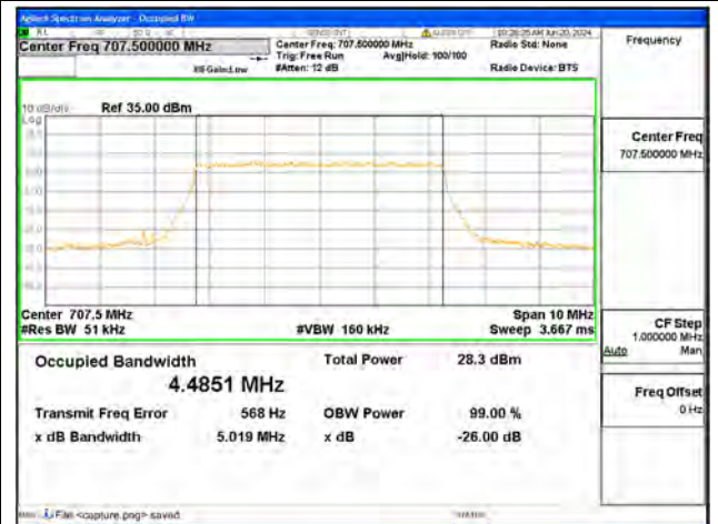
B12 / 5MHz / QPSK/ Mid CH
