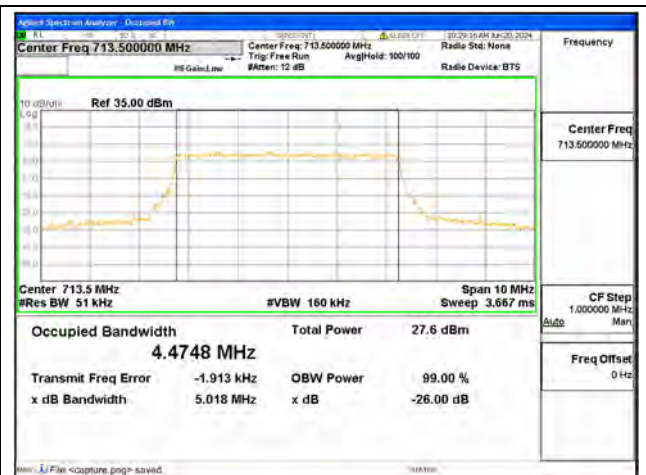
B12 / 5MHz / 16QAM/ High CH
