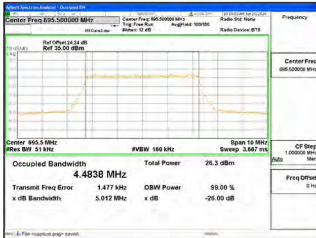
B71 / 5MHz / 64QAM/ High CH
