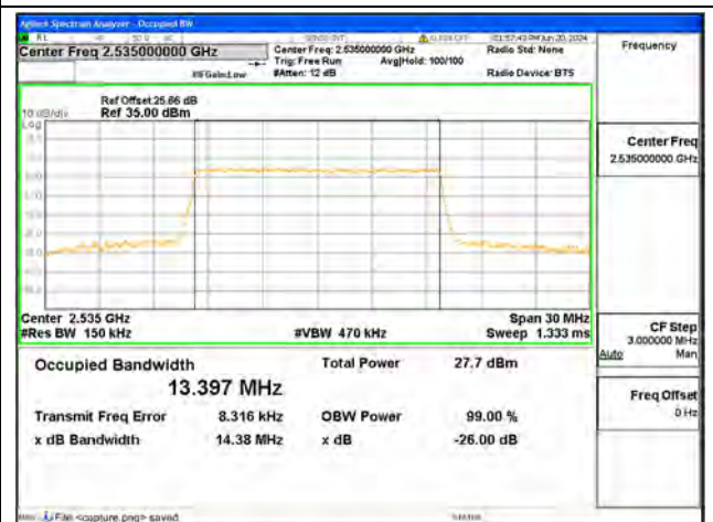
B7 / 15MHz / 64QAM/ Mid CH
