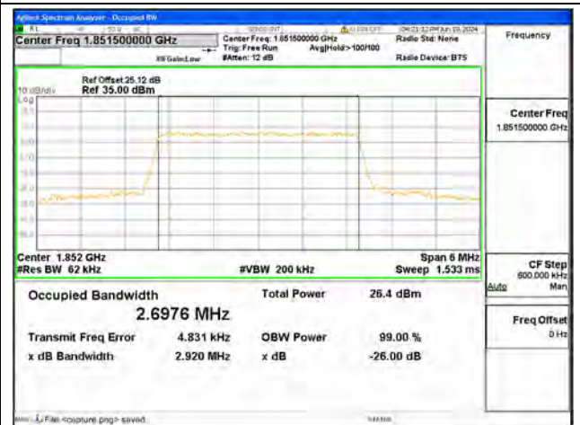
B2 / 3MHz / 64QAM/ Low CH
