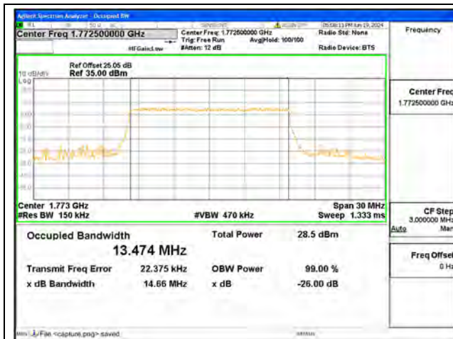
B66 / 15MHz / QPSK/ High CH
