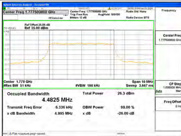
B66 / 5MHz / 64QAM/ High CH
