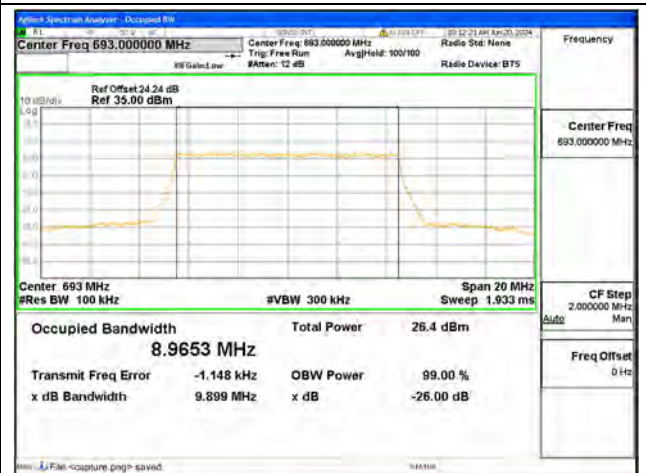
B71 / 10MHz / 64QAM/ High CH
