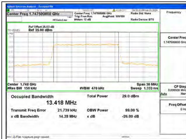
B4 / 15MHz / QPSK/ High CH
