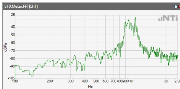
ANSI/TIA 5050-2018 \ 8N HAC OFF \ NB 12.2kbps\ 5.2 Receive path – distortion and noise\WLAN 5.3GHz
