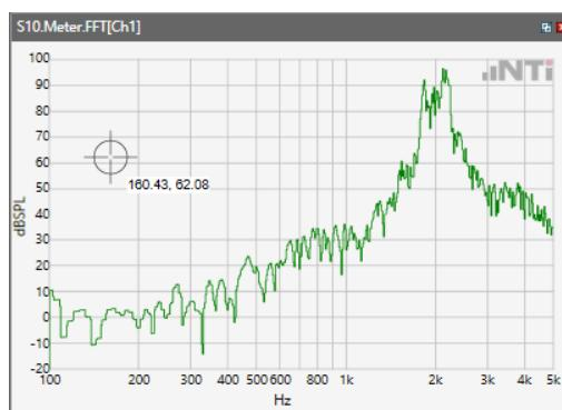
ANSI/TIA 5050-2018 \ 8N HAC OFF \ WB 23.85 kbps\ 5.2 Receive path – distortion and noise\LTE Band 66
