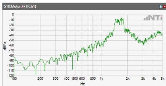
ANSI/TIA 5050-2018 \ 8N HAC OFF \ WB 23.85 kbps\ 5.2 Receive path – distortion and noise\WLAN 5.2GHz
