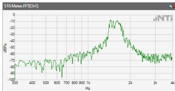
ANSI/TIA 5050-2018 \ 8N HAC OFF \ NB 12.2kbps\ 5.2 Receive path – distortion and noise\WLAN 5.8GHz
