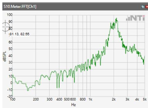
ANSI/TIA 5050-2018 \ 8N HAC OFF \ WB 23.85 kbps\ 5.2 Receive path – distortion and noise\LTE Band 7
