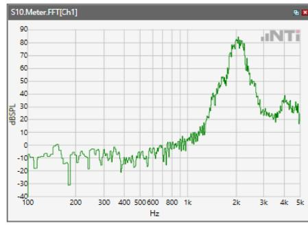
ANSI/TIA 5050-2018 \ 8N HAC OFF \ NB 12.2kbps\ 5.2 Receive path – distortion and noise\LTE Band 7
