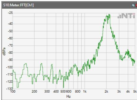
ANSI/TIA 5050-2018 \ 8N HAC OFF \ WB 23.85 kbps\ 5.2 Receive path – distortion and noise\LTE Band 5
