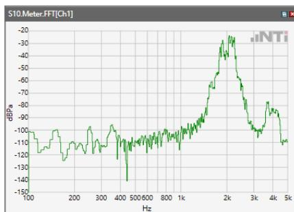
ANSI/TIA 5050-2018 \ 8N HAC OFF \ NB 12.2kbps\ 5.2 Receive path – distortion and noise\GSM 1900
