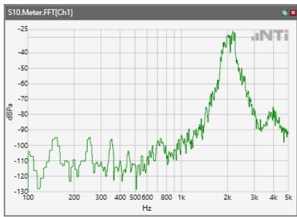
ANSI/TIA 5050-2018 \ 8N HAC OFF \ WB 23.85 kbps\ 5.2 Receive path – distortion and noise\WCDMA Band II
