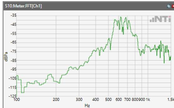
ANSI/TIA 5050-2018 \ 8N HAC OFF \ NB 12.2kbps\ 5.2 Receive path – distortion and noise\LTE Band 5
