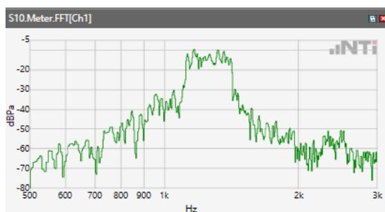
ANSI/TIA 5050-2018 \ 8N HAC OFF \ NB 12.2kbps\ 5.2 Receive path – distortion and noise\WLAN 5.8GHz
