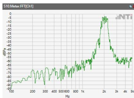
ANSI/TIA 5050-2018 \ 8N HAC OFF \ WB 23.85 kbps\ 5.2 Receive path – distortion and noise\WLAN 5.8 GHz
